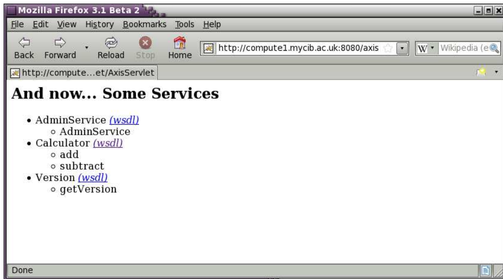
Figure 4.2: The ‘Available Services’ links leads to a web page as shown in this figure. The new Calculator service is listed along with the associated methods.
