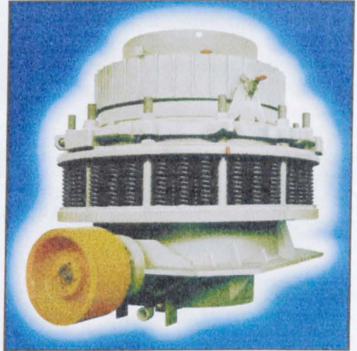
Figure 13-15 [ref 120] Tel-smith cone crusher. An advanced version of one of the Symons family of crushers. These crushers range in weight from about five to fifty tonnes.
