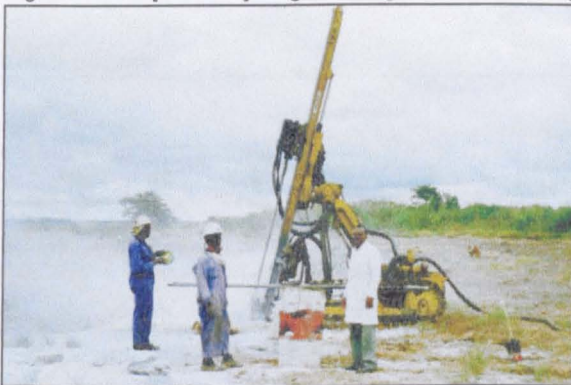
Figure 11-41 [ref Mills] Angle drilling with a drifter rig
