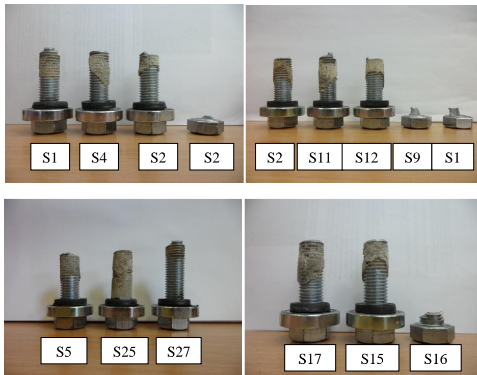
Figure 4.4 : Failure mode of Extended Hollobolt
