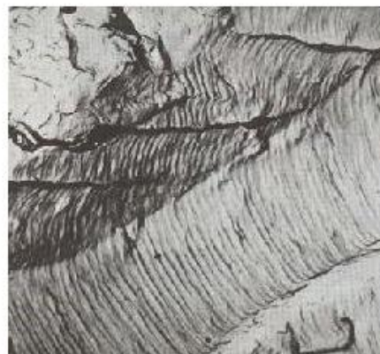
Figure 2.22 : Magnification of fatigue failure showing striations (marinediesels.co.uk)
