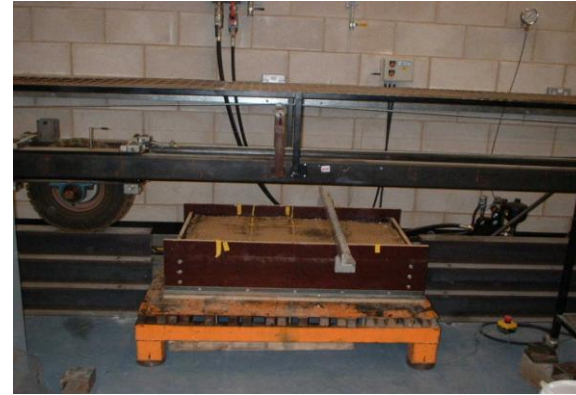
Figure 4. 5 Side view of the Nottingham Slab Testing Facility
