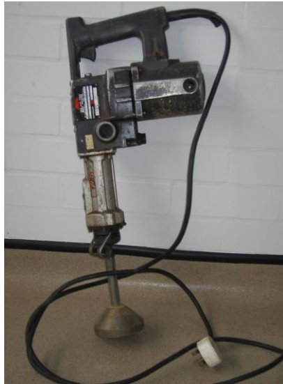
Figure 4. 9 Vibrating hammer used on soils for the SW
