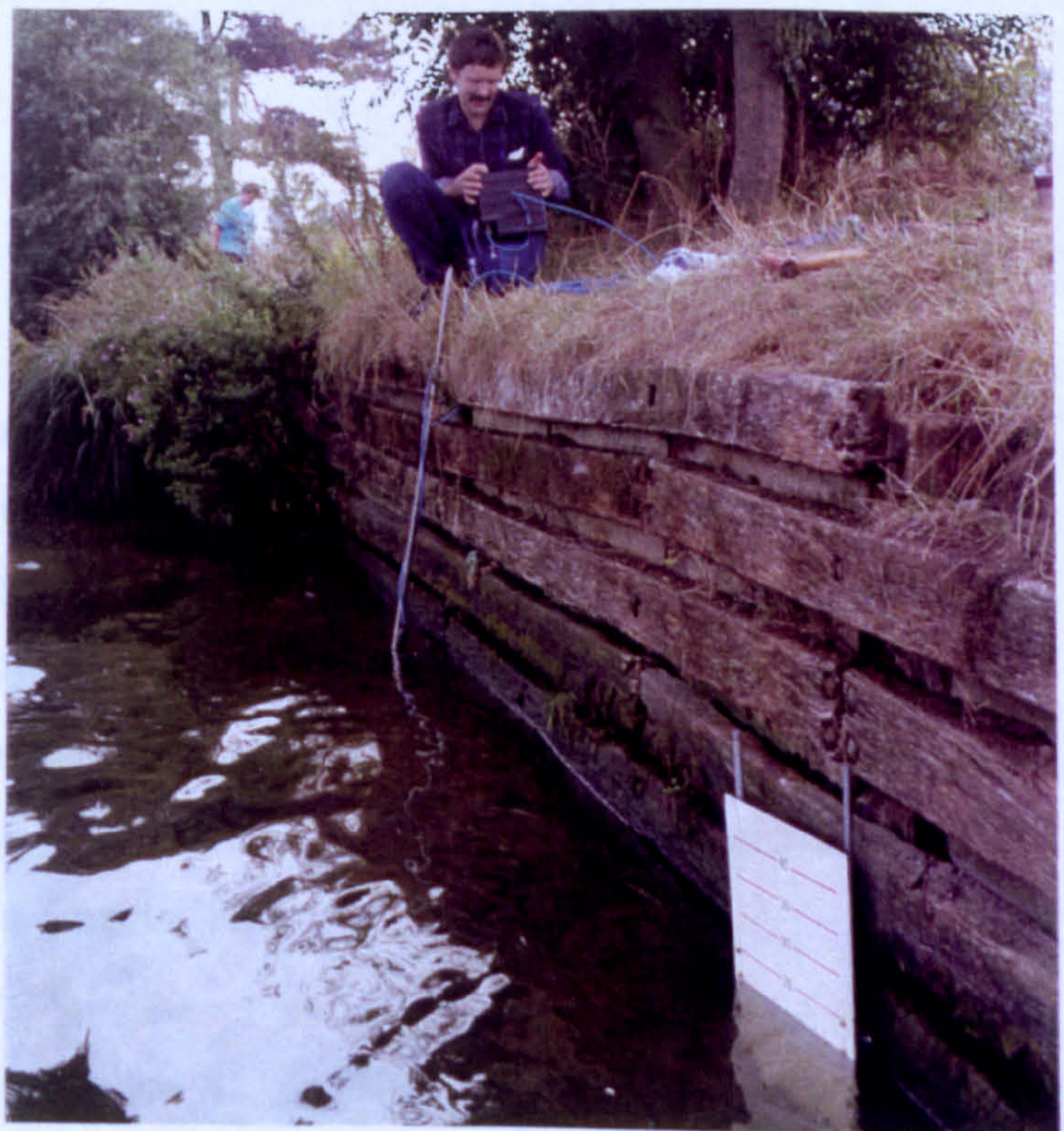
Plate 2.1 Wave board and EMF used to monitor wash characteristics.
