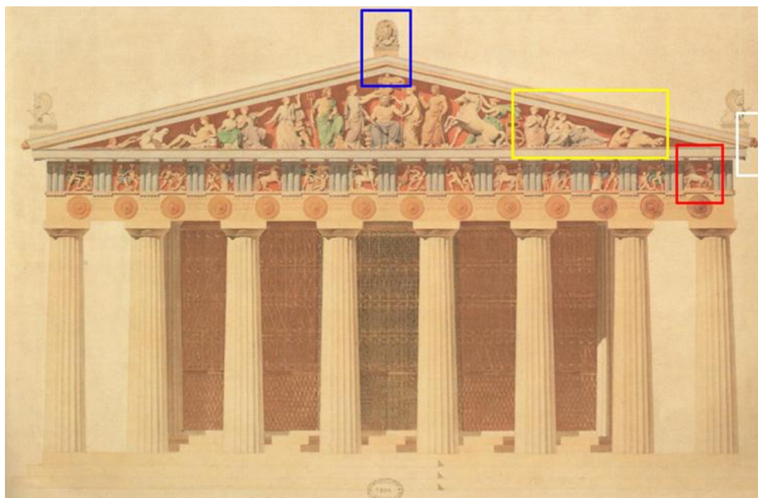
Figure 3.12 Reconstruction of the east façade of the Parthenon, which presents levels of sculptures - blue: akroteria (highest level); yellow: pediment; white: cornice - lion head; red: metope. (Source: Tournikiotis, P. The Parthenon and Its Impact in Modern Times , 1994, p. 261, edited by researcher)
