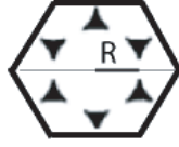
Figure 7.40: In the top transversal plane of the NSL substrates, there are 6 metallic nanostructures in a hexagonal cell. R is the radius of the inner circle, corresponding to a bead that has been removed.
