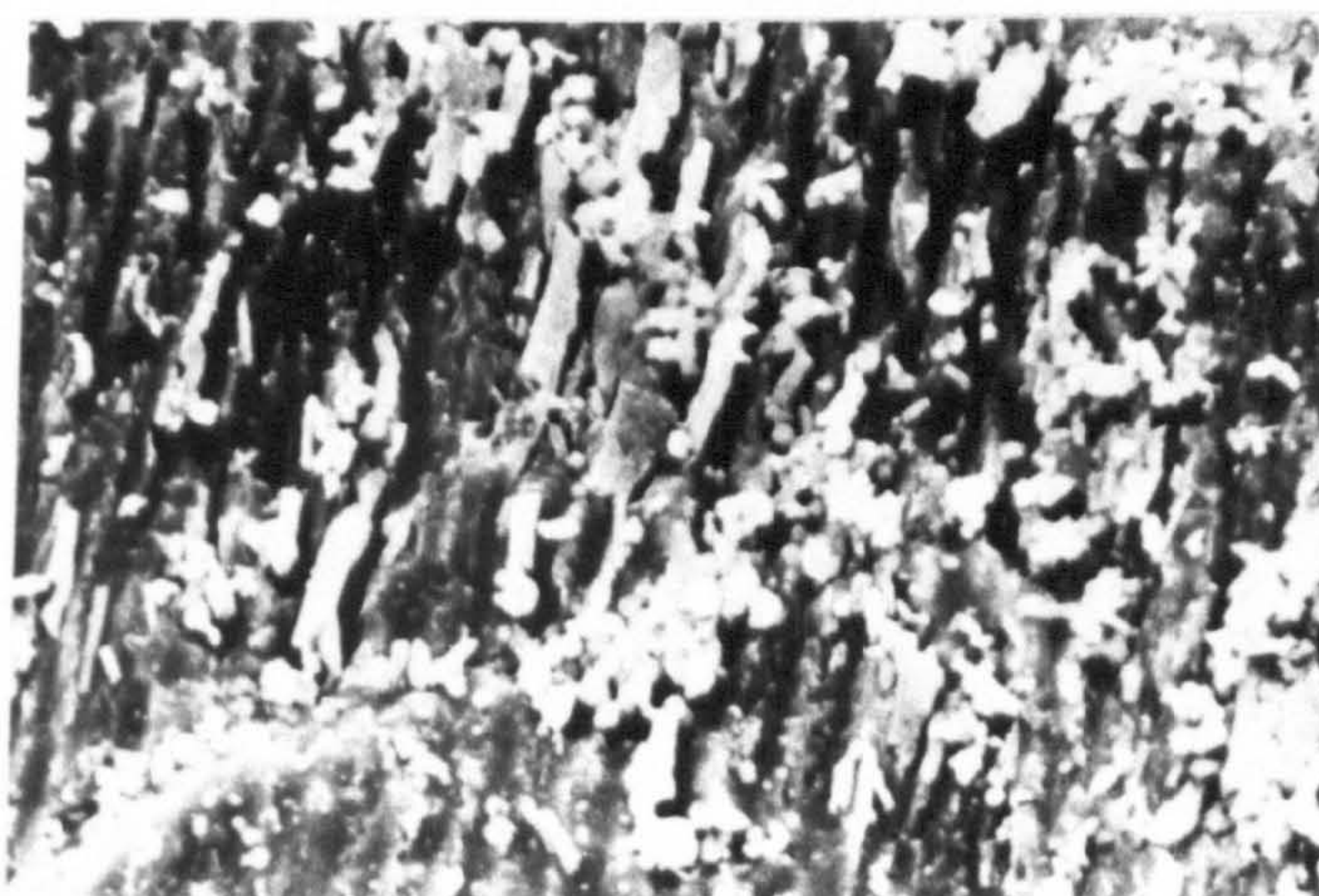
24c) Alloy 7010 (heavily peened)
