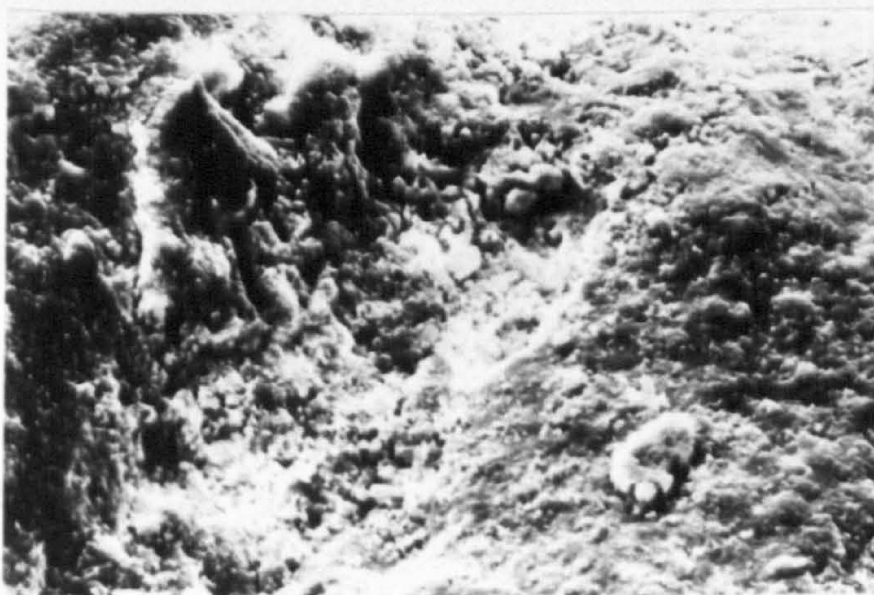
27b) Alloy 8090 (heavily peened)
