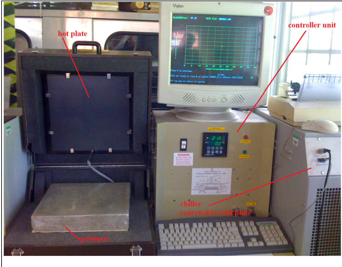
Figure 3-2 Heat flowmeter apparatus for thermal conductivity measurement
