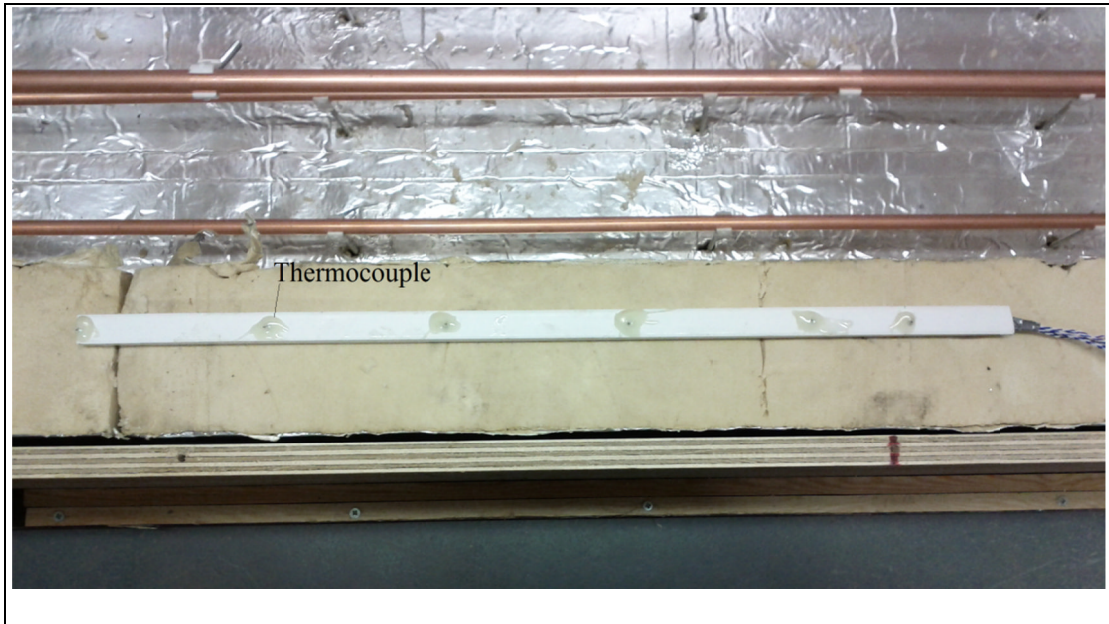
Figure 5-8 Thermocouples were fastened on a conduit
