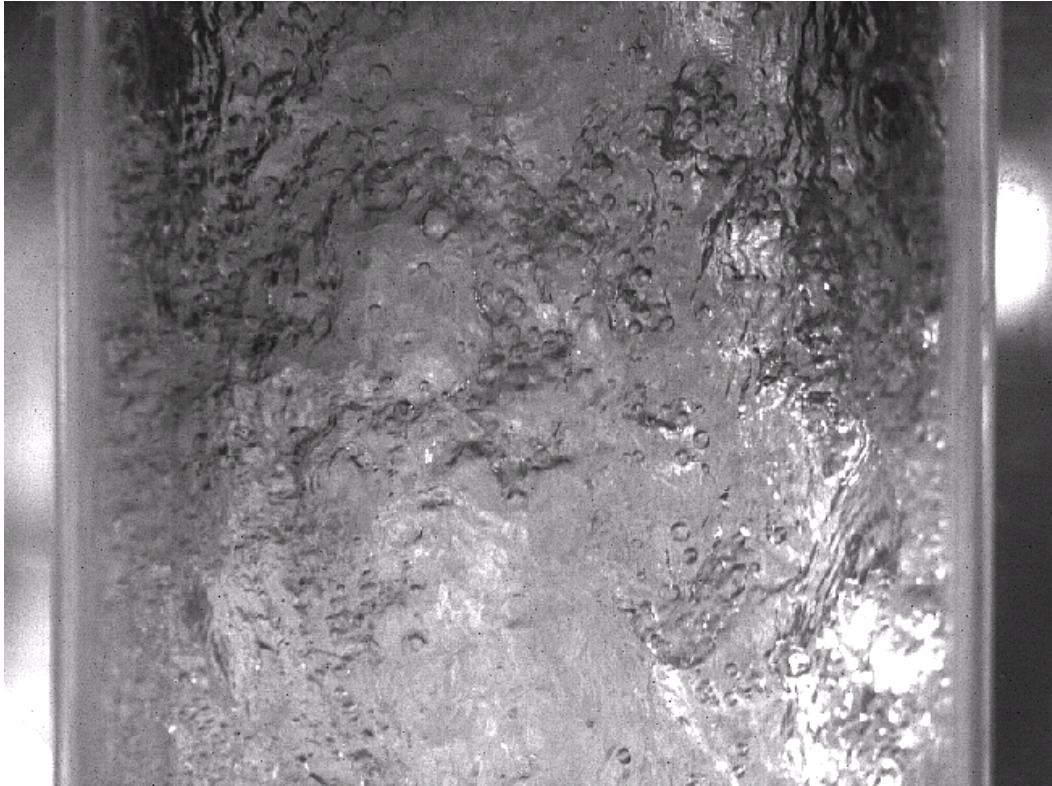
Figure 4.4 Churn-annular flow. Gas superficial velocity 10 m/s, liquid superficial velocity 0.04 m/s. Waves are very irregular, moving “sideways” on the pipe wall. Also gas bubbles in the liquid film can be observed.
