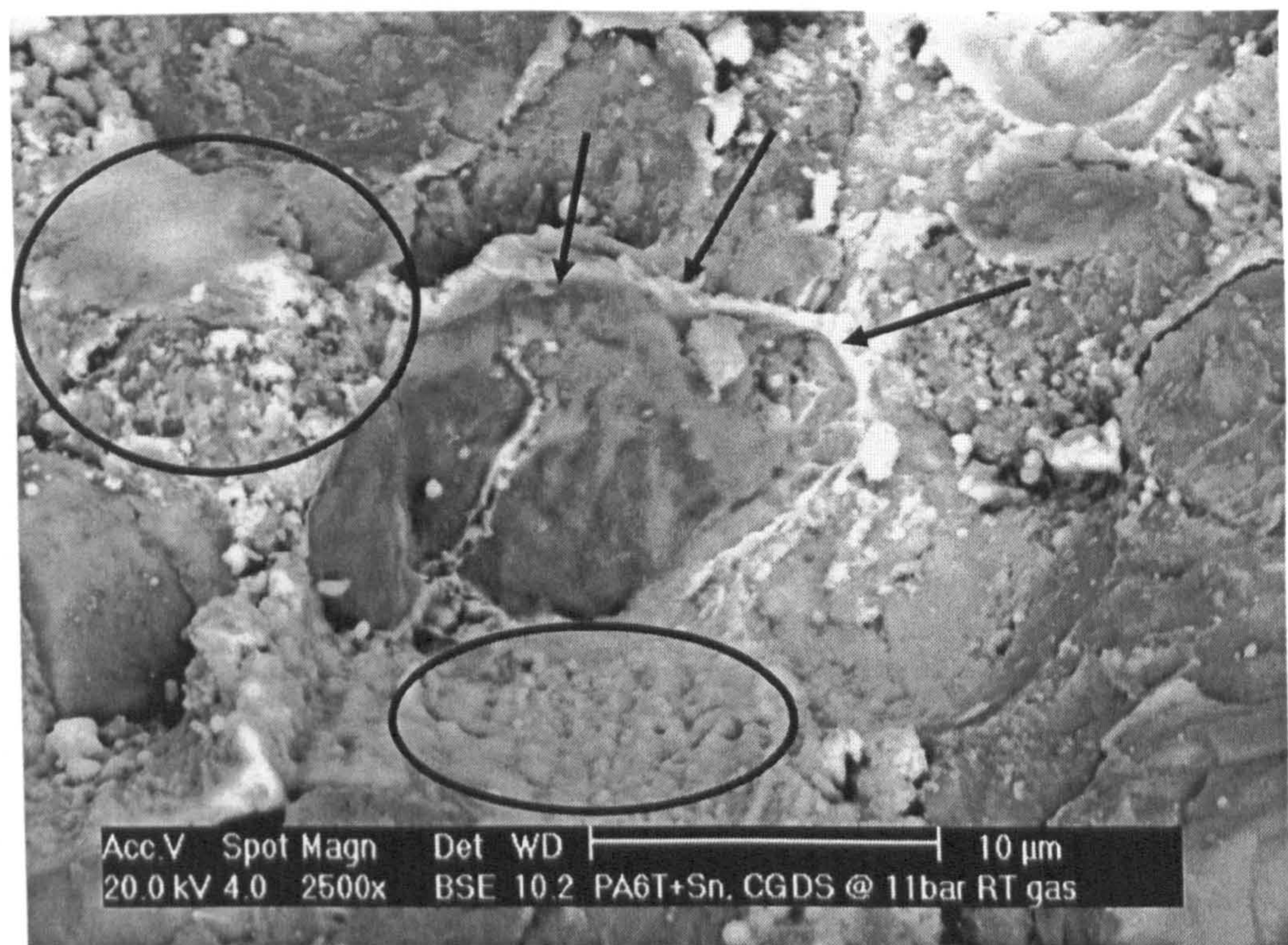
Fig. 5.33: BSE image of copper cold sprayed on PA6T + Sn at 11 bar using powder feed rate of 0.25\text{ g s}^{-1} , showing fine particles formed in tin and extensive deformation of tin (shown inside circle). Metal jetting in tin due to impact of copper is also seen (shown by arrows). Tin deposited using conditions described in Table 5.19 and traverse speed of 0.5\text{ m s}^{-1} .
