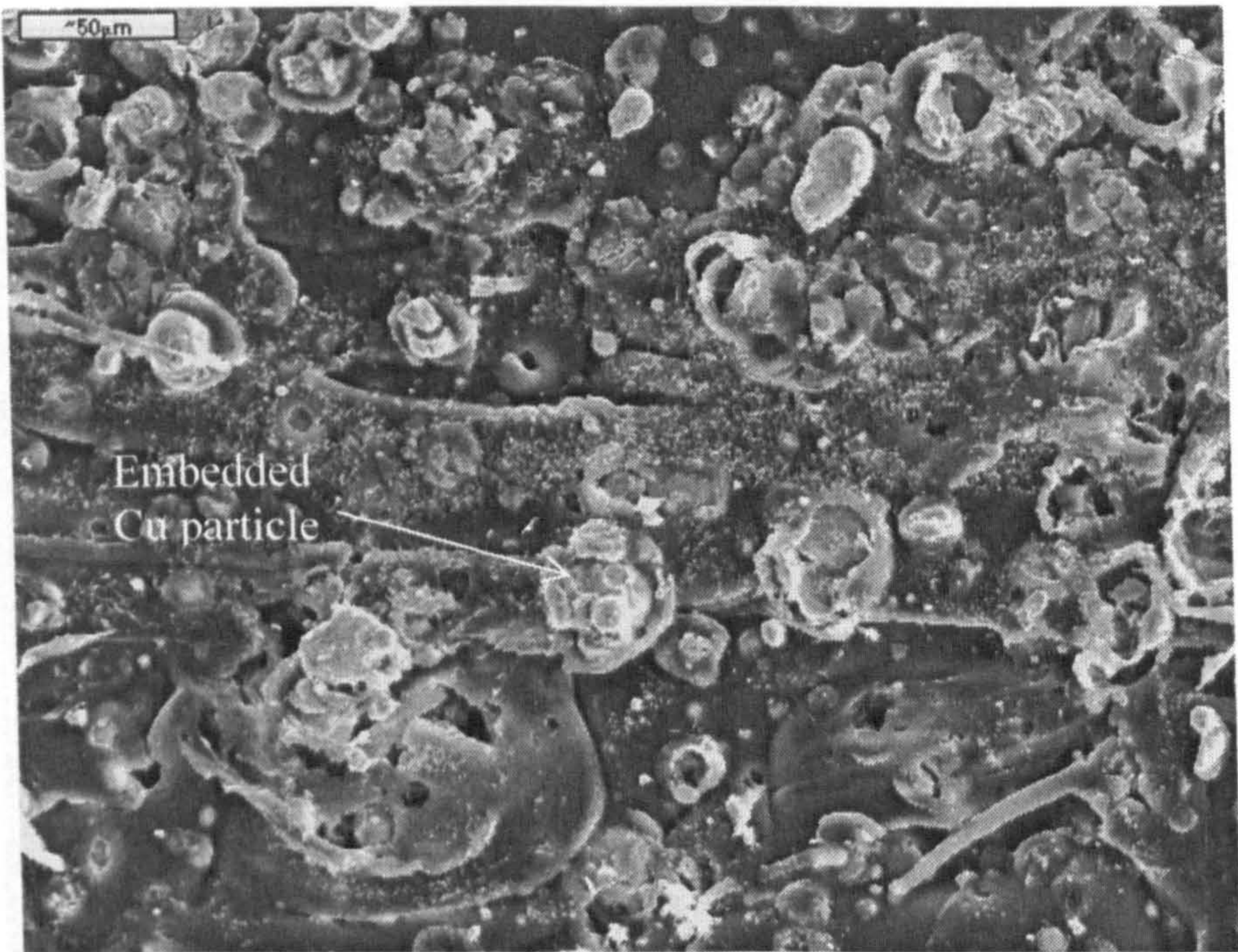
Fig. 5.24: Secondary electron image of copper cold sprayed on PA6T at 29 bar and 298 K respectively. Very few glass fibres are seen and the substrate is heavily fractured. Deposition using traverse speed of 0.5\text{ m s}^{-1} and powder feed rate of 0.25\text{ g s}^{-1} .
