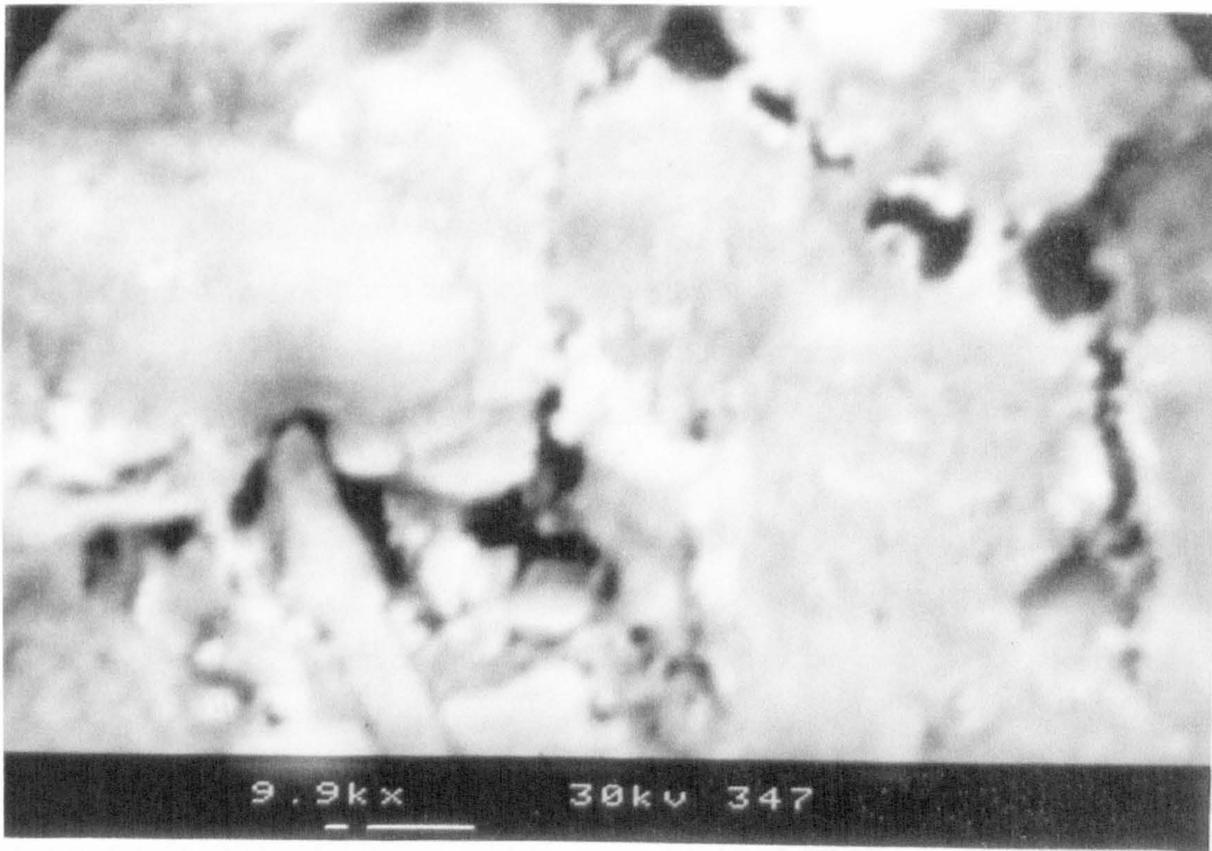
Fig 7.21 SEM of membrane cleaned with 4000ppm hydrochloric acid
