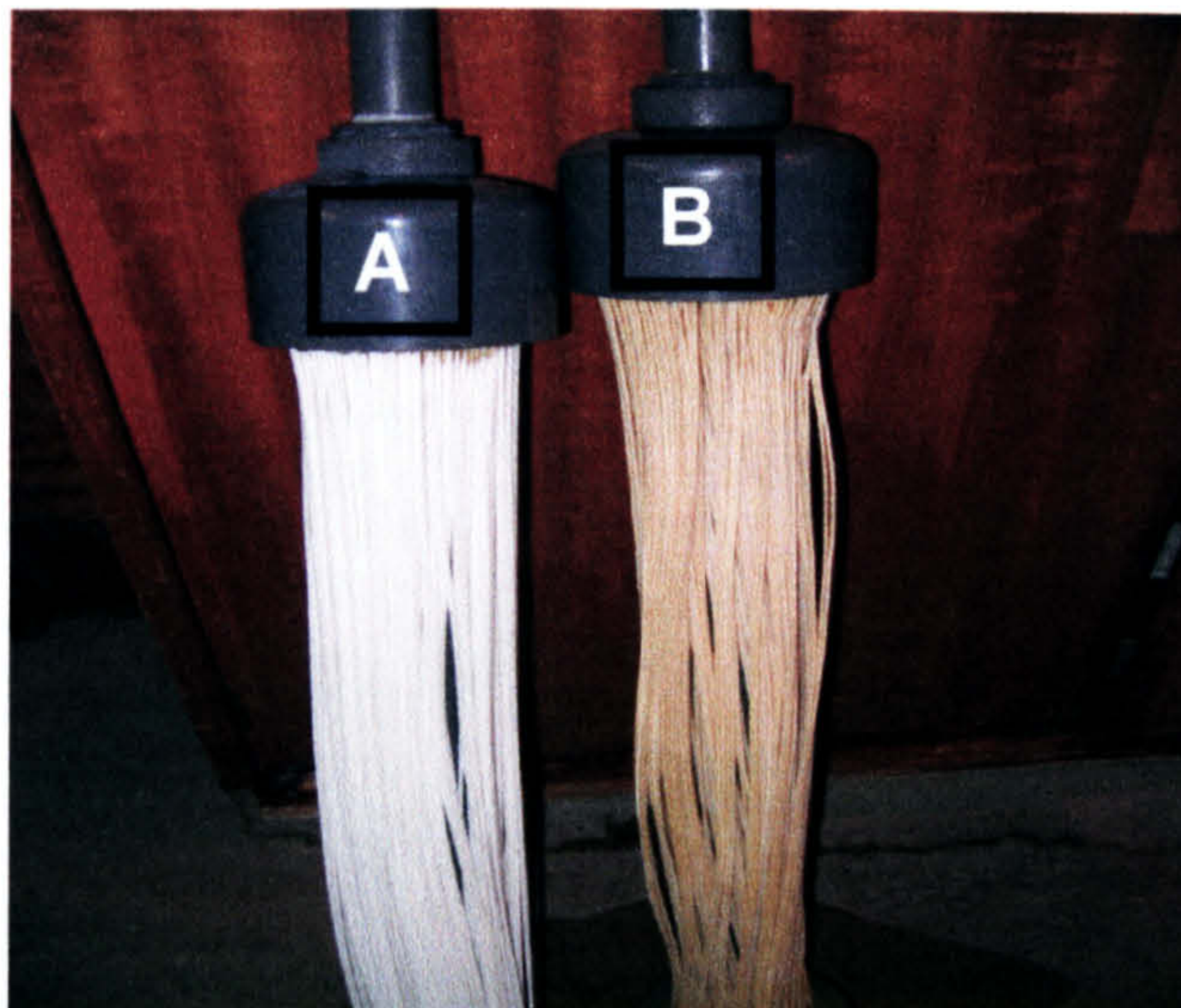
Fig 7.15 A is a clean membrane, while B is after 2 weeks operation conducted with 0.3mg/l \text{Fe}^{3+} overdose.
