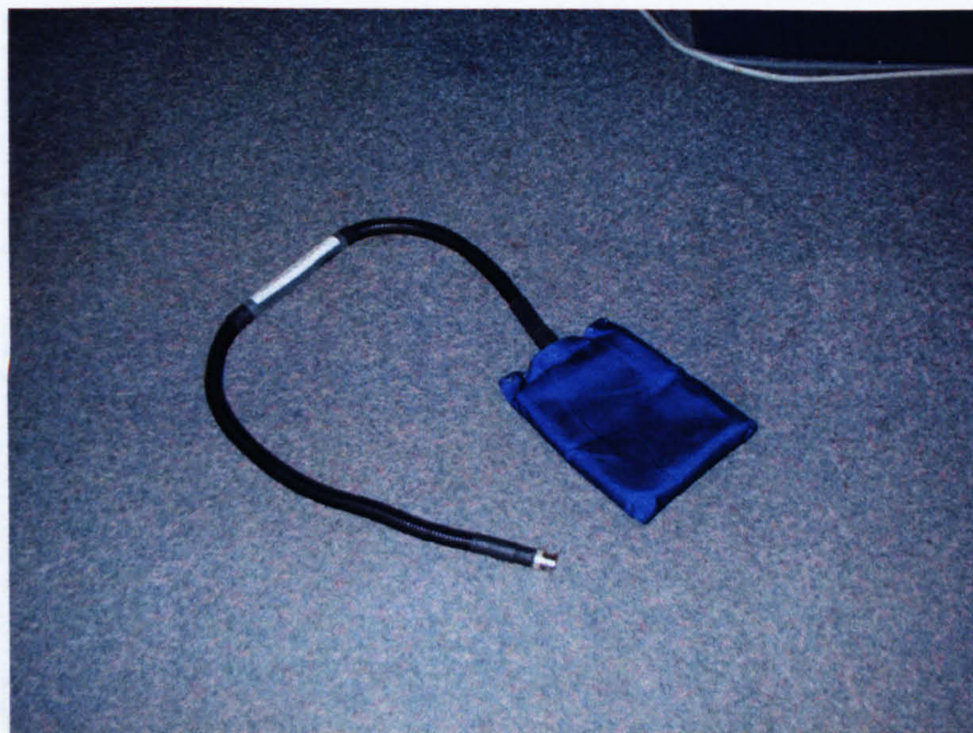
Figure 4.4: The surface coil, of 9 cm in diameter, manufactured by MR Instruments Inc. used in conjunction with TEM coil in this study.
