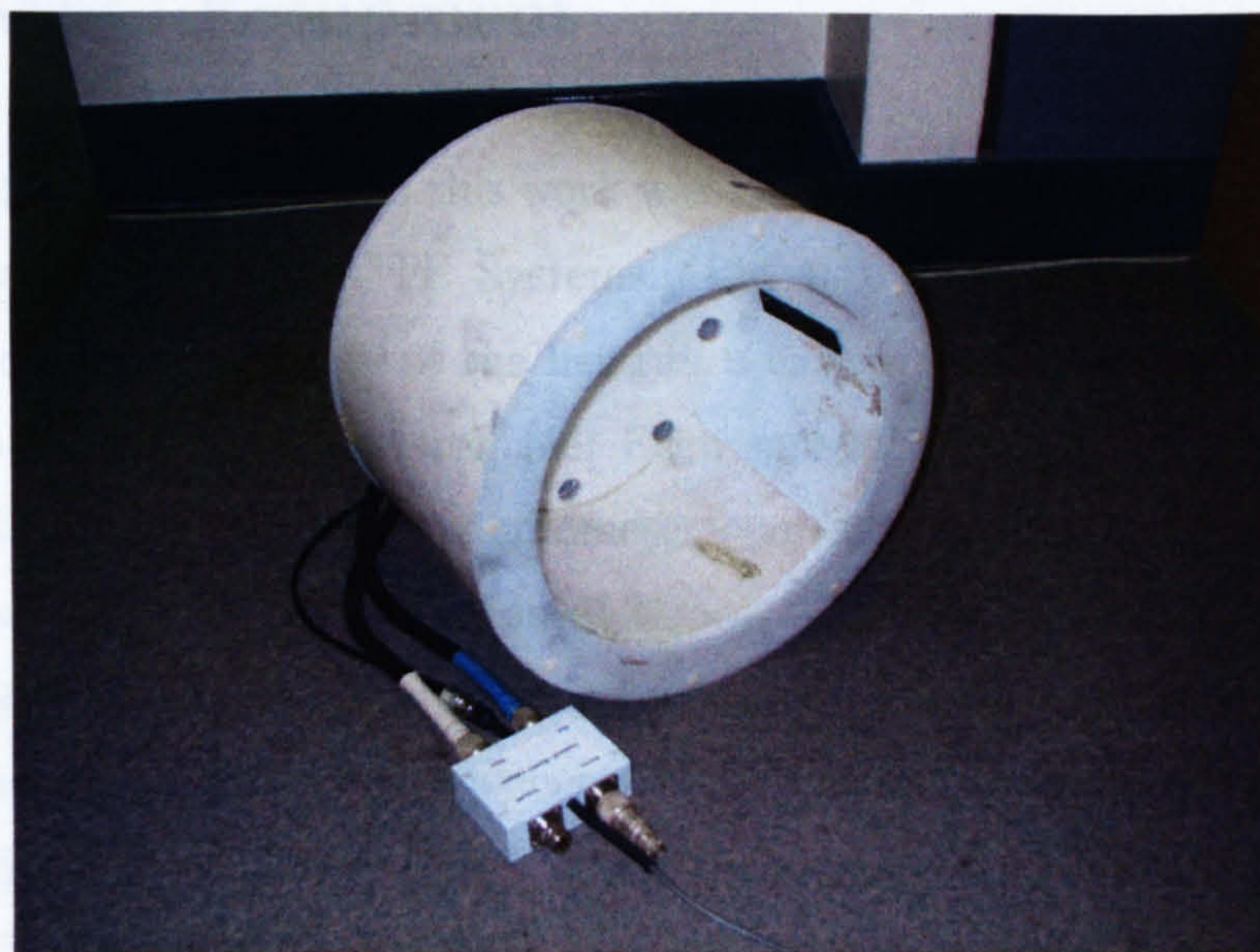
Figure 4.6: The TEM coil, of 26.5 cm in diameter and 23 cm in length, manufactured by MR Instruments Inc. used in this study.
