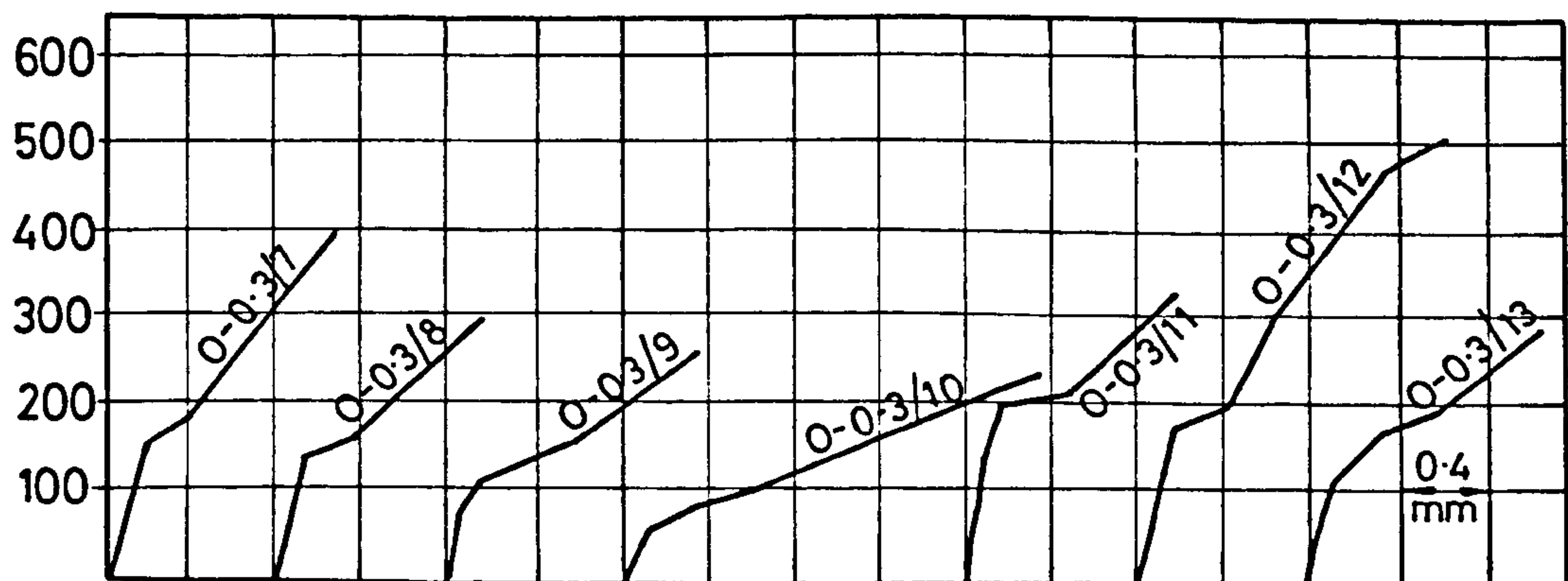
(b) No web steel; x/D = 0.3 ; opening 7-13
