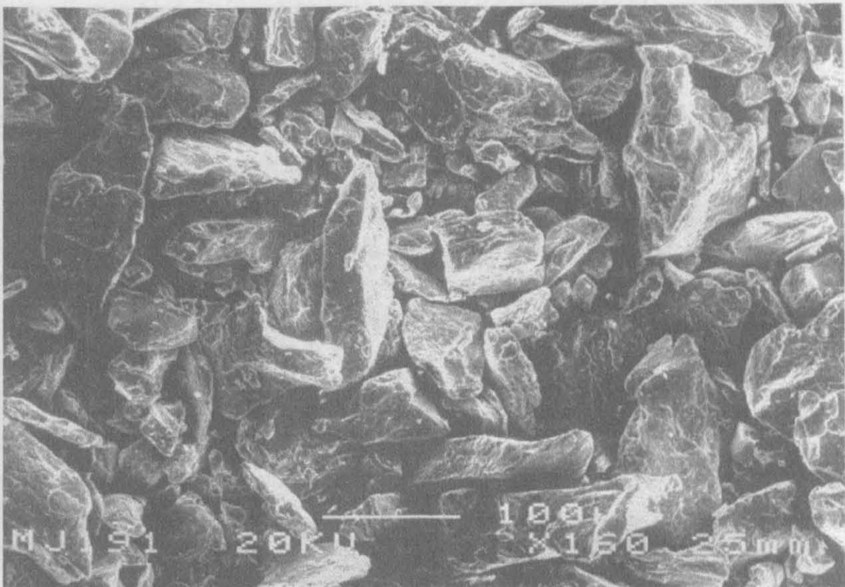
Figure 7.4:Morphology of chromium powder
