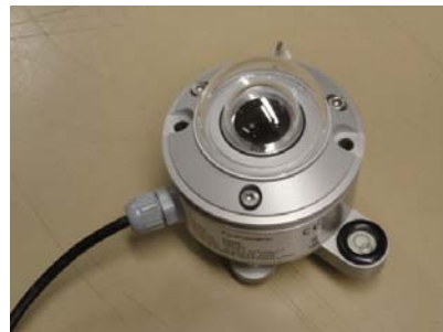
Figure 3-12. Pyranometer for solar radiation measurement.
