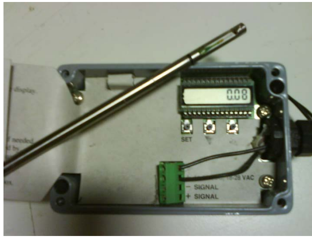
Figure 3-10. The hotwire anemometer.
