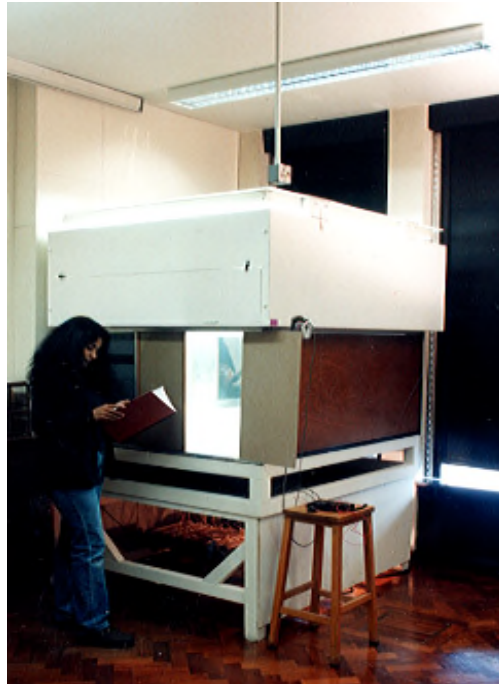
Figure 4:2 Mirror Box Artificial Sky (University of Sheffield)
