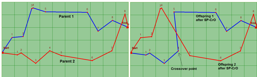
Figure 4.22: Left) Parents before RSPCrO; Right) Two offspring after RSPCrO at point 4
