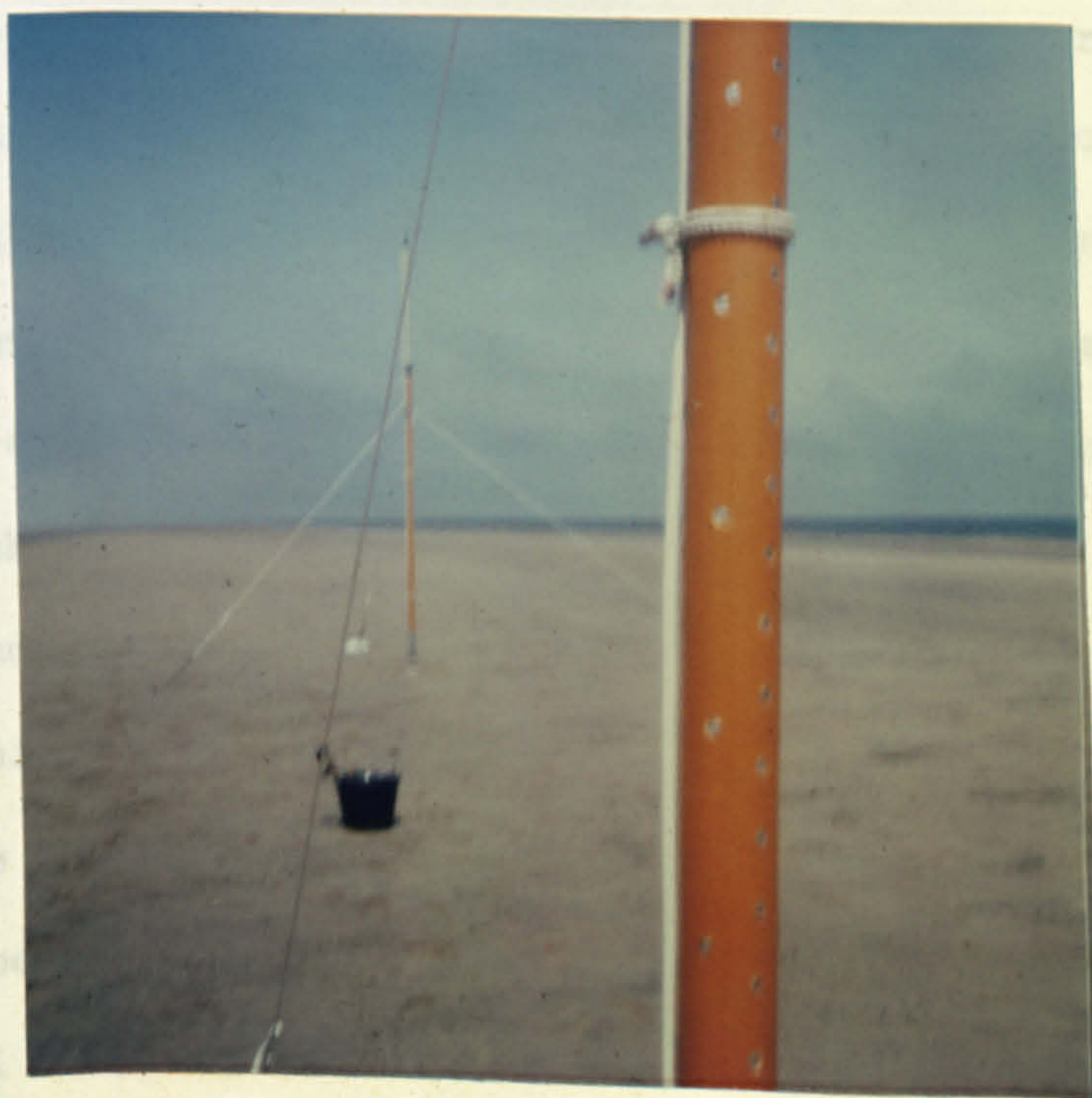
Plate A1.1. Detail of completed wave pole (foreground). Pole fixed to beach face with concrete base and guy ropes (background).
