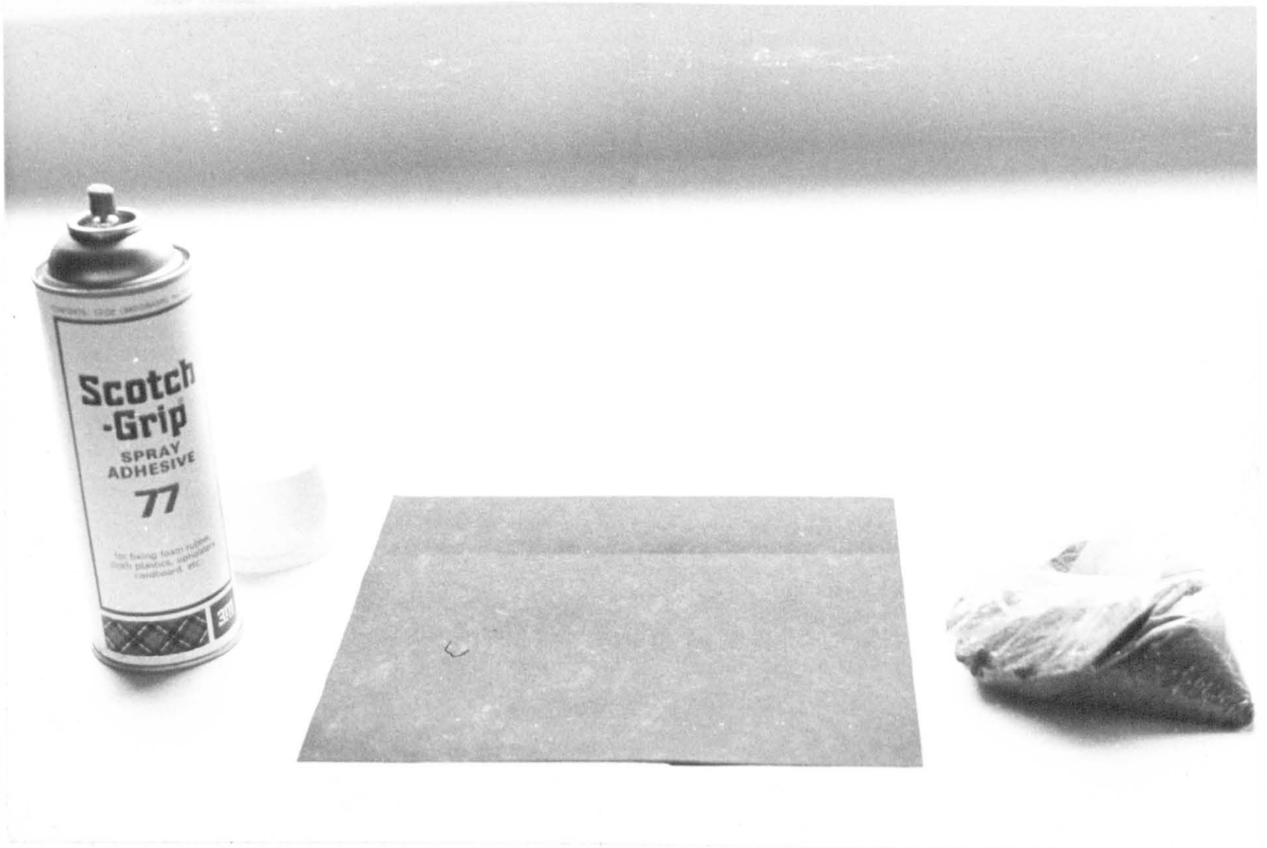
Plate 3.1. Spray glue and black sugar paper used in counting procedure for each sample.
