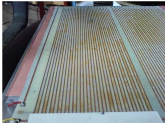
Figure 10.1.1. Detail of burnthrough of electrode sheet after the PEF = 50\text{Hz} experiment. Note discoloured regions and pitted areas of the Mylar material in plasma regions.
