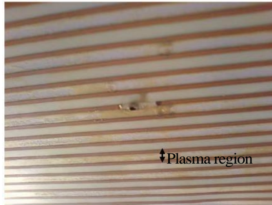
Figure 10.1.1. Detail of burnthrough of electrode sheet after the PEF = 50\text{Hz} experiment. Note discoloured regions and pitted areas of the Mylar material in plasma regions.
