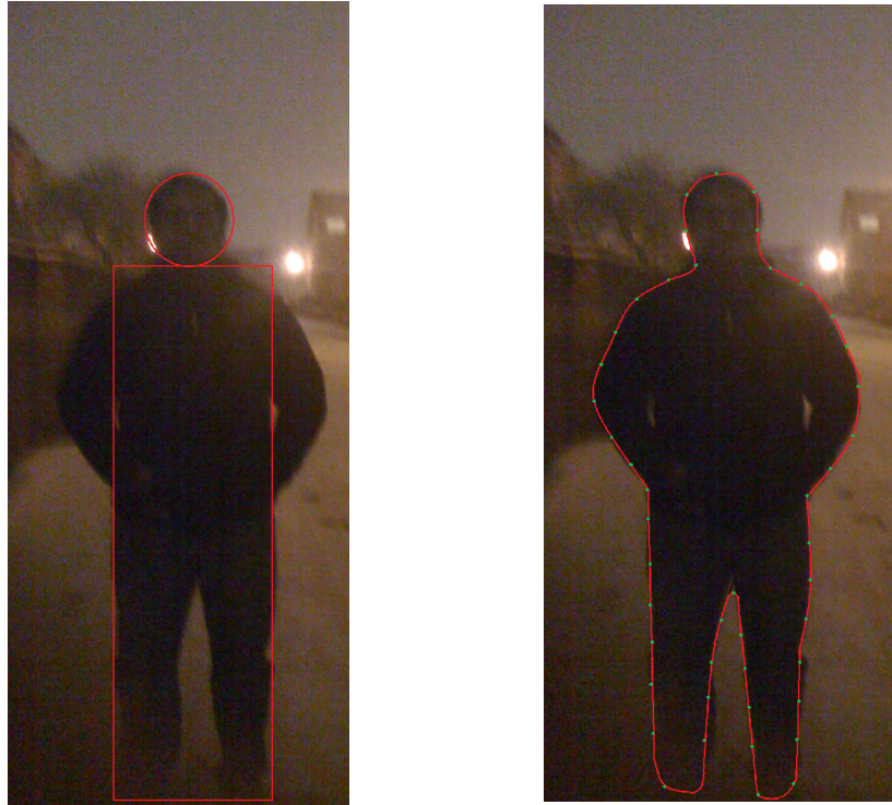
Figure 10. Human Detection using template representation (a) Circle placed over a rectangle (b) Silhouette
