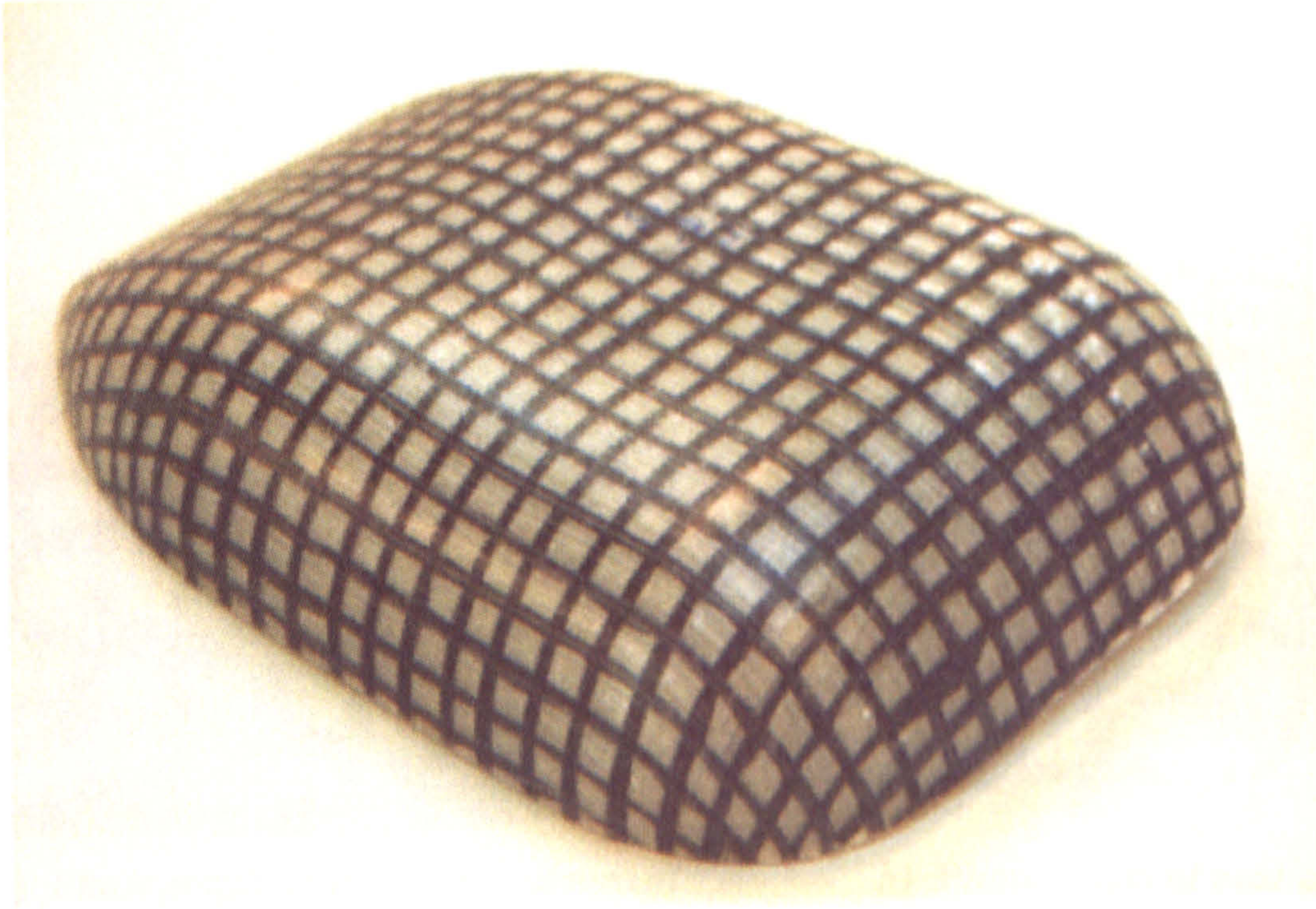
a) Conventional 0°/90° tow placed reinforcement
