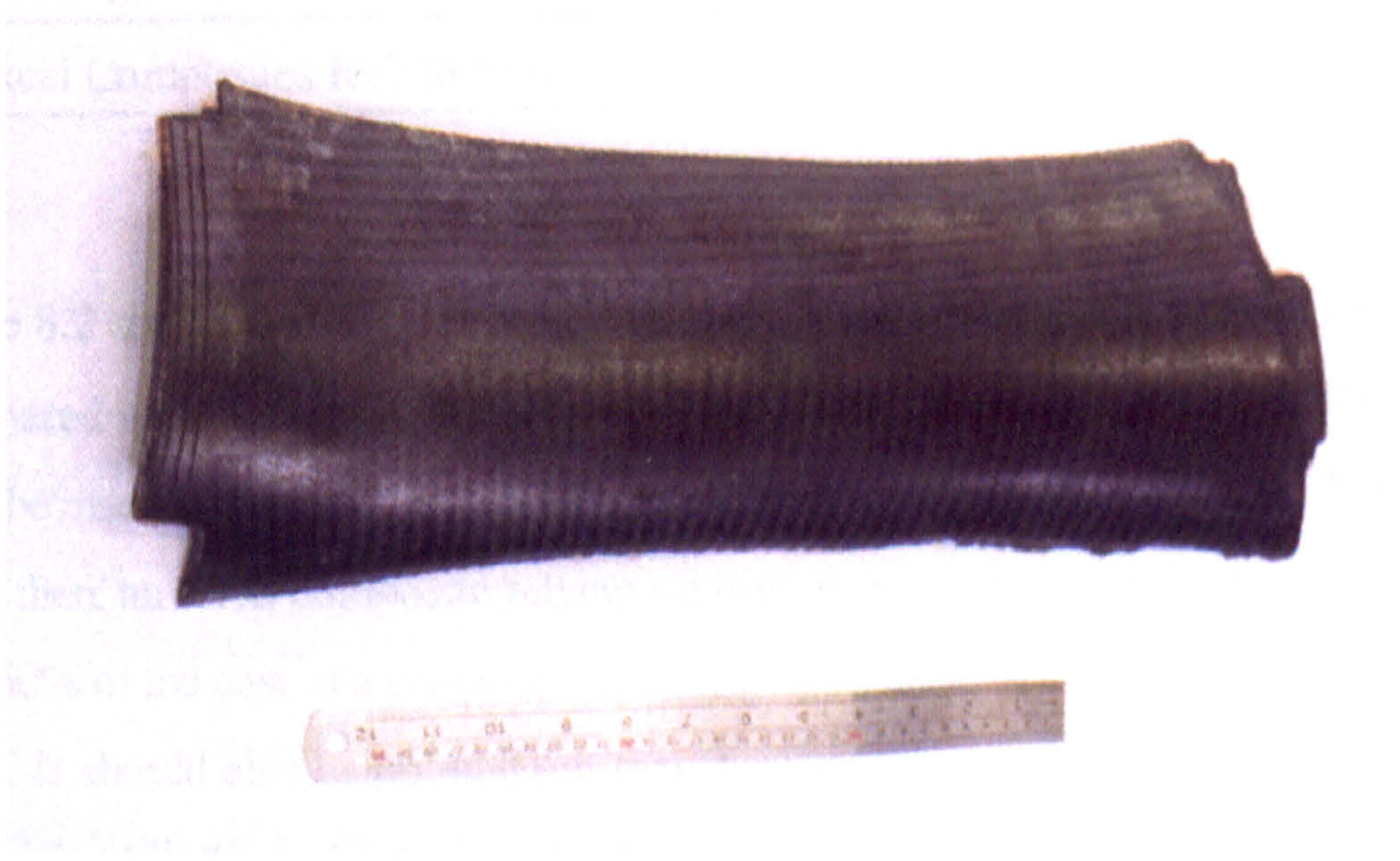
Figure 7.5 Moulded OGV produced using a tow placed preform
