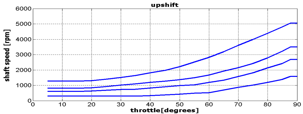
Figure 3-6 Gear up-shift schedules for an automatic transmission, (Rajamani, 2006).
