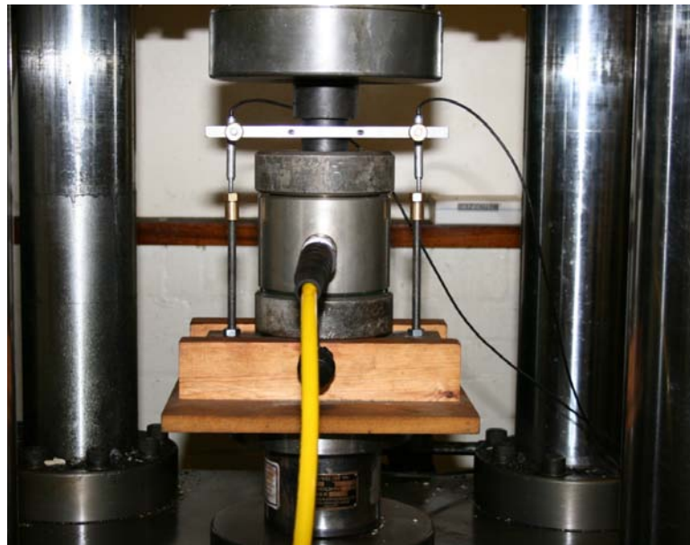
Figure 3.5 Test set up for triaxial compressive tests
