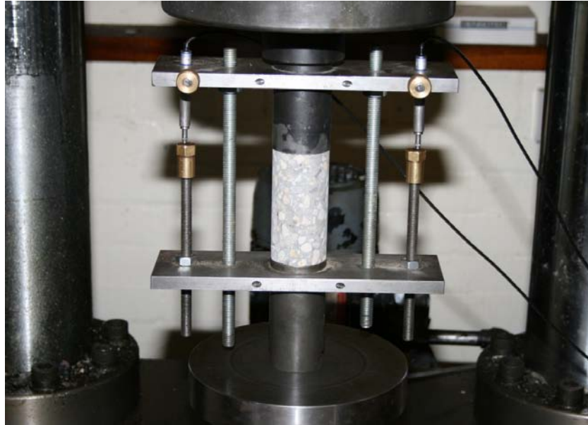
Figure 3.4 Test set up for UCS and Young's modulus
