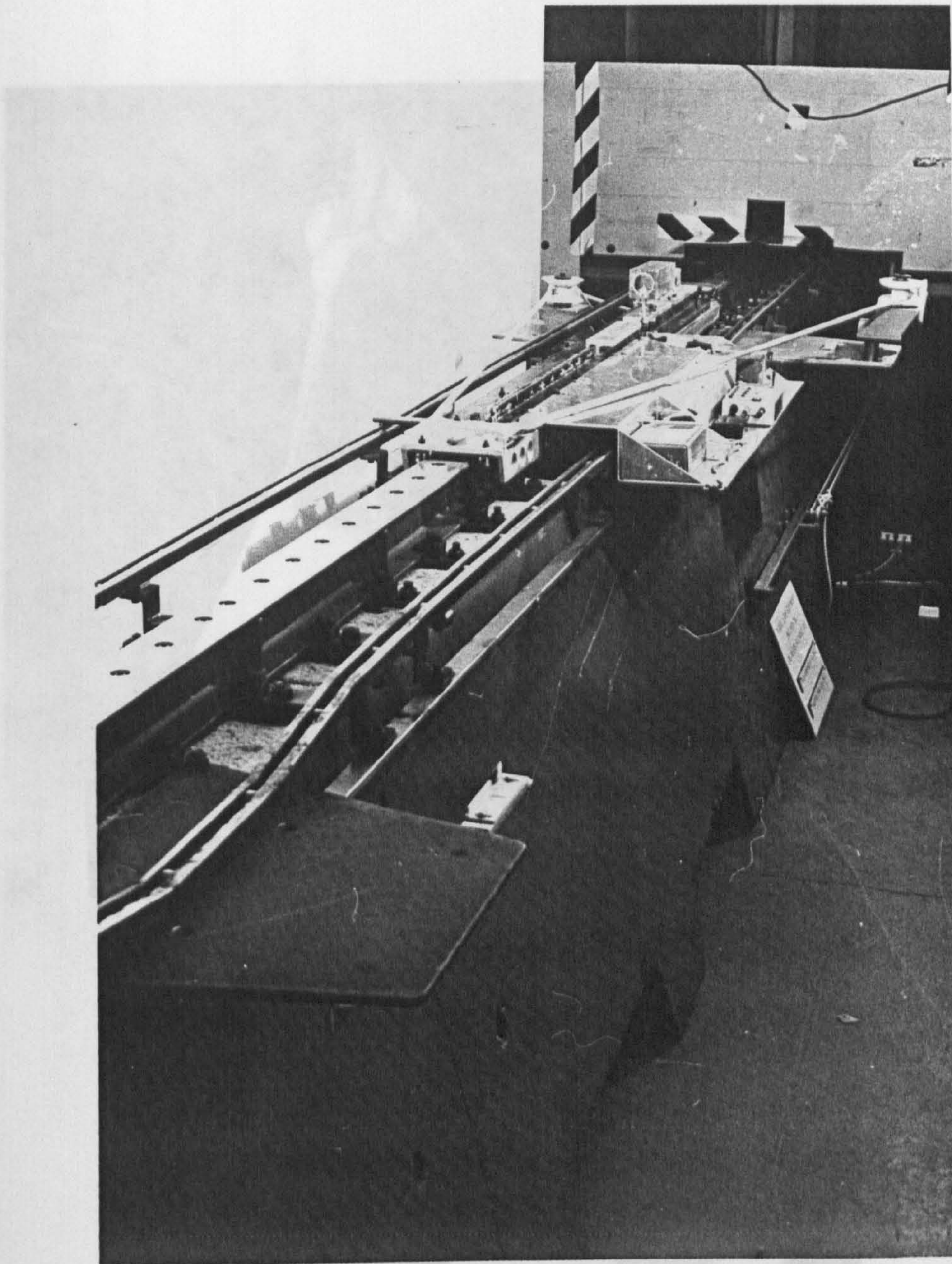
Figure 4.14 The moving model rig used for the first test series. The live trolley being arrested by friction brakes and rubber bungees soon after leaving the working section.
