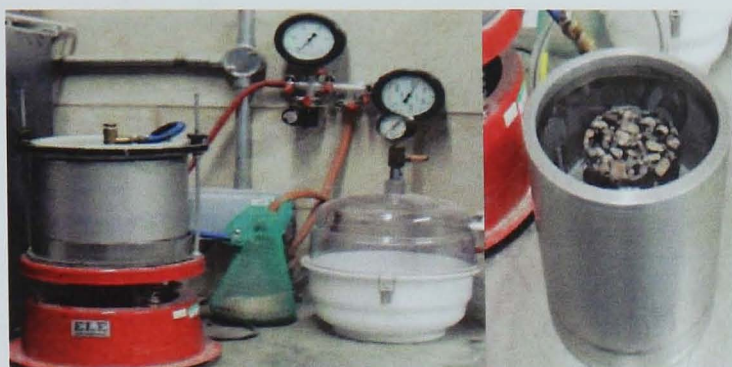
Figure 6.3 Laboratory setting for saturating the specimen
