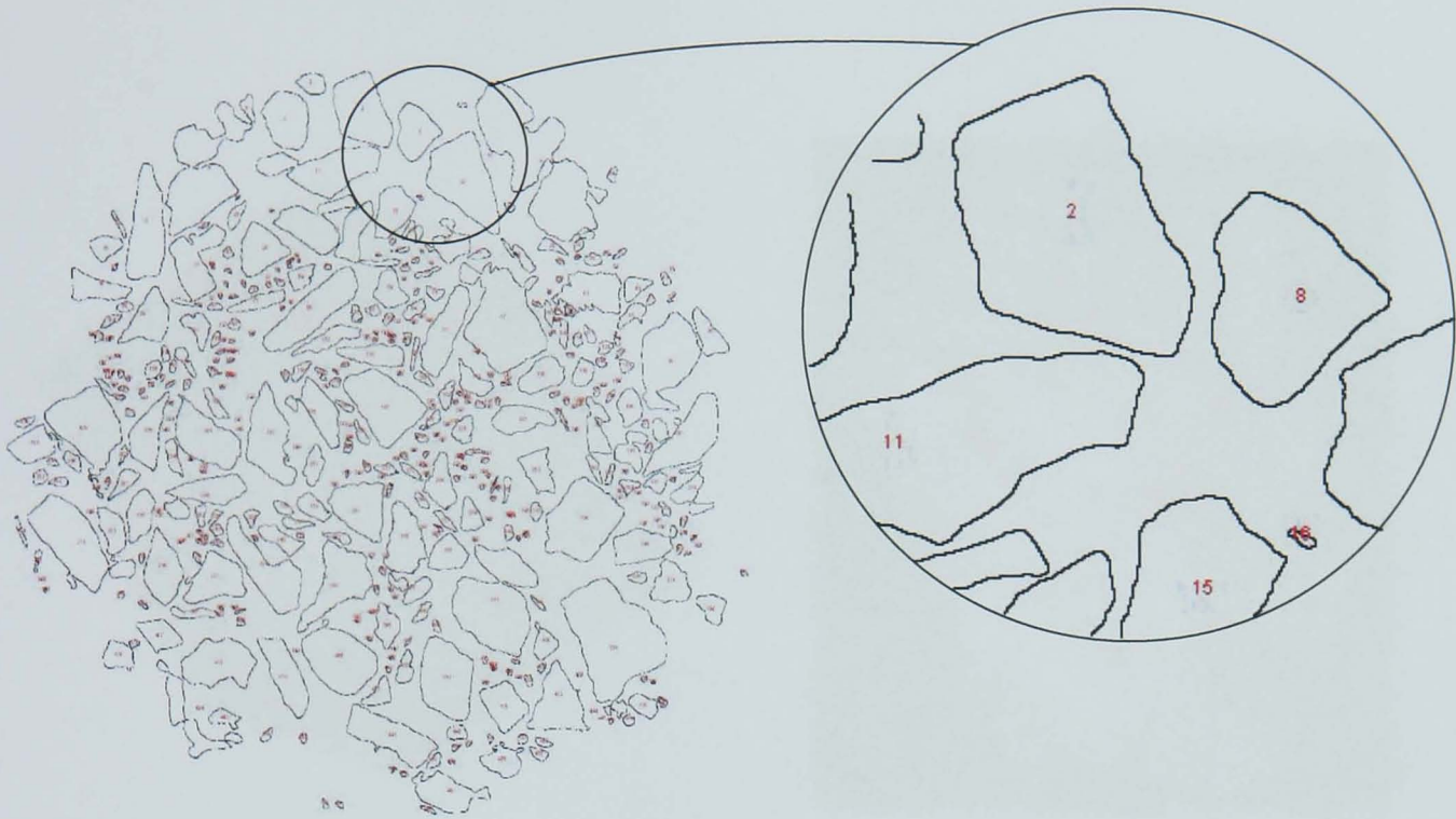
Figure 3.17(b). Aggregate component from 2D image of asphalt mixture
