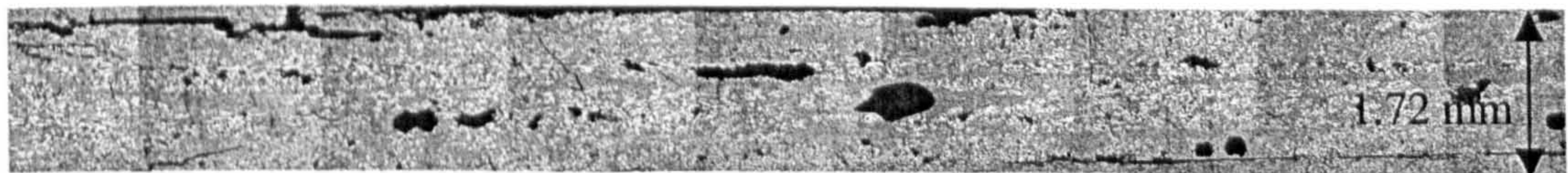
Figure 5.3 Laminate consolidated for 40 seconds with a void content of approximately 6.5%.
