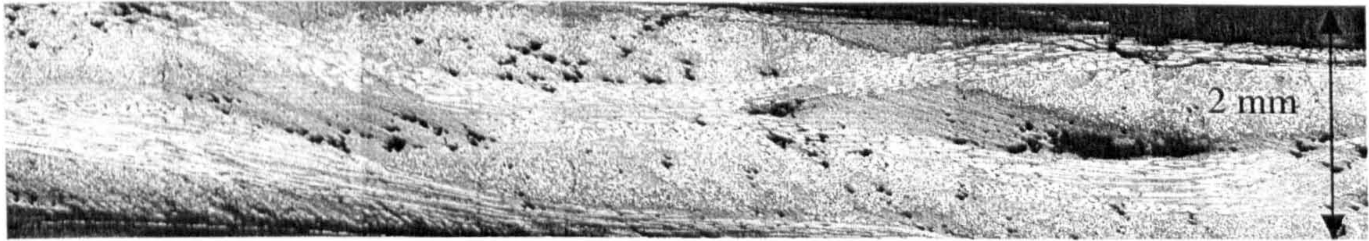
Figure 5.8 Commingled glass/PP laminate consolidated by pressure forming [52].
