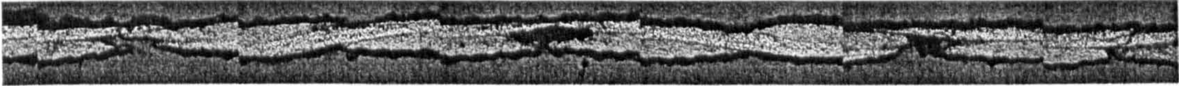
Figure 4.19 Micrograph of a single ply, at 45° to the warp direction. The micrograph showed 7.98% void content.
