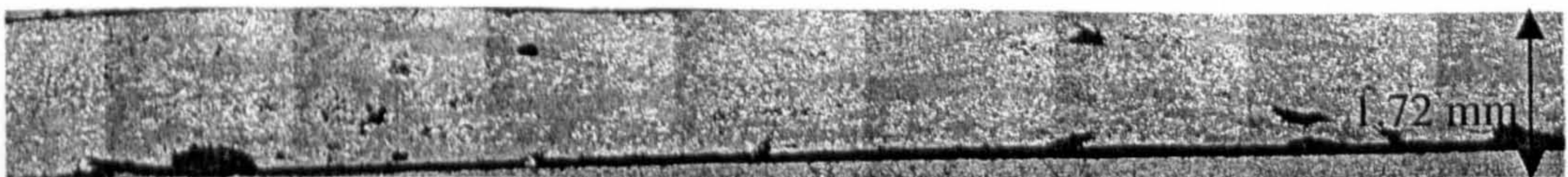
Figure 5.4 Laminate consolidated for 60 seconds with a void content of 4.5%.
