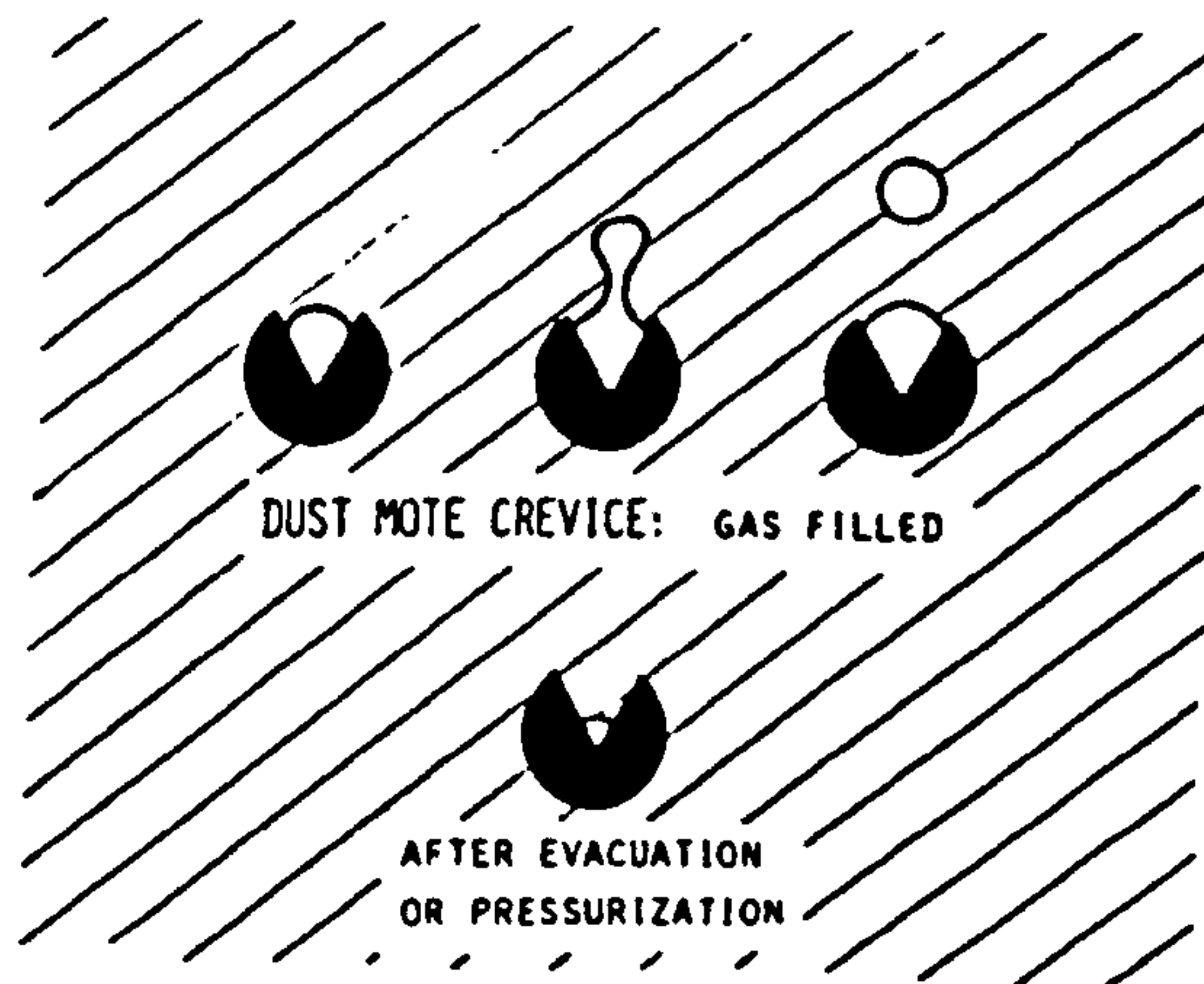
Figure 1. Nucleation of acoustic cavitation
