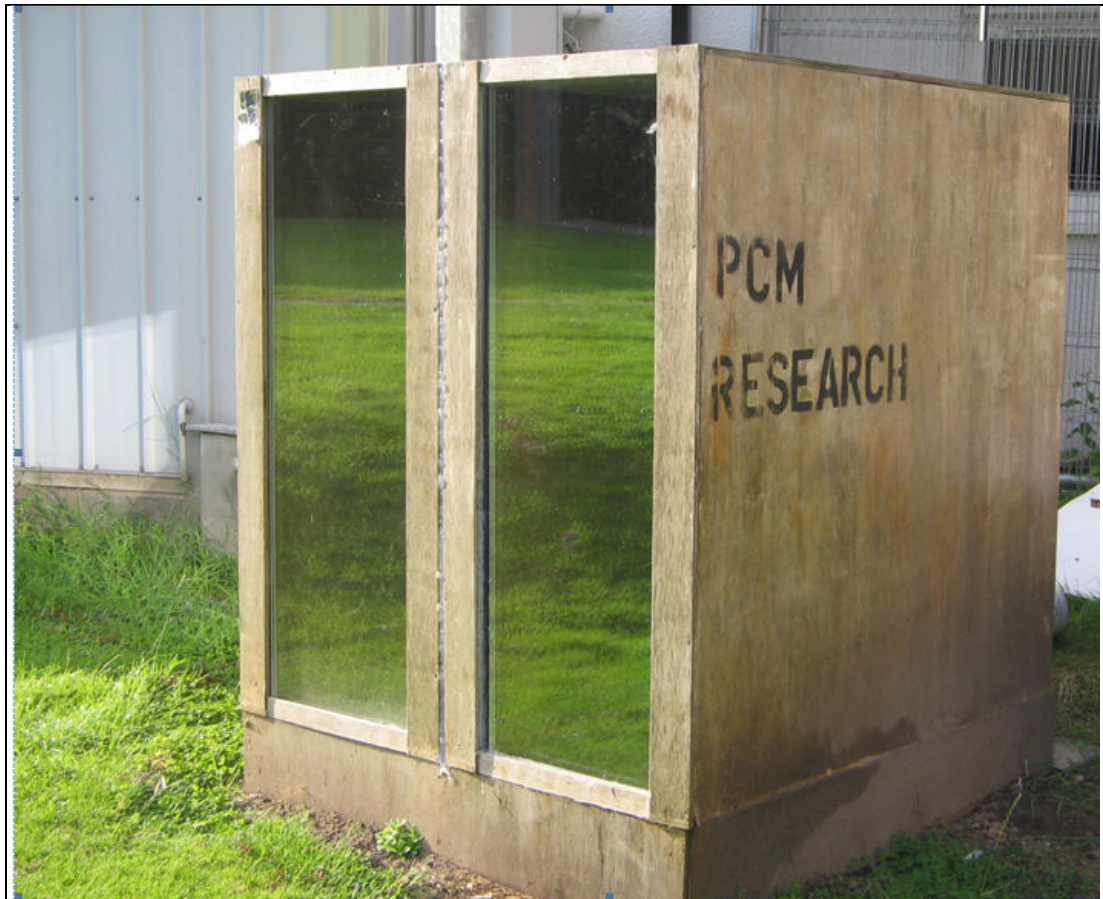
Figure 8.5: Outdoor PCM test box with 2 identical chambers
