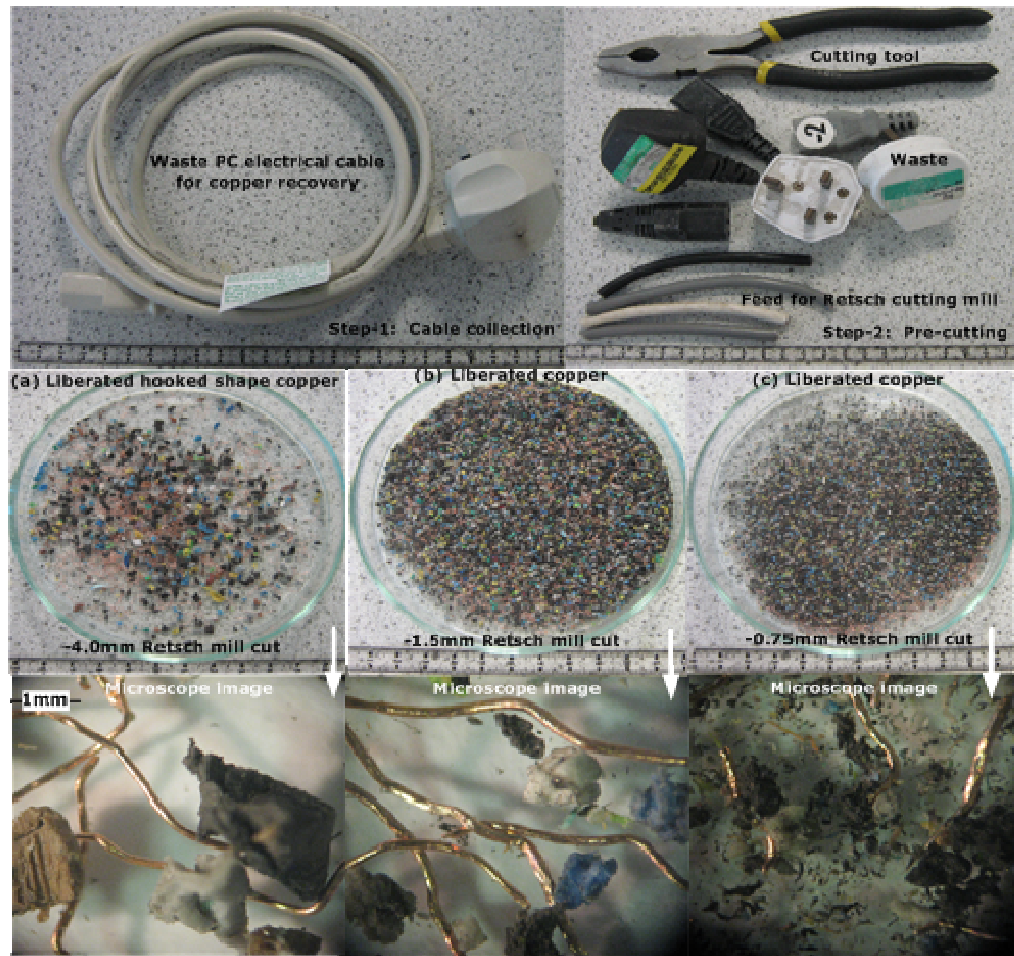
Figure 7.2: Feed preparation steps for vibration separation of waste PC electrical cables.
