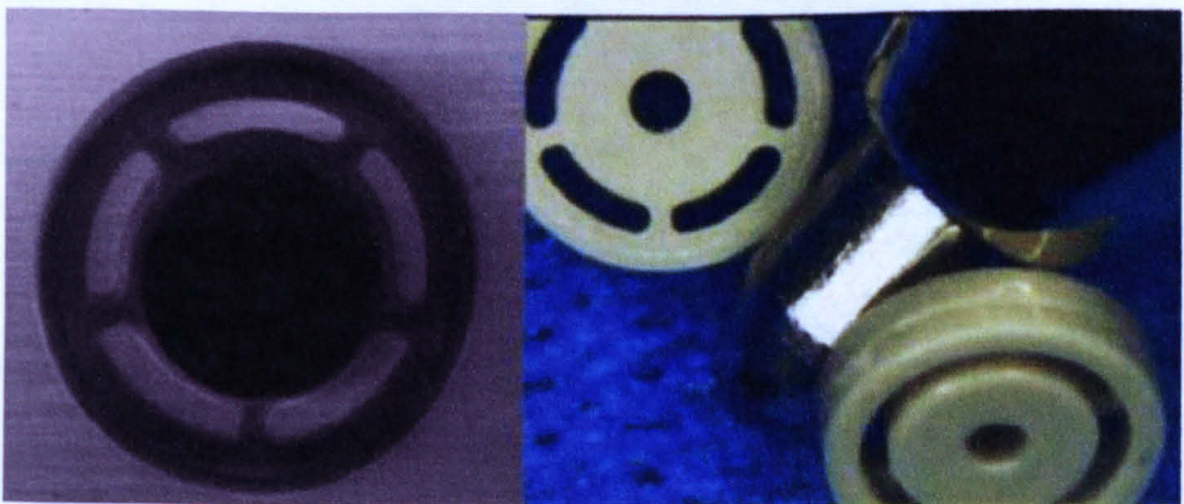
Figure 2.9 Micro-mould (tyre-rim for micro car) on steel (SAE H13) [131, 149]
