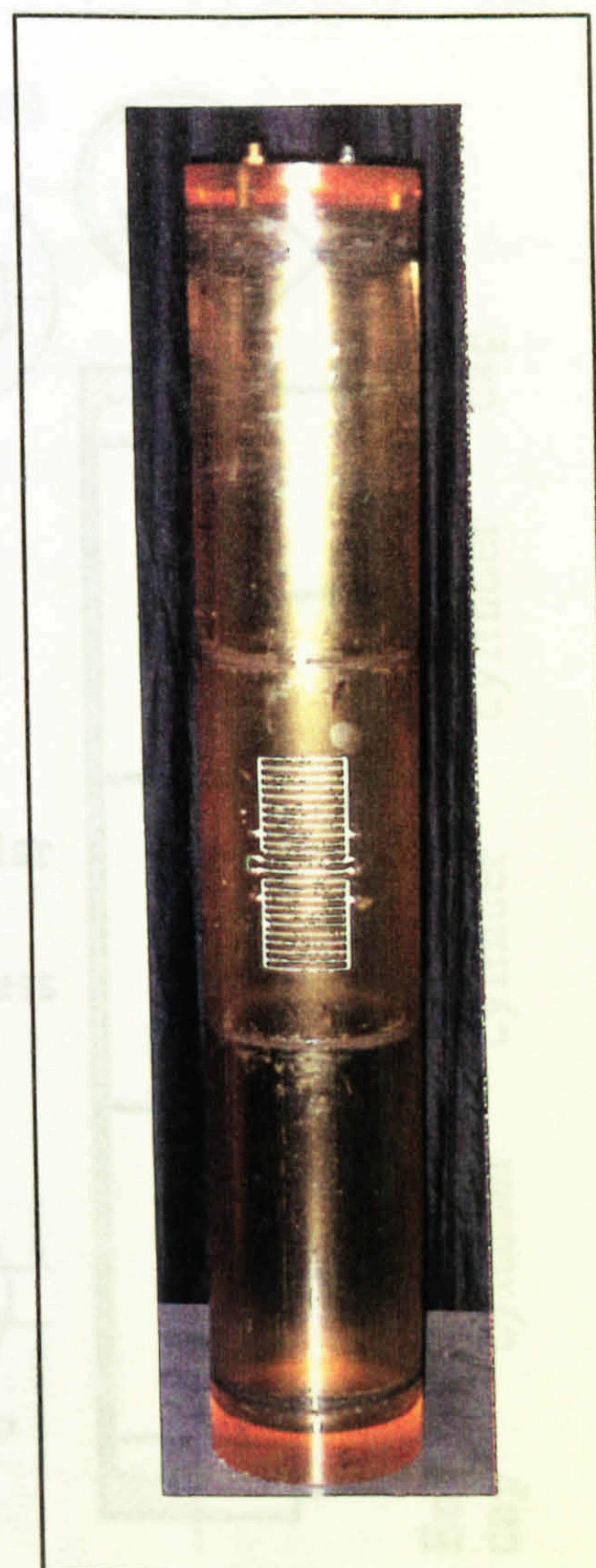
Fig. 9.1. Photograph of a pressure tube prior to testing.
