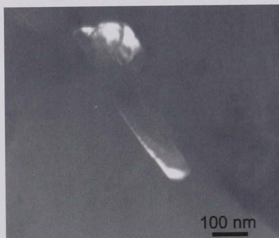
Figure 4.1.12. An end-on perspective of an M_{23}C_6 particle ( SP10 Grip ) Zone axis = [-2-11] a = 10.6599 \text{ \AA}
