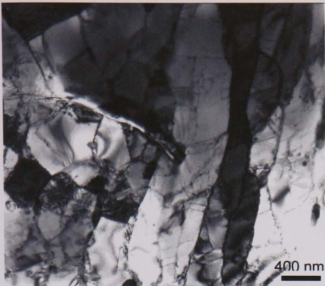
Figure 4.1.10. TEM bright field image (thin foil) showing martensitic lath (subgrain) morphology in the as-PWHT P91 parent metal.
