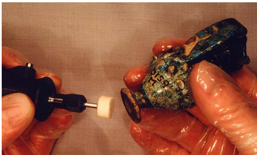
Figure 4.19 Sample preparation for XRF analysis- polishing archaeological artefact (sample 10).
