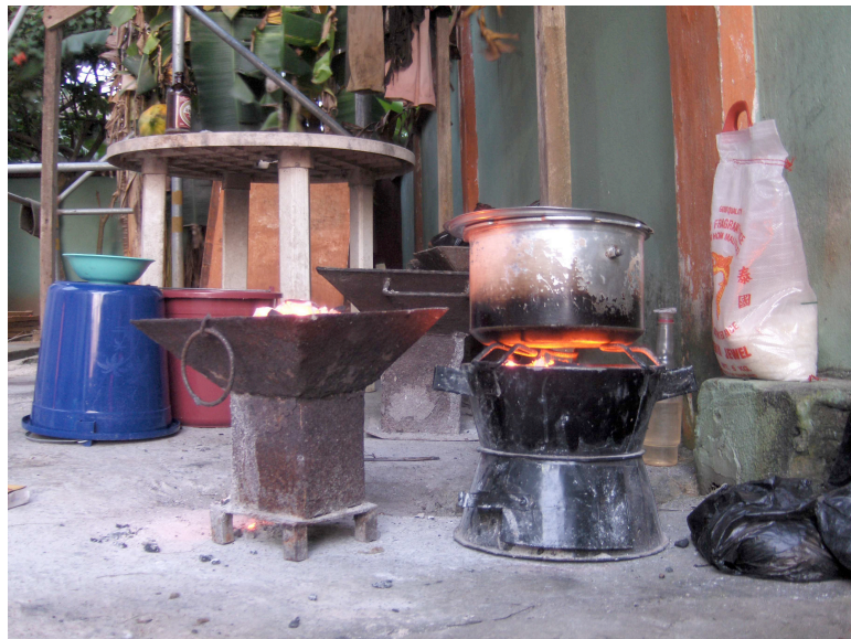
Figure 1.3: Charcoal is commonly used as a cooking fuel especially in the urban areas. On the left we have the traditional charcoal stove, known as the coalpot and on the right a popular improved charcoal stove, the Gypa stove. The Gypa stove is more thermally efficient than the coalpot, and ash is collected in a compartment below the charcoal, making it cleaner to use [6].
