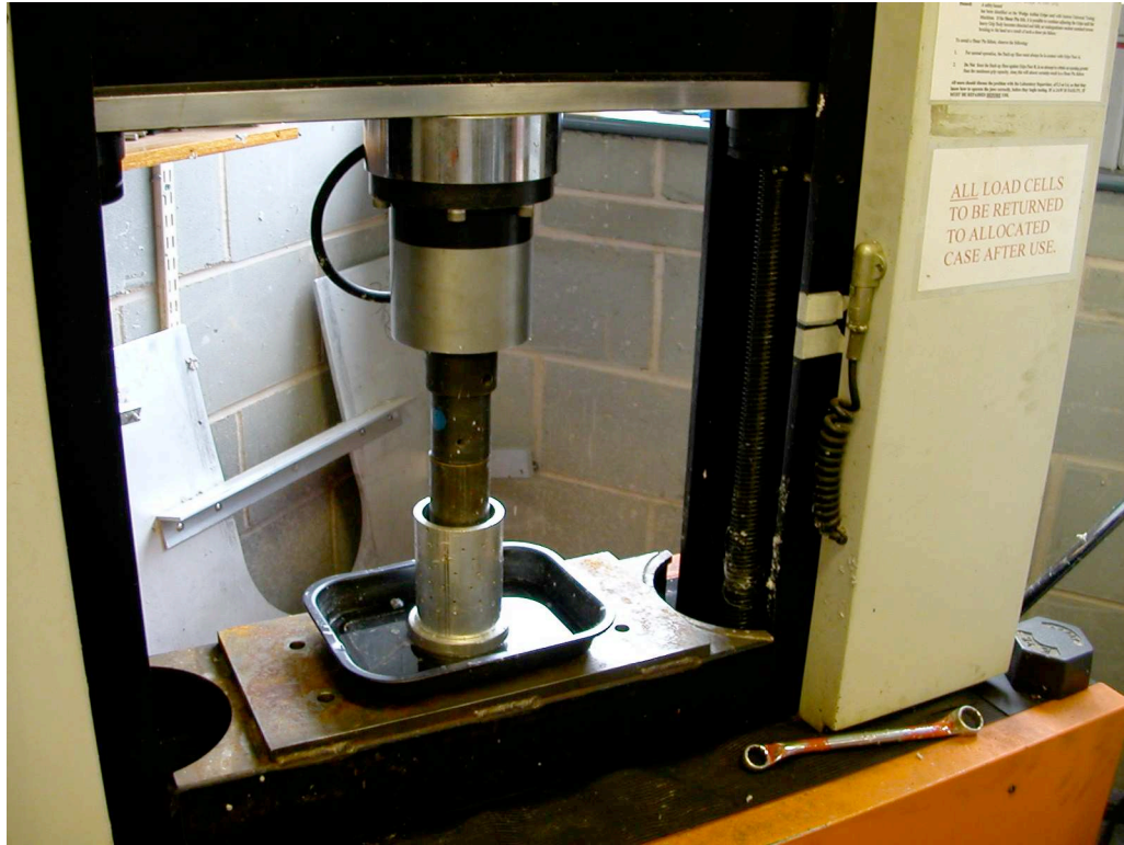
Figure 3.1: The Instron compression machine used for forming the briquettes. A cylindrical mould used to form briquettes with a central hole can be observed. Notice the small holes riddled around the mould to allow the expulsion of water from the pulp during compression.
