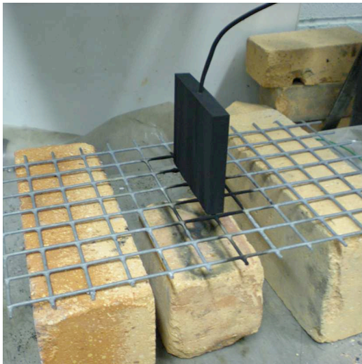
(a) The experimental set-up of the slab experiment: An aluminium slab was placed on a mesh grid with a thermocouple to monitor its temperature. N.B. the slab is black because it is covered in soot.
