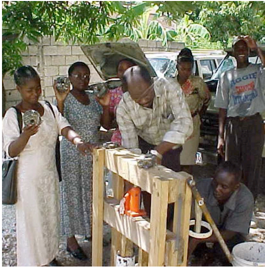
(a) A press that uses a car jack
