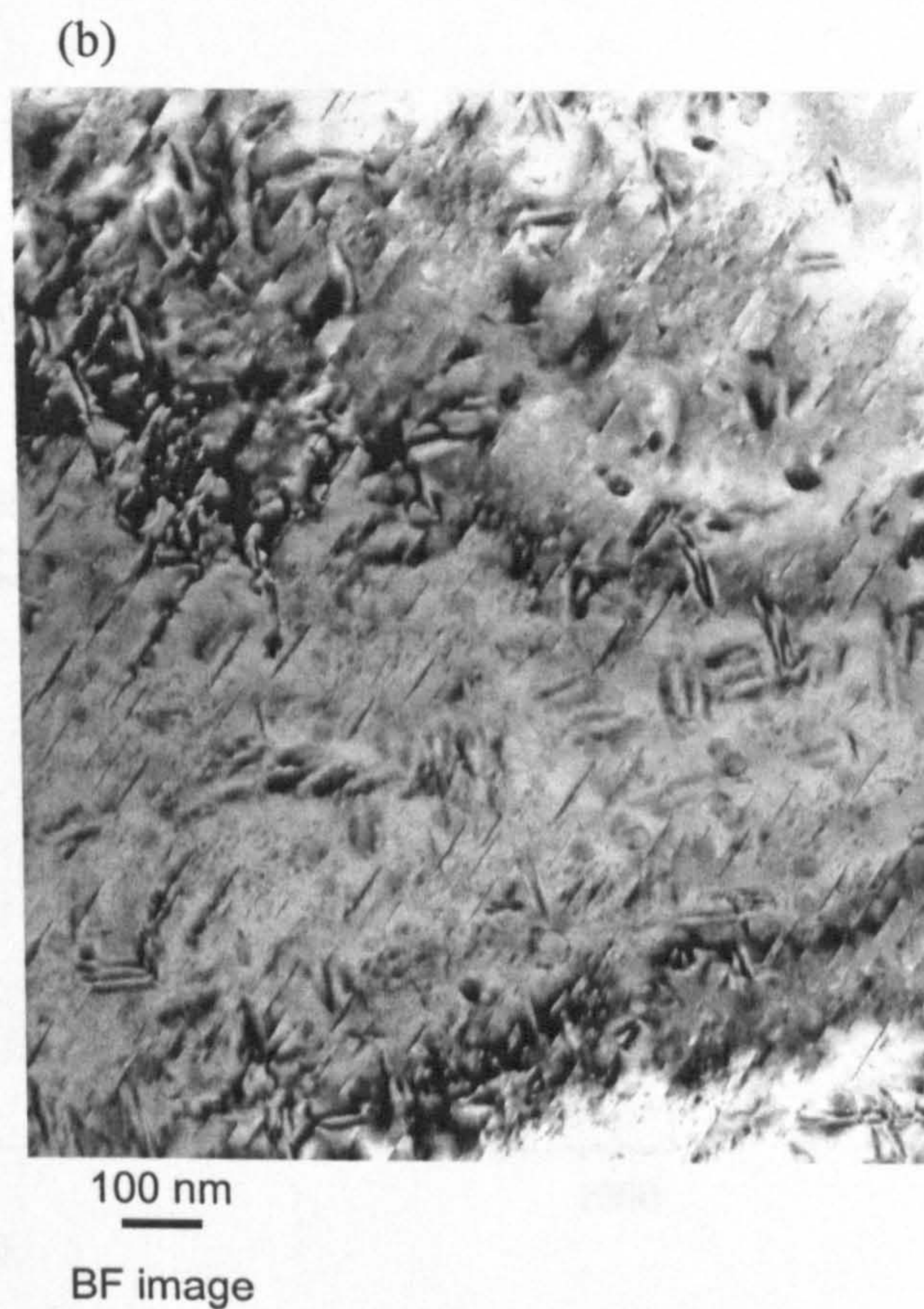
Figure 9.36 (a, b): TEM images of 1.7Li3.0Cu alloy aged for 7 days at 100°C after exposure for 1000h at 70°C . Zone axis \langle 001 \rangle .
