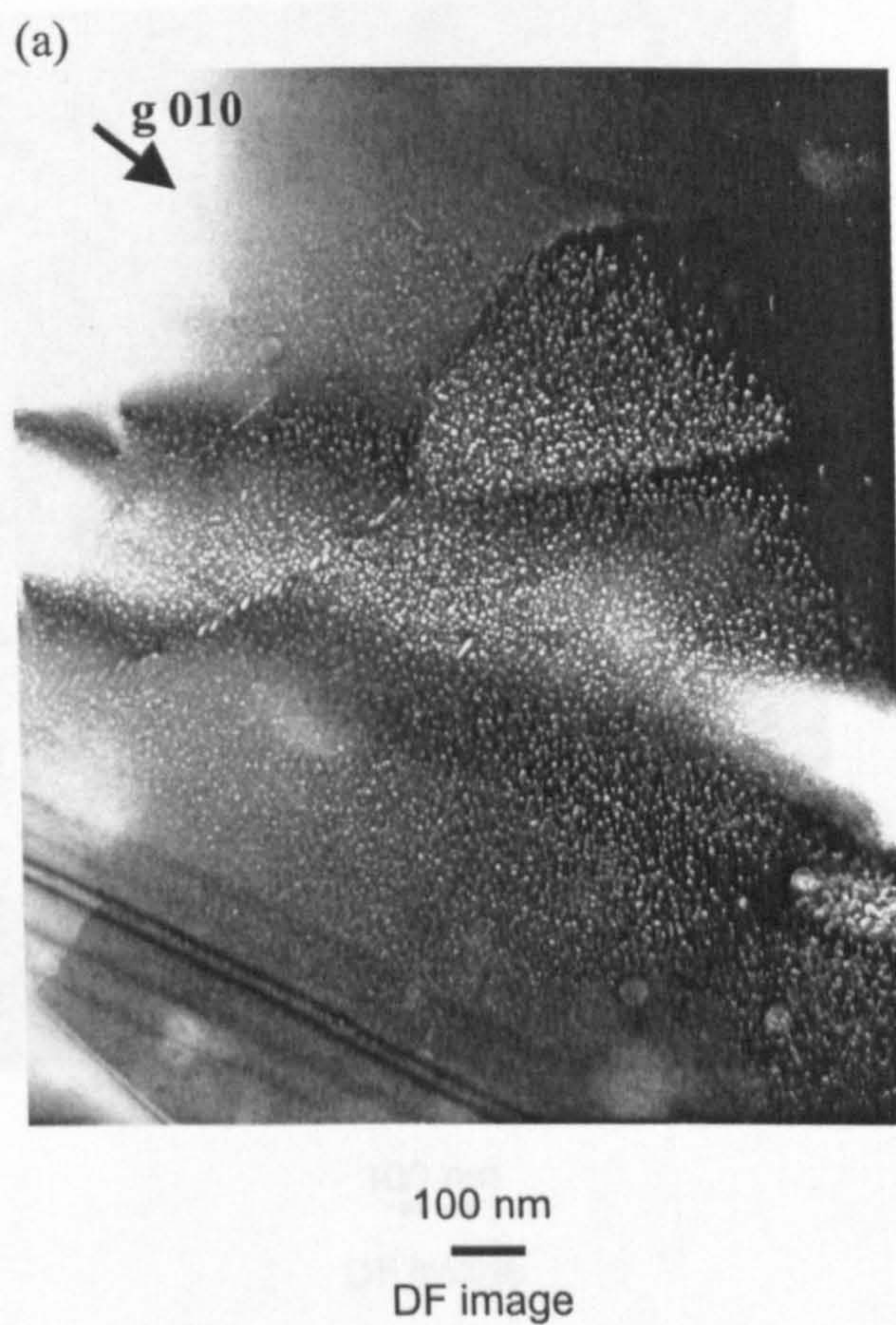
Figure 9.12 (a): TEM image of 1.7Li1.2Cu alloy after ageing for 1000h at 100°C. Zone axis \langle 001 \rangle .
