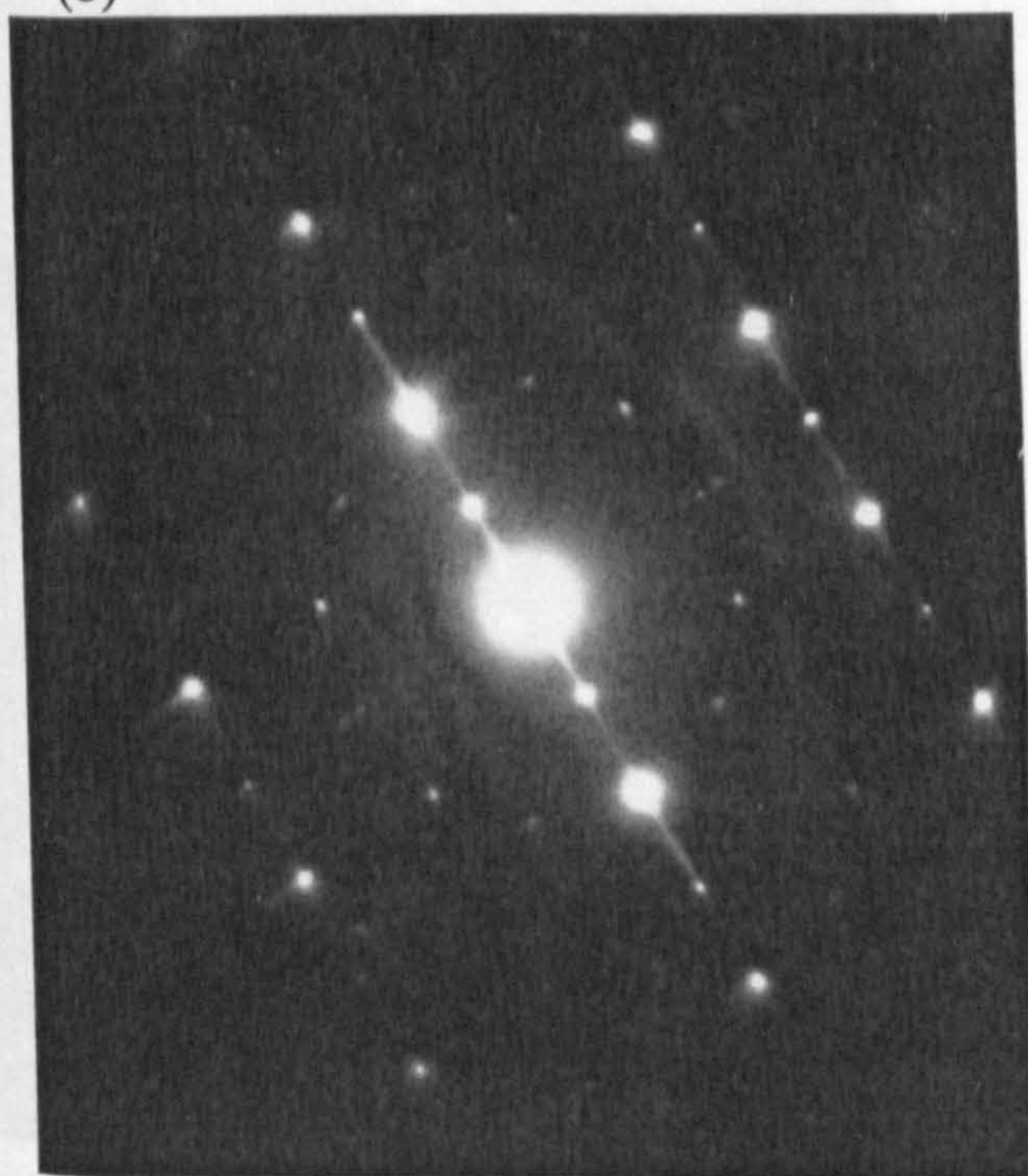
Figure 9.35 (b): SAD pattern of 1.7Li3.0Cu alloy after exposure for 1000h at 70°C . Zone axis \langle 013 \rangle .
