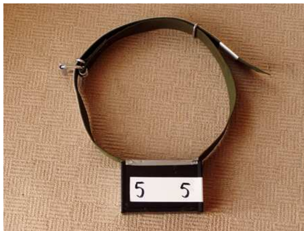
Figure 3.3. Collar with a GPS receiver and a mobile phone
