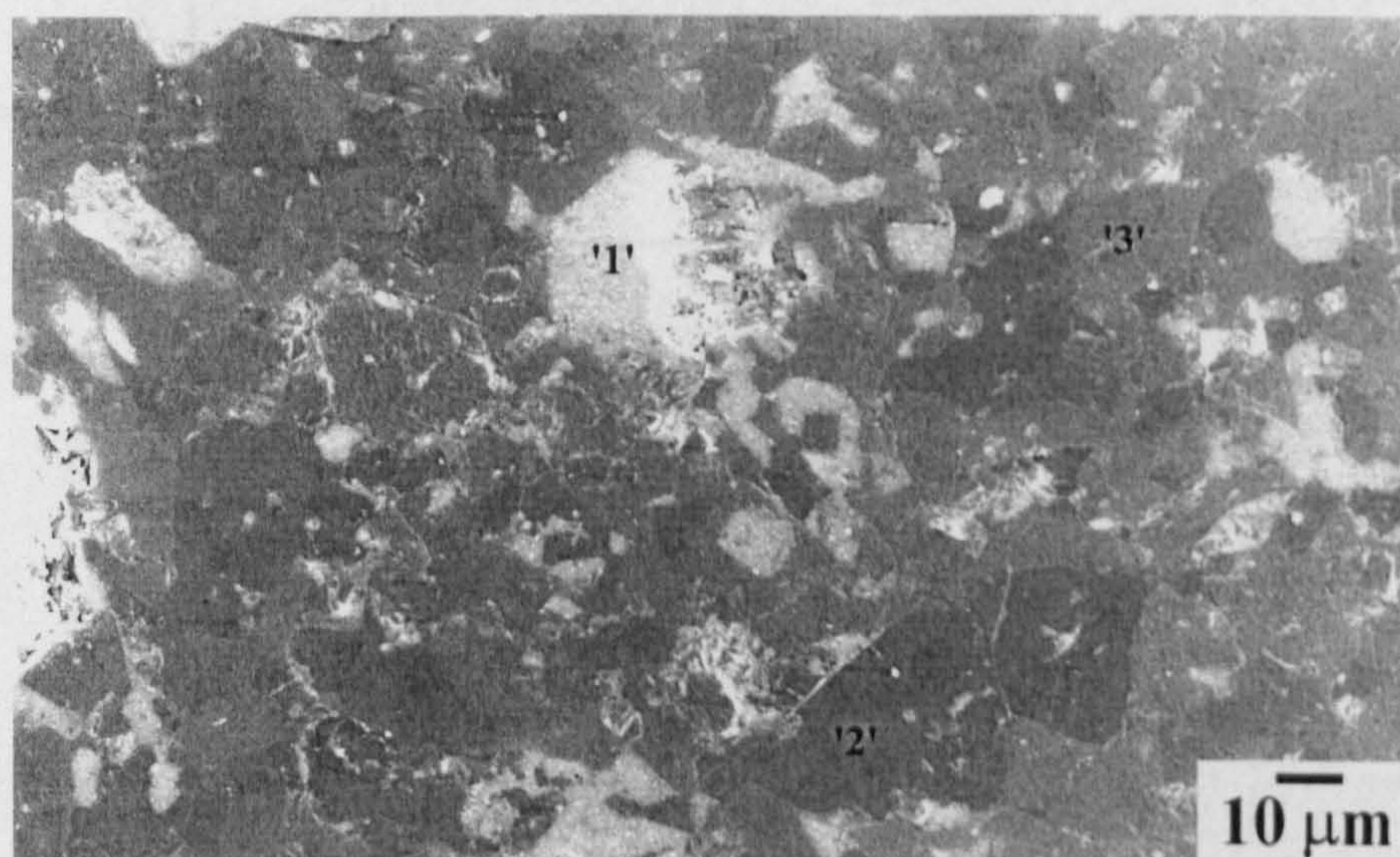
Fig. 6.25 Worn surface of Al 2 O 3 ball slid against sintered carbide disc at load 3.57 kg showing (a) the wear scar with material loss leading to pore formation and (b) high magnification image in the centre of the wear scar indicating the grain structure of Al 2 O 3 and holes filled up with mixed wear debris.
