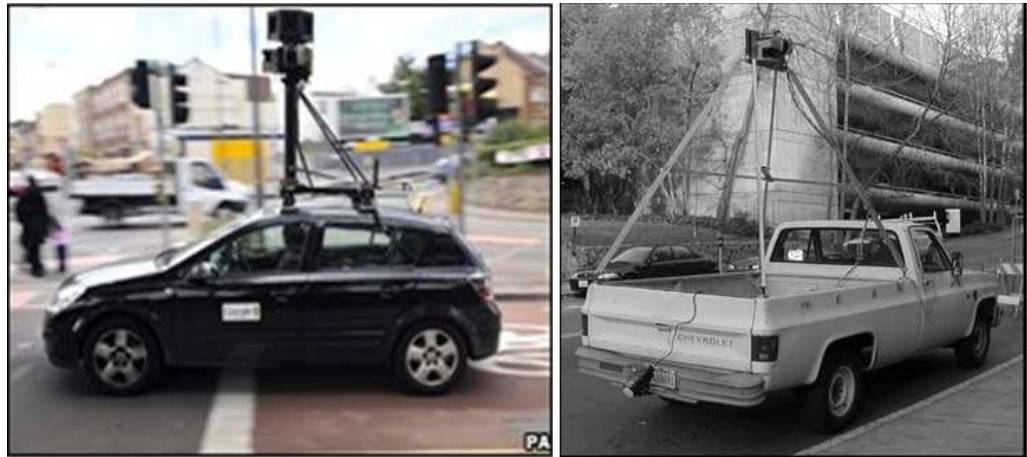
Figure 2.15: (Left) Street View car with its camera mounted on the roof used by Google Earth to capture home facades, adapted from: http://news.bbc.co.uk/1/hi/england/beds/bucks/herts/7980737.stm , (Right) truck with acquisition equipment that was used by Frueh and Zakhor (2004).
