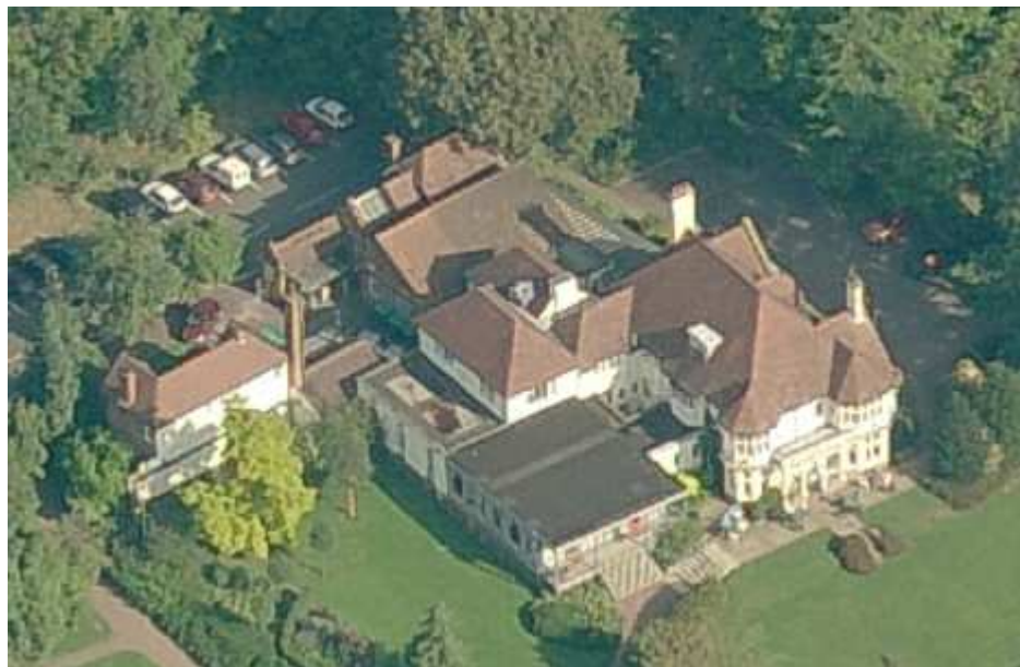
Figure 2.10: A building in Nottingham University campus with occlusion due to vegetation, Pictometry oblique aerial image.
