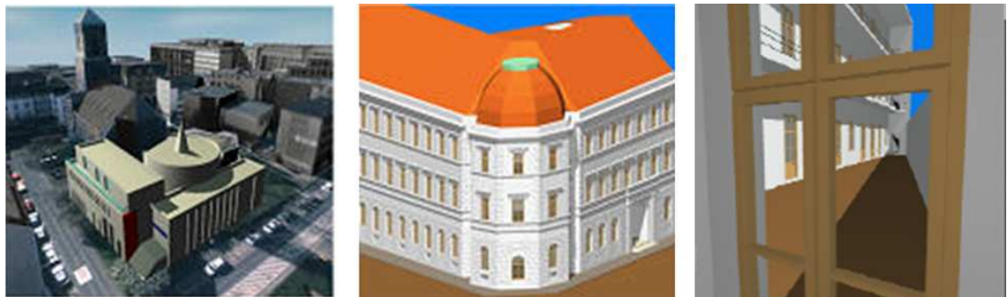
Figure 2.20: Left: LoD2; site model with roof structures and added textures, middle: LoD3; detailed architectural model, right: LoD4; interior walkable model, adapted from (Kolbe et al., 2005).
