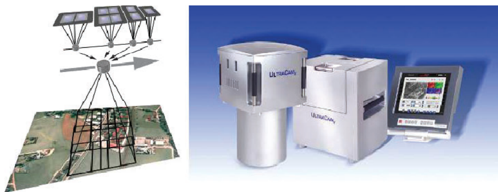
Figure 3.5: Left; concept of the Microsoft UltraCam large-format digital camera, showing the arrangement of the four lenses mounted along the flight direction and the multiple CCD area arrays that are used to generate the final panchromatic image. Right; the principal components of the Microsoft UltraCamX model with (from left to right) the camera unit with its recessed handles; data storage unit; and user display screen (source: Microsoft, 2009).
