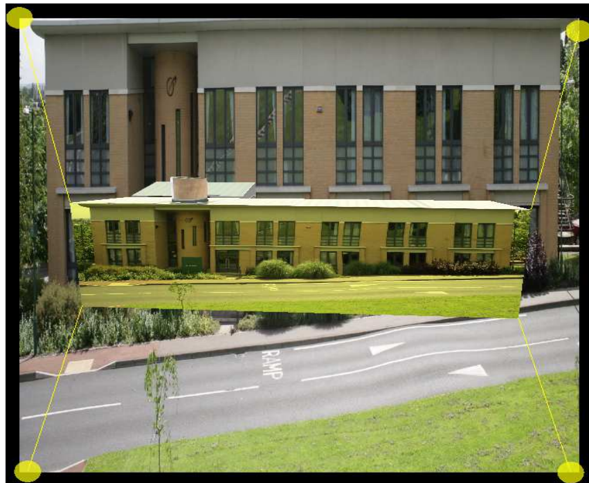
Figure 7.5: Vertices of 3D model and the terrestrial image used for texturing should overlay each other.
