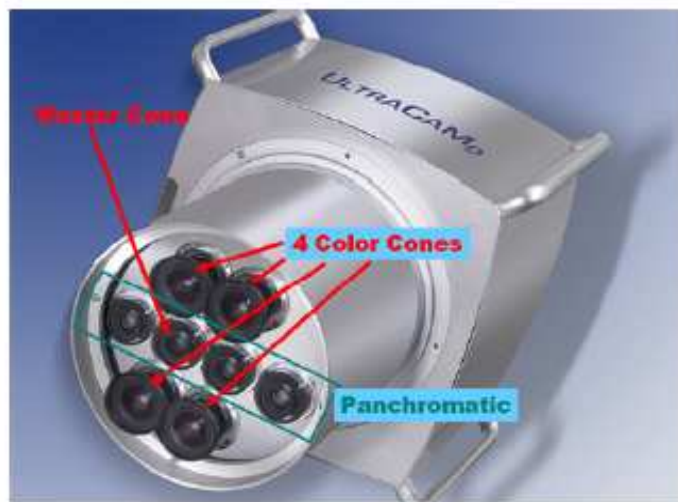
Figure 3.20: Microsoft's UltraCamD large format digital camera showing the sensor unit of the camera which consists of eight independent cameras, so-called cones; the middle four create the large format panchromatic image at a size of 11500 by 7500 pixels. The other set of four cones is responsible for the multi spectral channels of the UltraCamD (source: Vexcel, 2007).
