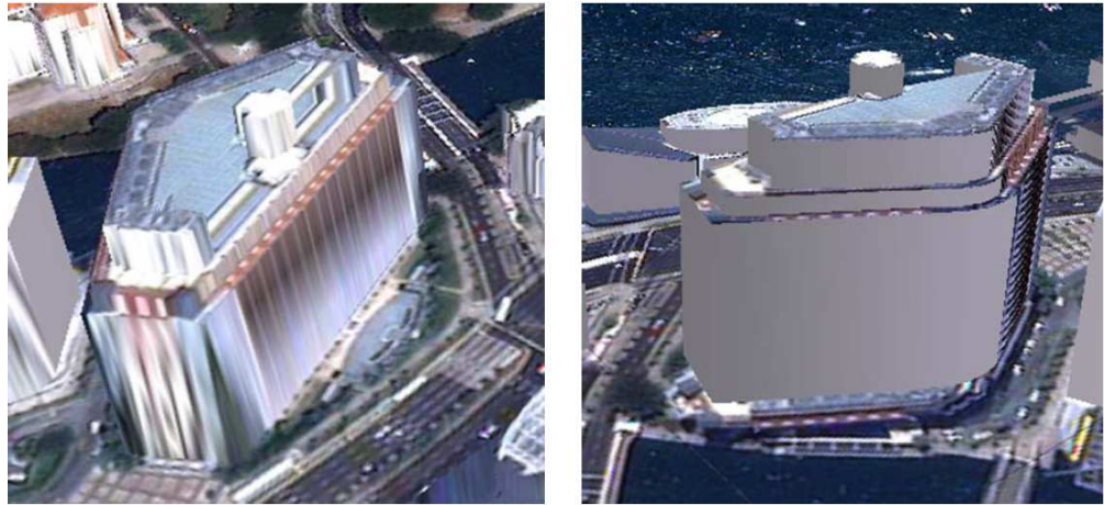
Figure 2.12: Front and back views of a 3D building model textured using IKONOS imagery, adapted from Huang et al. (2006).
