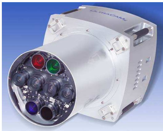
Figure 3.4: Sensor head of UltraCamX digital aerial camera system with 8 cones and five spectral bands (pan, RGB and NIR), adapted from Schneider and Gruber (2008).
