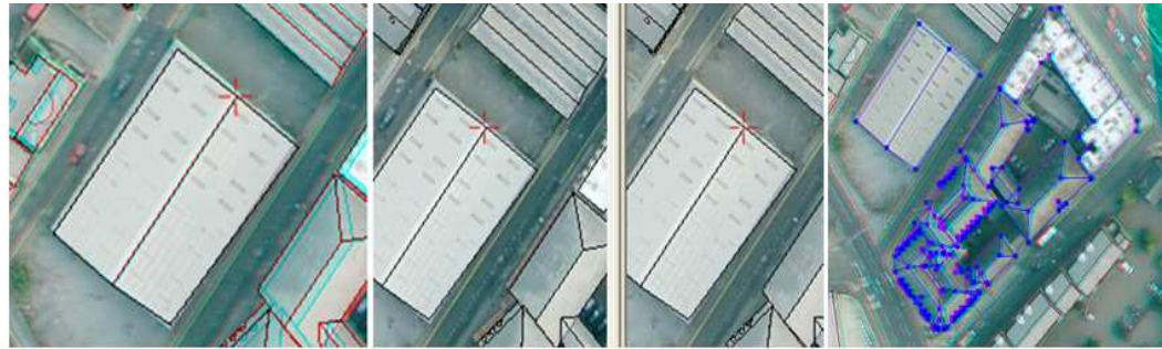
Figure 6.5: x-parallax has been adjusted for point of interest (left) so that the measuring mark on each image is placed on the corresponding point of left and right images (middle). Right image shows extracted polygons for several buildings in the Nottingham city centre.
