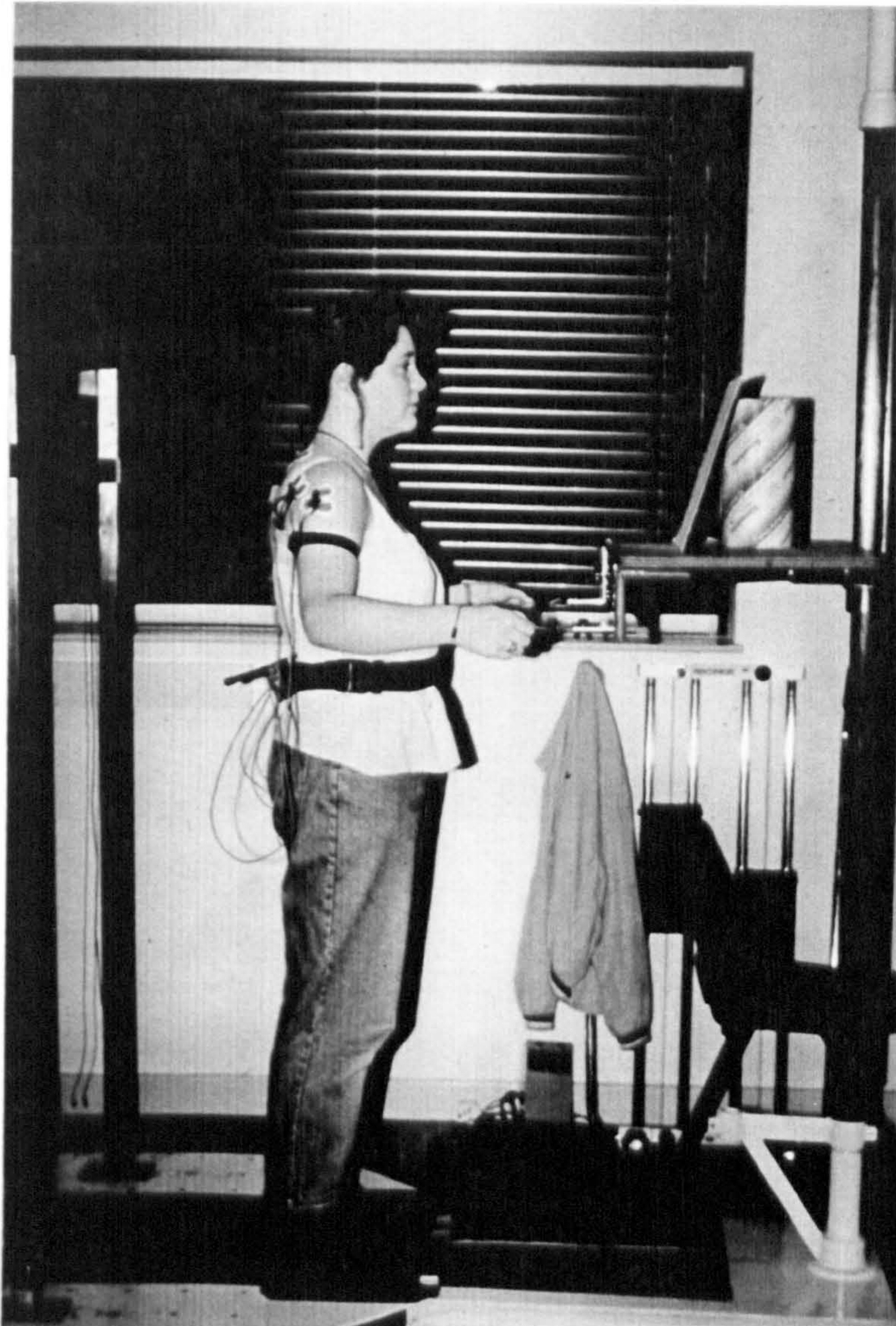
Figure 3.5 Full view of the experimental set-up used during the measurement of maximal endurance to arm abduction. The case illustrated was the holding at 30^{\circ} .
