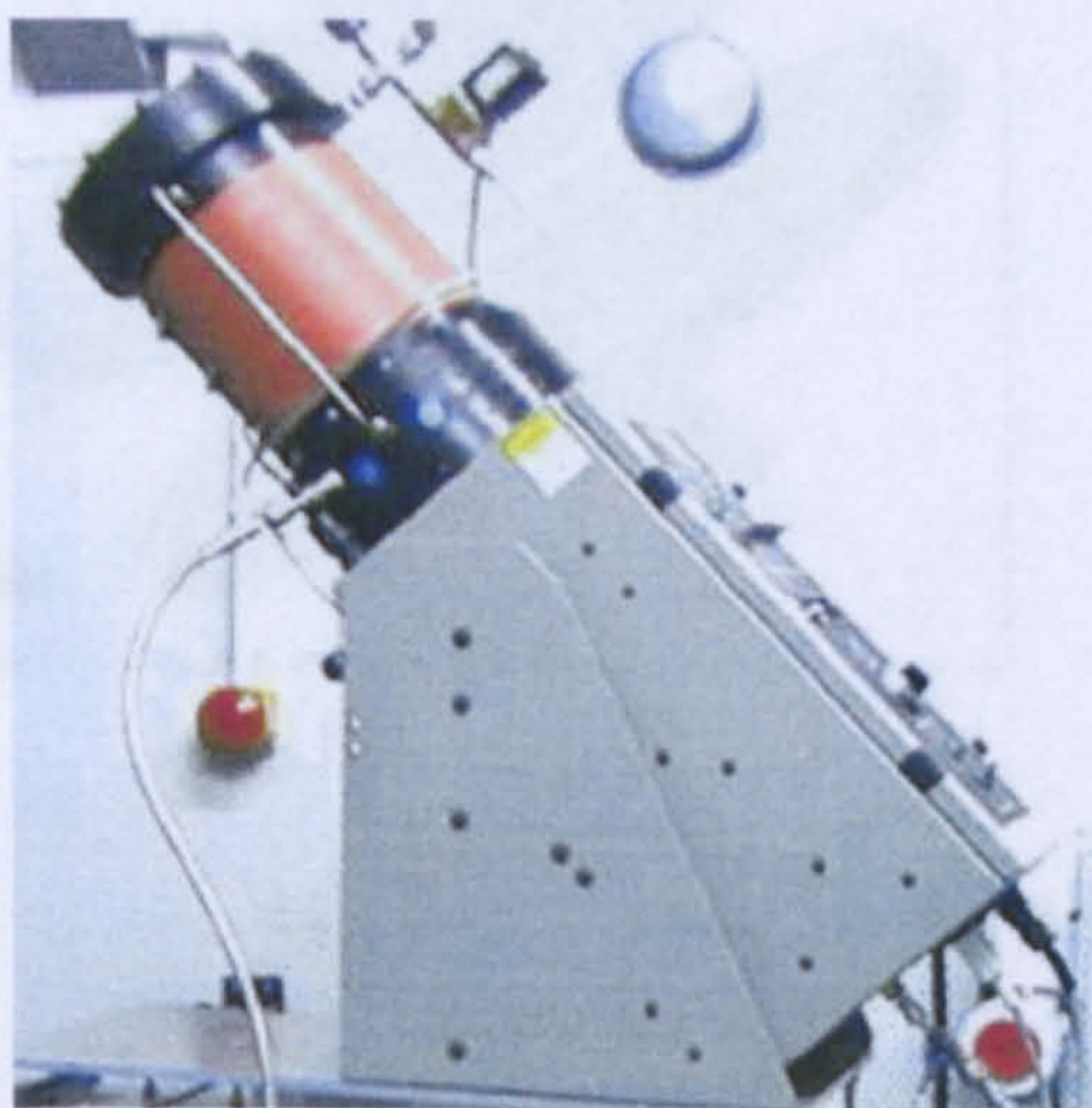
Figure 4.9: Praxair high-pressure powder feeder with the heating jacket.
