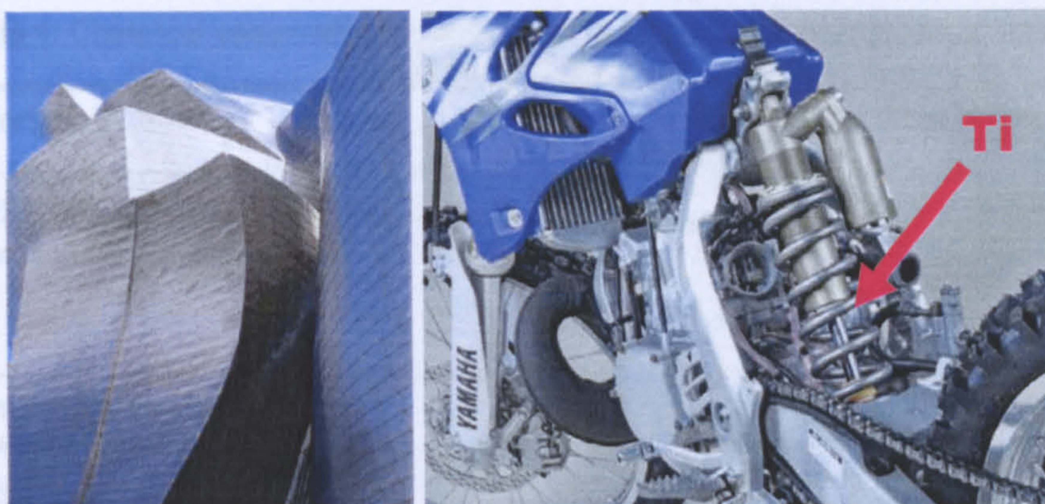
Figure 4.1: (right) Architectural application of Ti in the prospect of the Guggenheim Museum in Bilbao. (left) Monoshock coil spring in Ti alloy (TIMETAL LCB™) mounted on the 2006 Yamaha YZ250 MX bike; it is 30% lighter than an equivalent steel spring [2].
