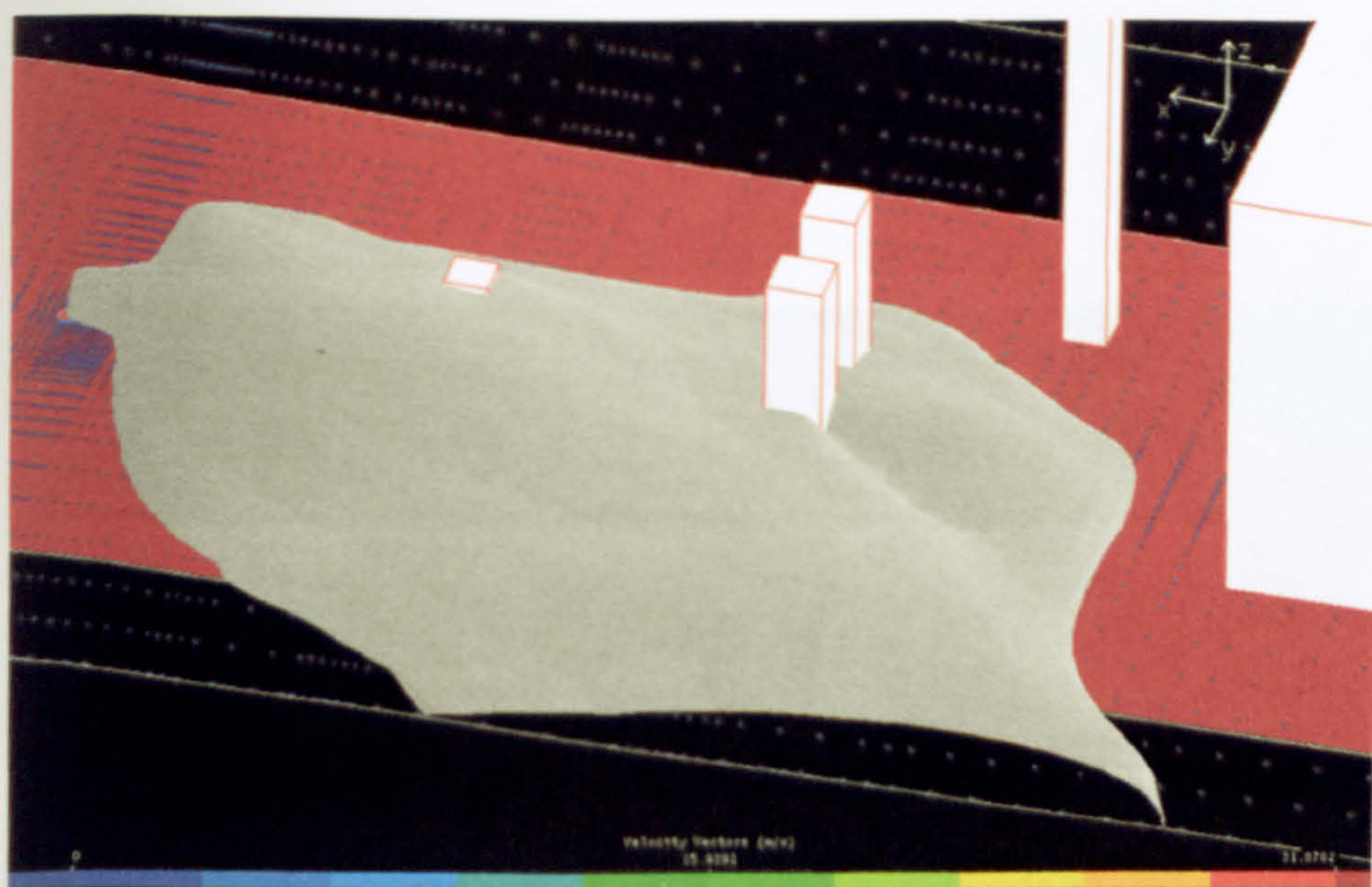
Figure 6.12 - Dispersion of 2,000 ppm CO 2 surface within a hypothetical plant environment and for the conditions described. The purple ground is the surface roughness z_0 = 1.5 m, used in order to consider small obstacles.
