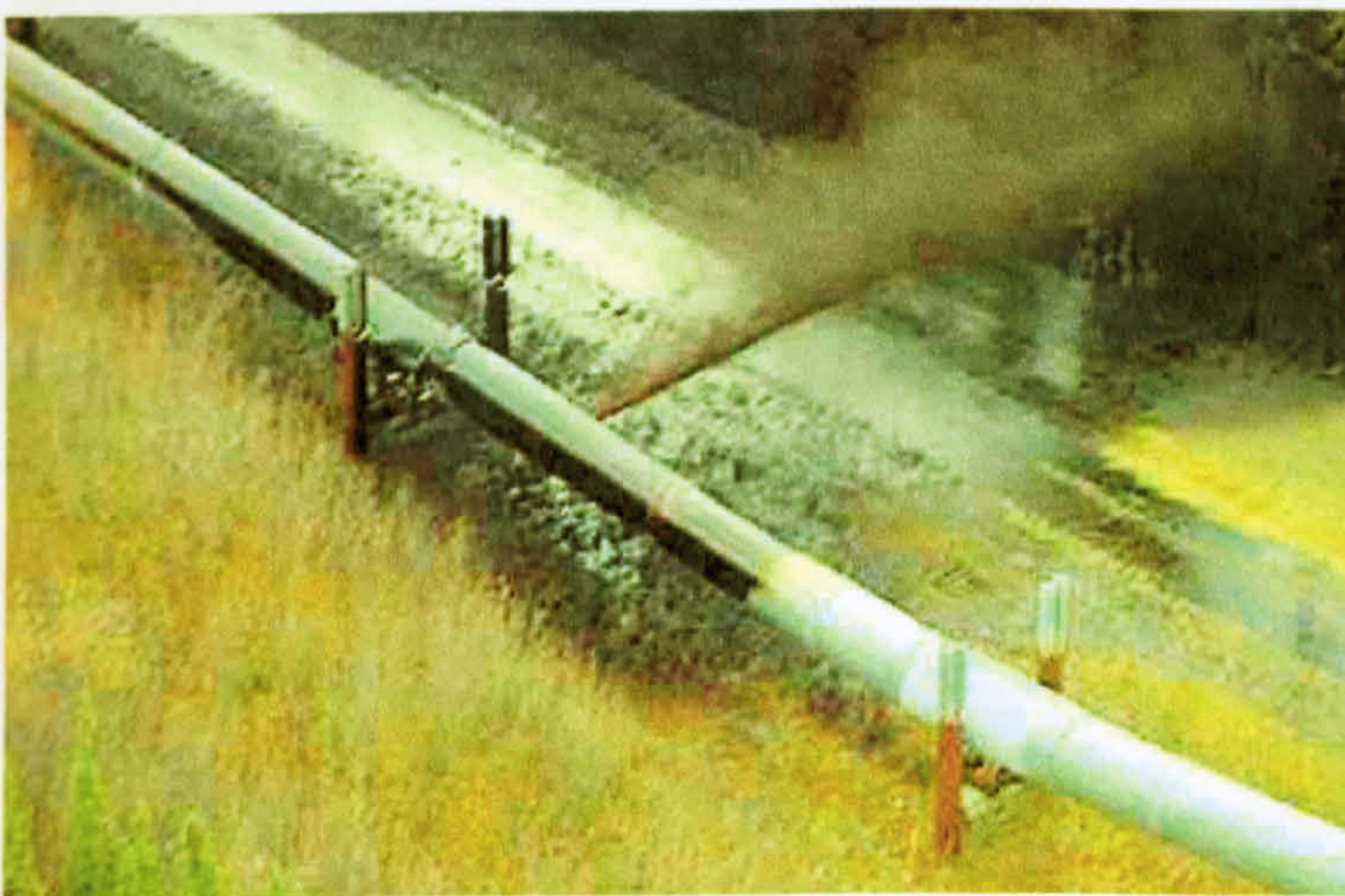
Figure 6.1 – A jet-released leakage from a high-pressure gas pipeline (Townes et al., 2004).
