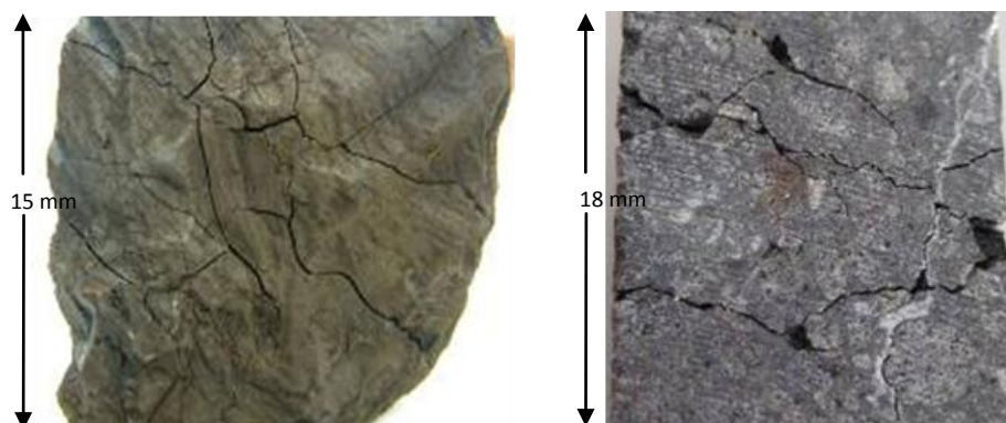
Figure 4.23 (Left) A Kimberlite II ore sample treated at 22 kW for 10 s (Right) A Kimberlite I sample treated at 18 kW for 7.5 s
