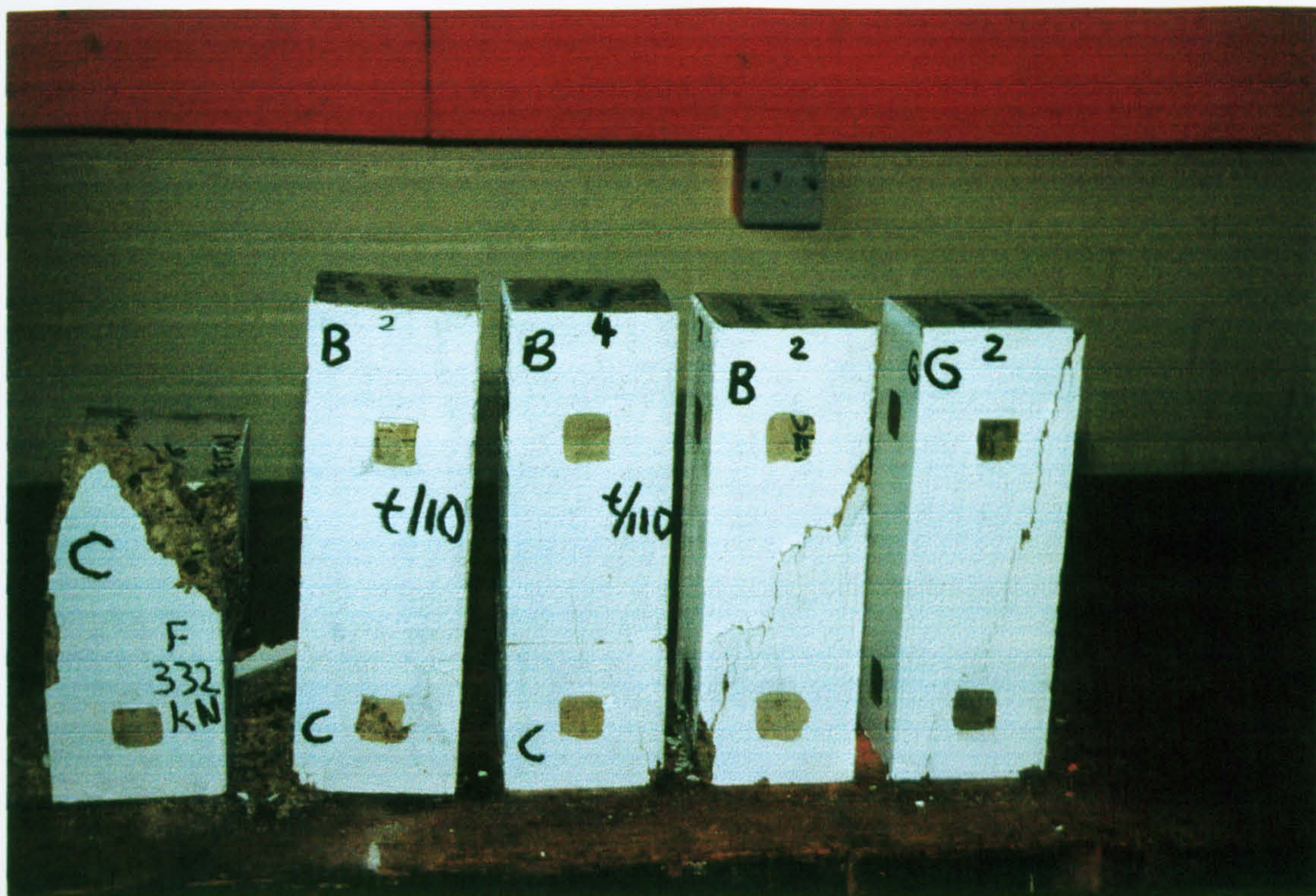
Plate 9.5(b) : Failure regions of test series 5 (the most damaged faces)
