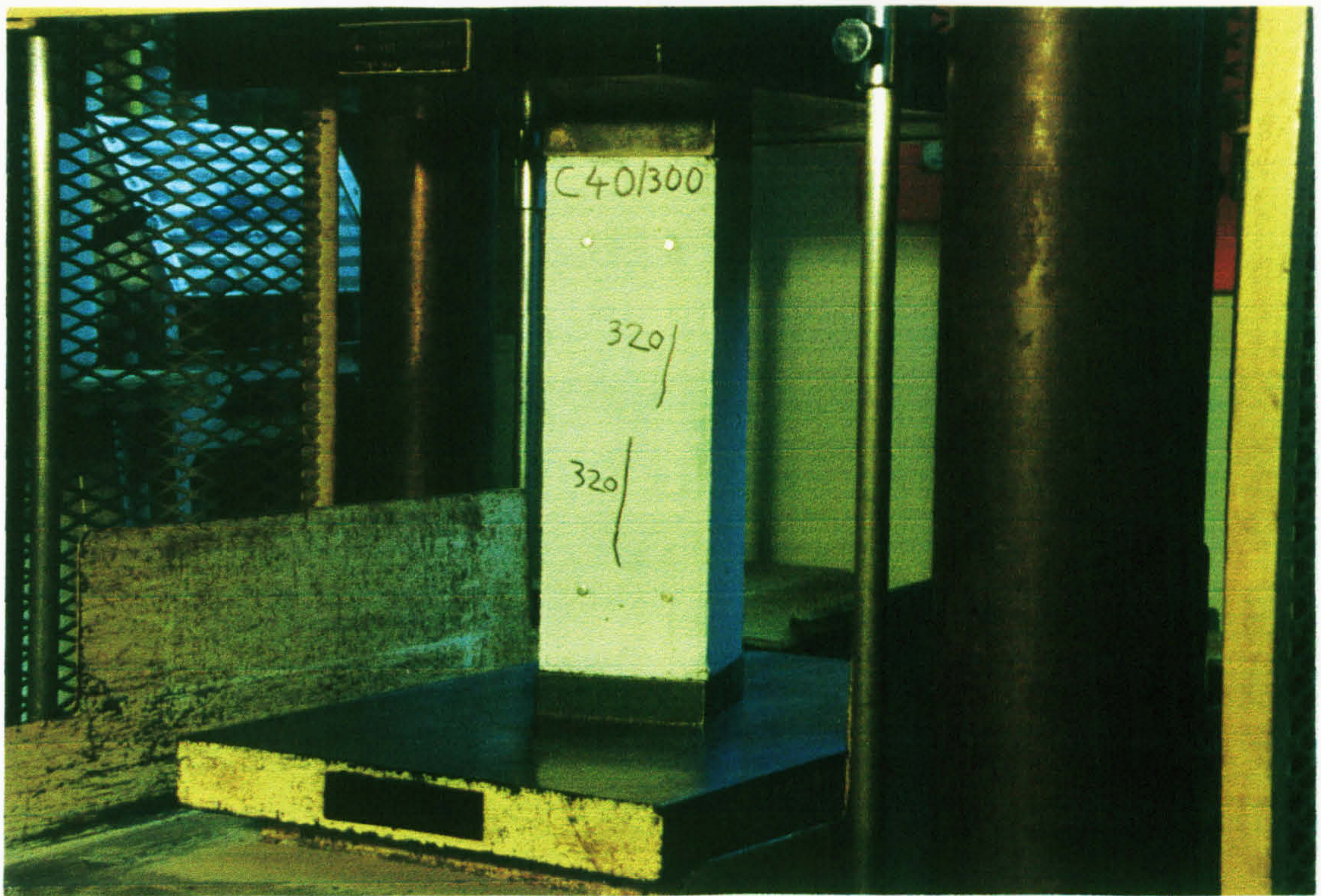
Plate 8.1: General arrangement of compression specimens type A for test series 1, 2 and 3
