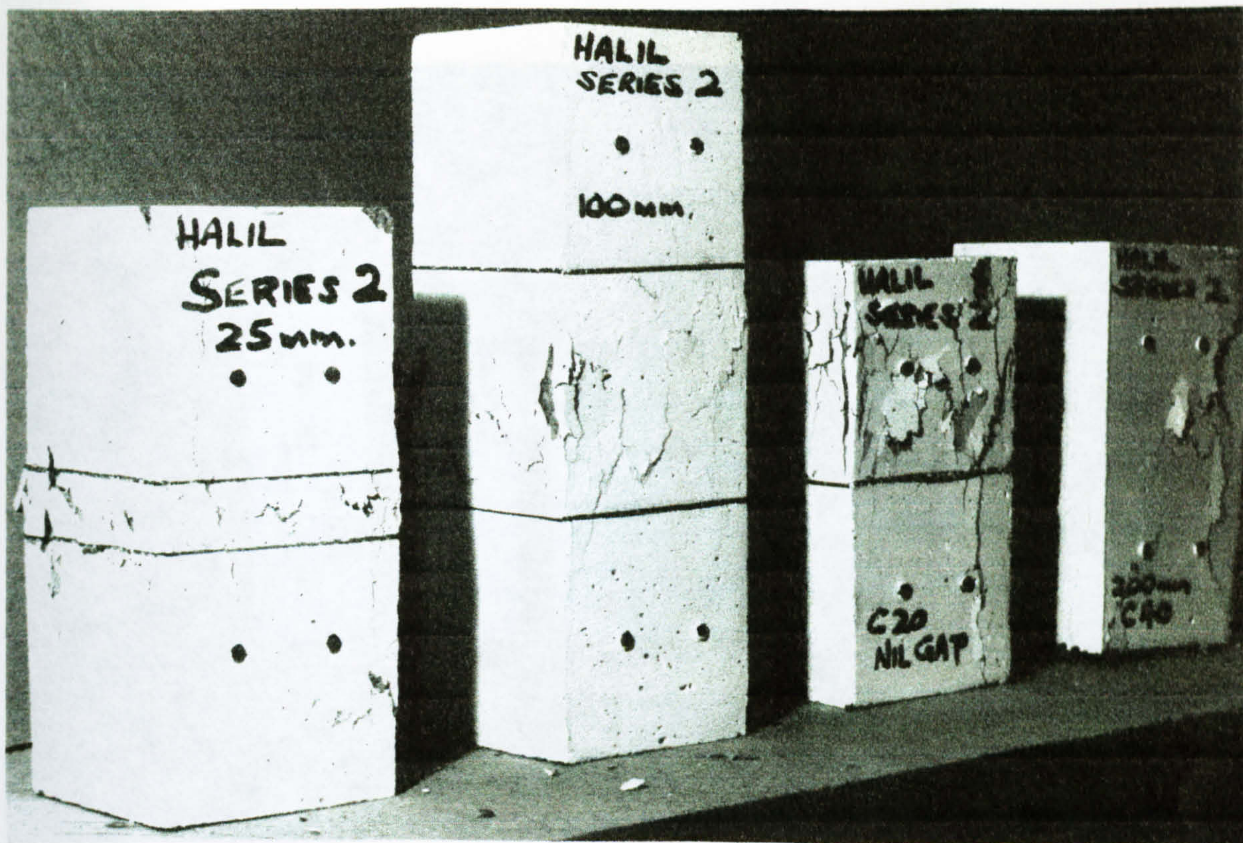
Plate 9.2 : Failure regions of test series 2
