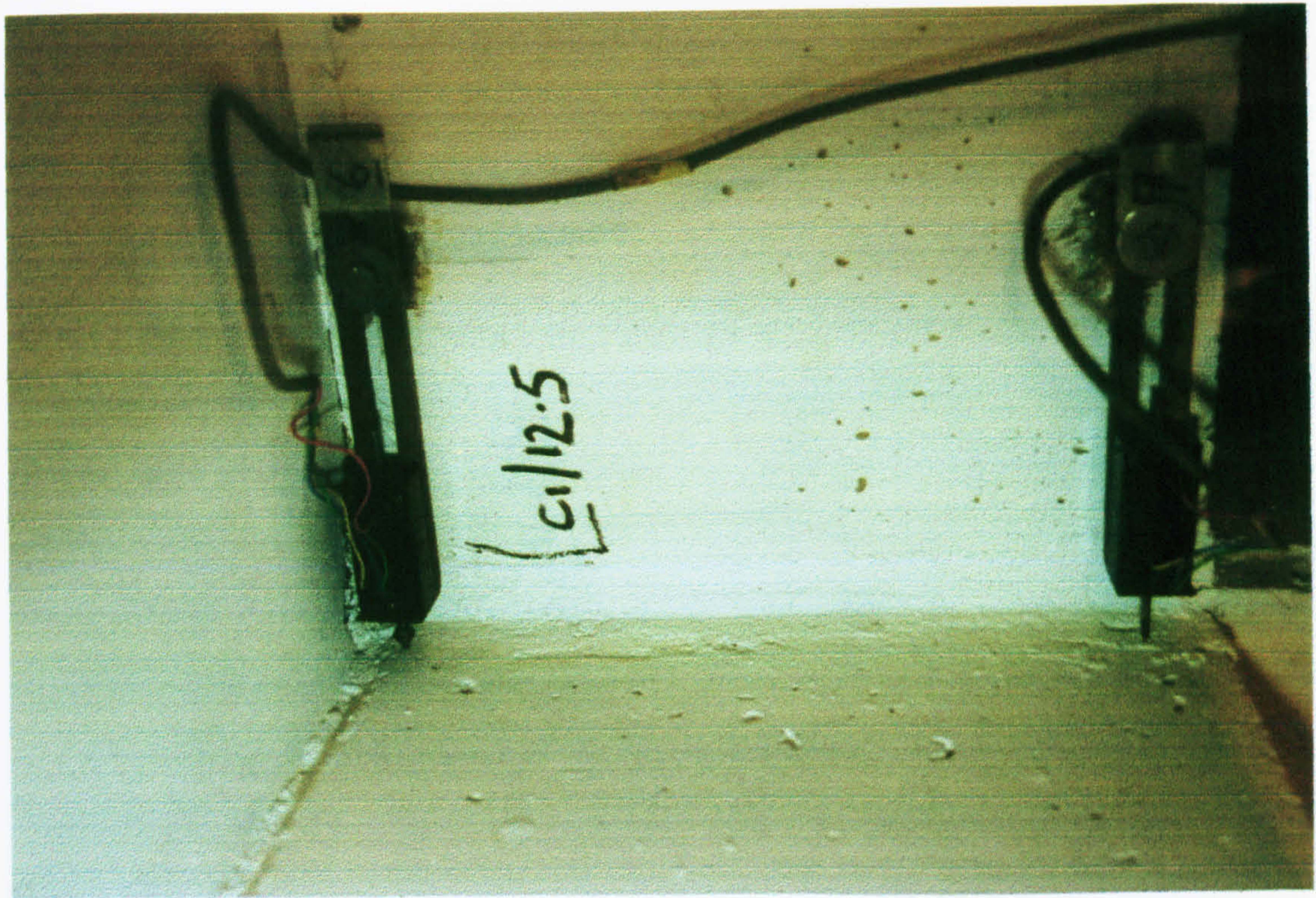
Plate 6.29: First cracks opening at joint-column boundary from East and West in TB2
