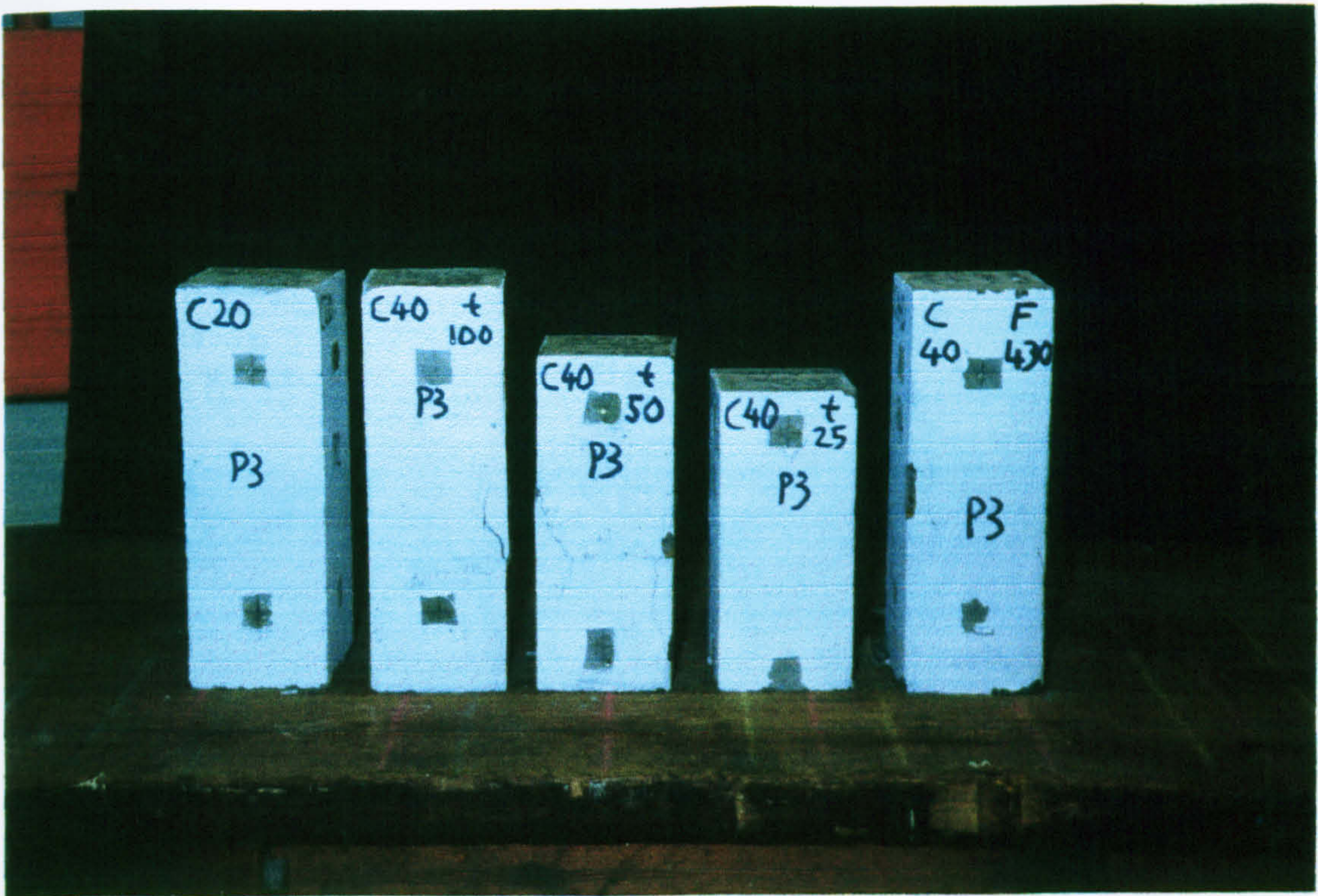
Plate 9.4(b) : Failure regions of test series 4 (back face)
