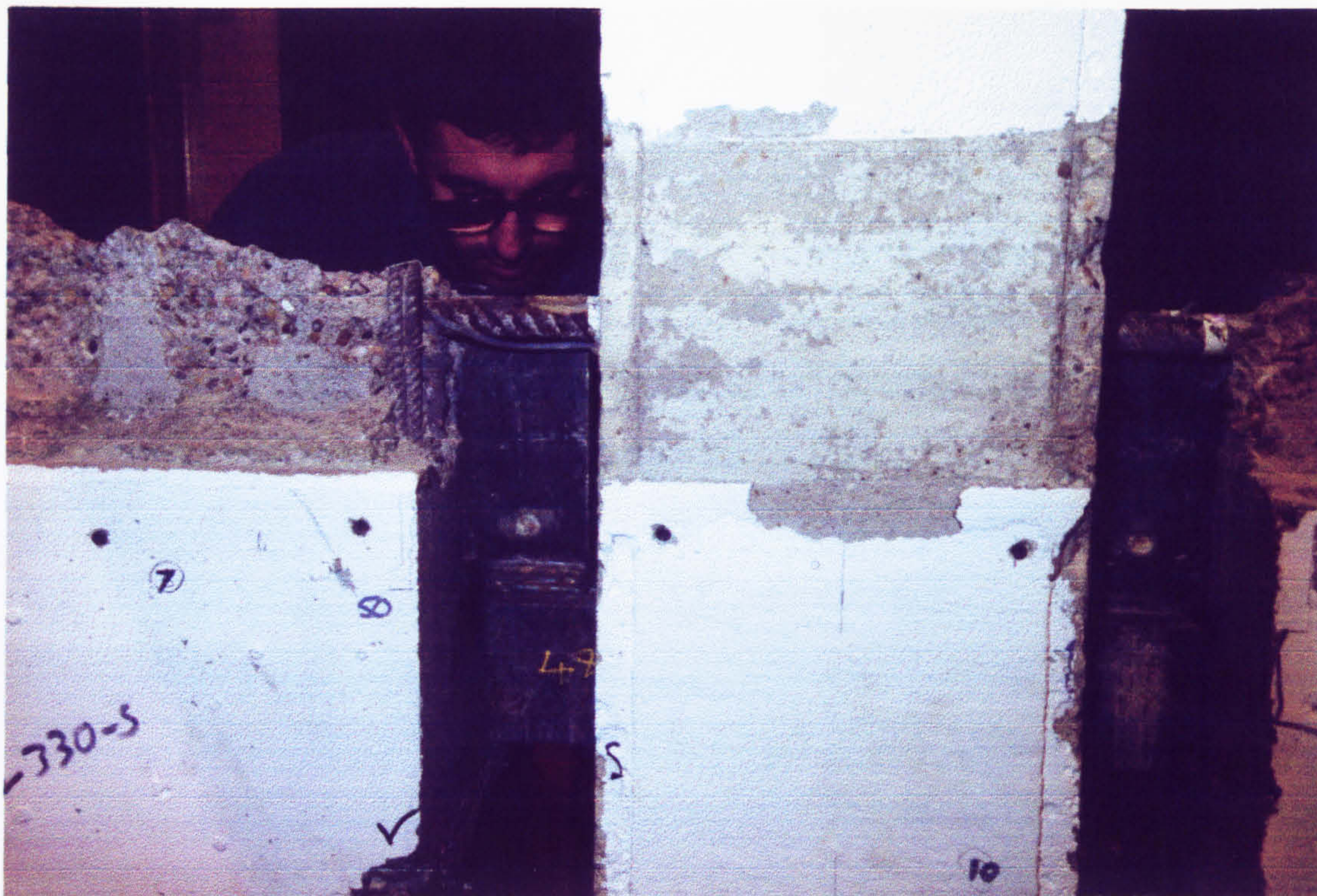
Plate 6.9: Inspecting the weld after re-welding for TW1(C)
