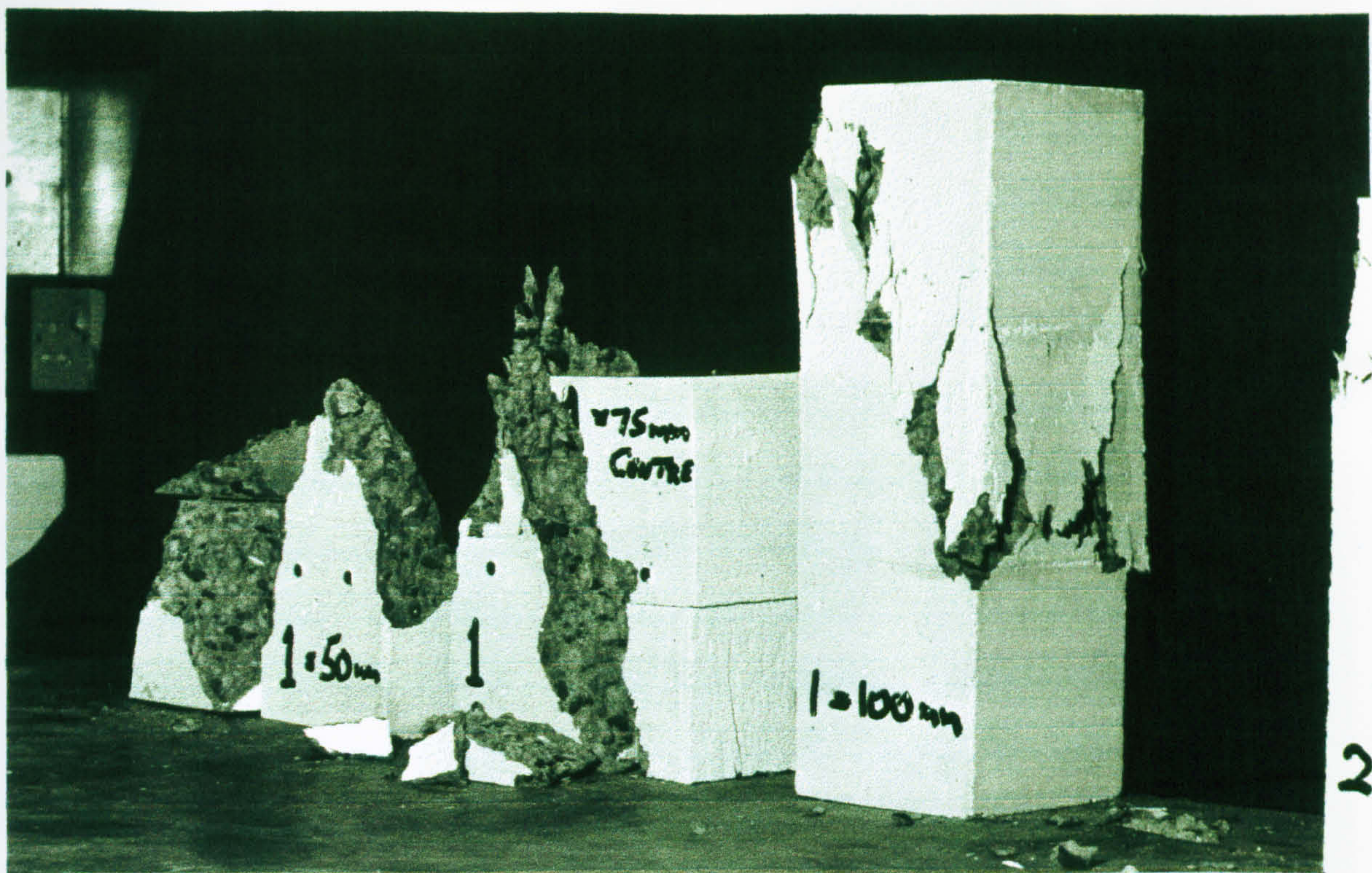
Plate 9.1(a) : Failure regions of test series 1 for mix 1 specimens
