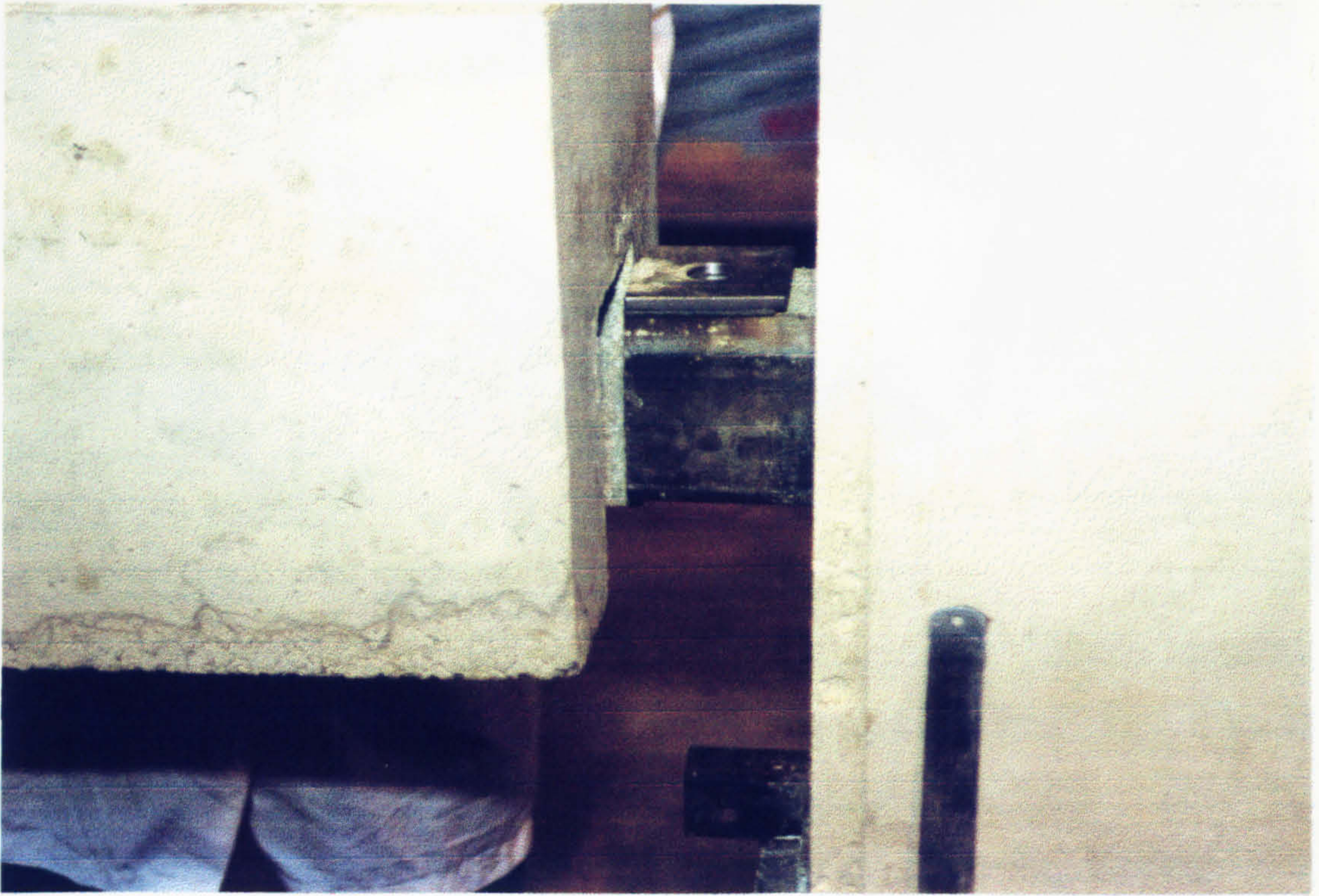
Plate 5.17: Construction of bolted billet connection in test series 3
