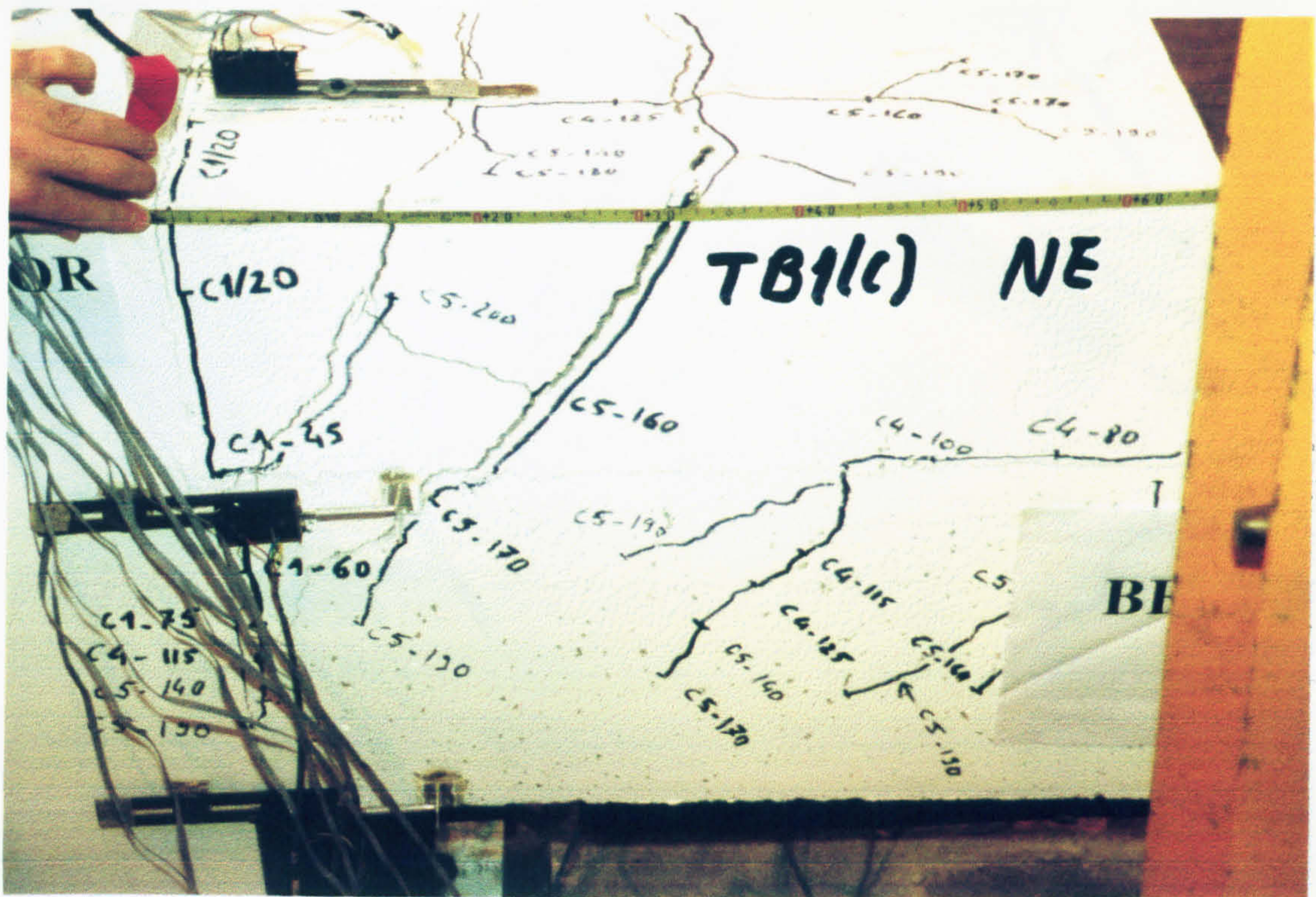
Plate 6.23: Failure regions in beam 1 from East in TB1(C)
