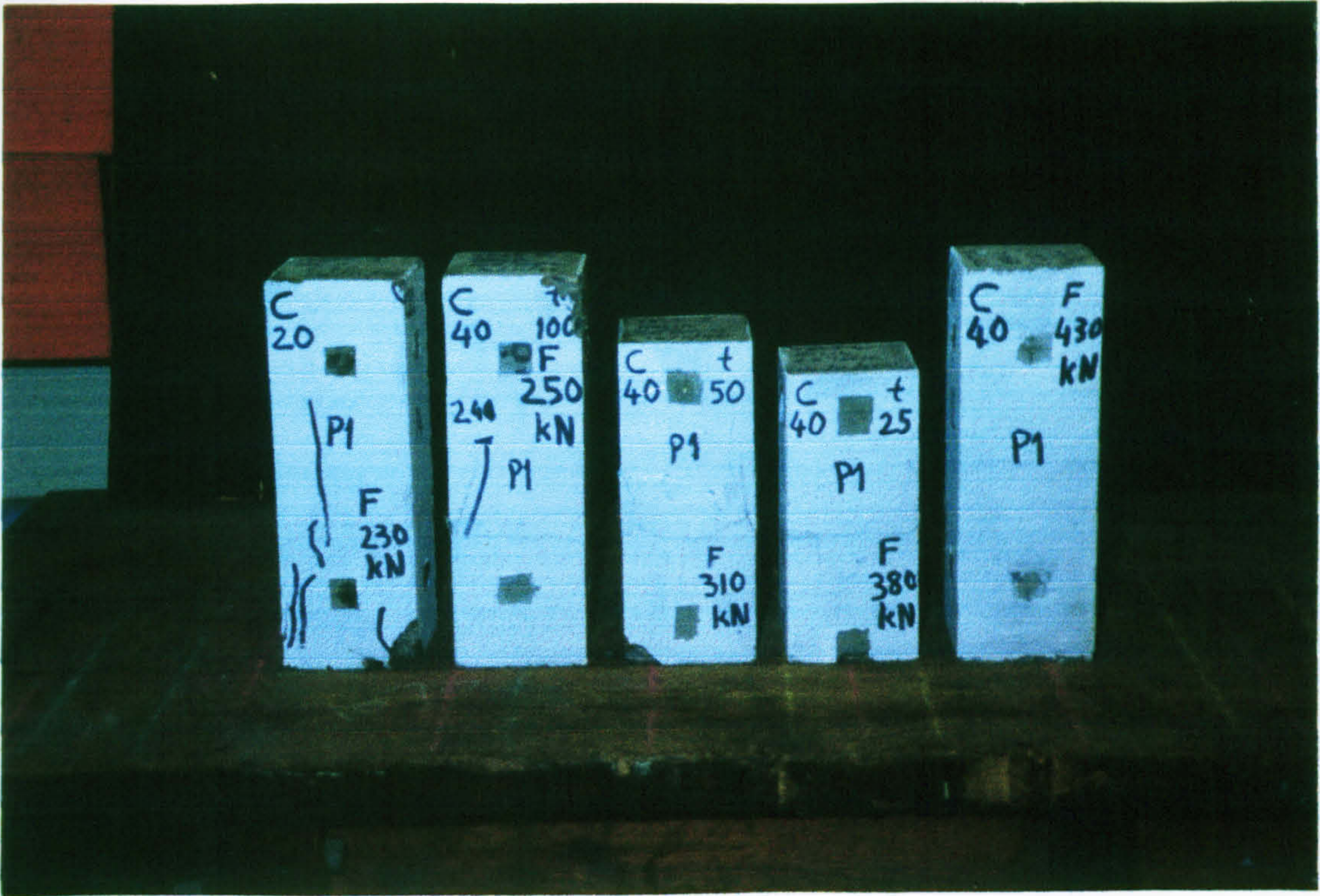
Plate 6.4(a): Failure regions of test series 4 (front face)
