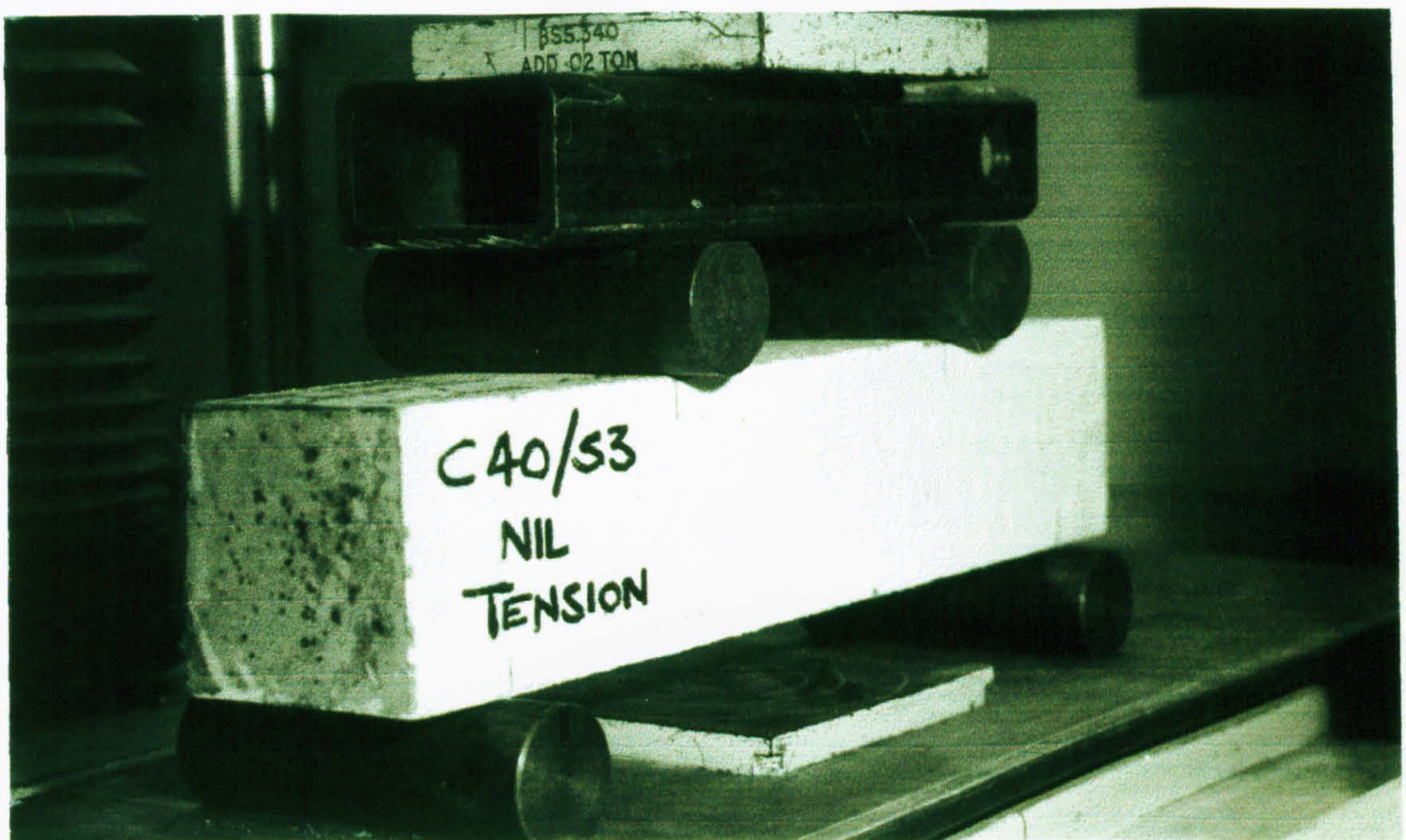
Plate 8.4: General arrangement of flexural specimens type B for test series 6
