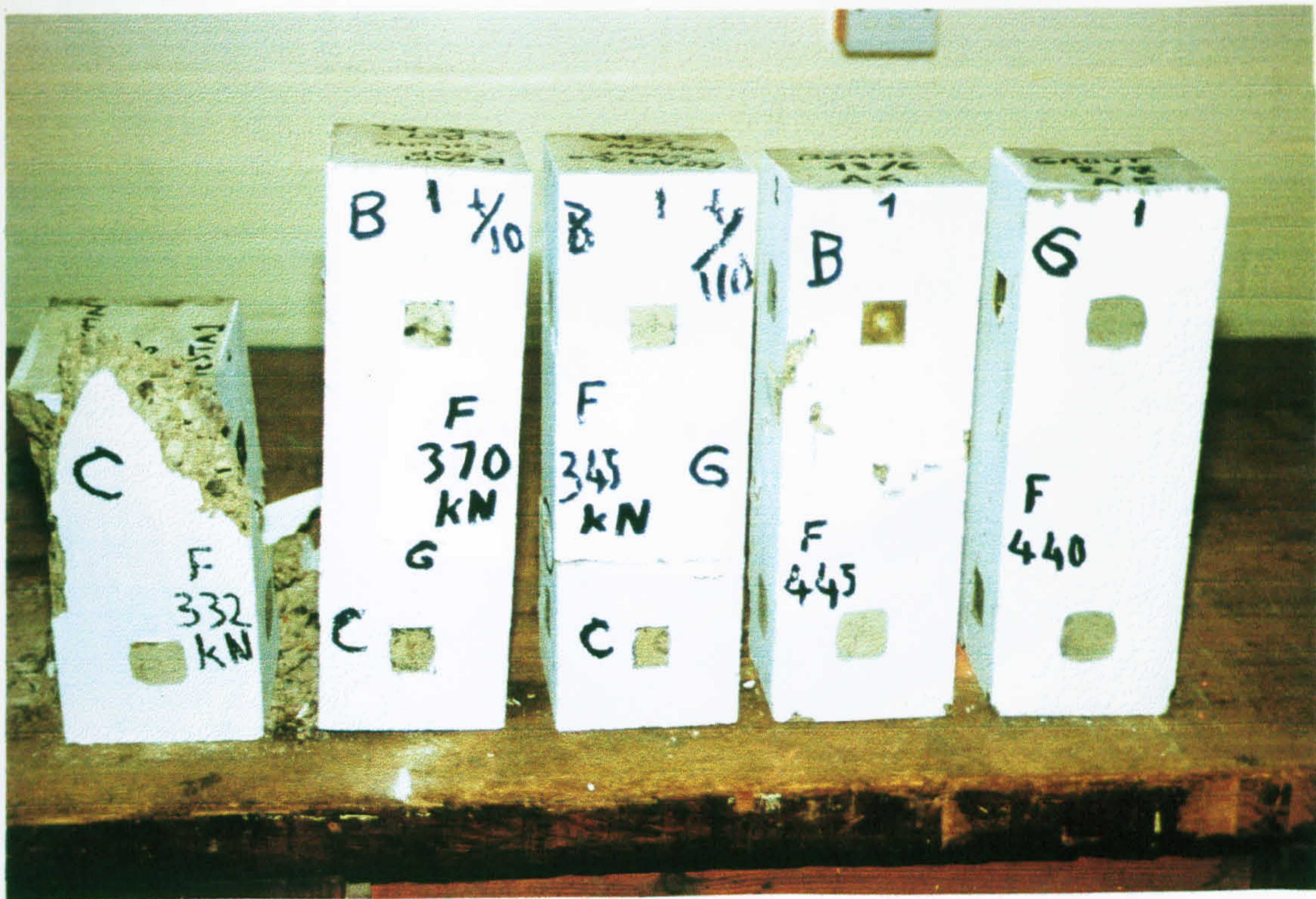
Plate 9.5(a) : Failure regions of test series 5 (front face)
