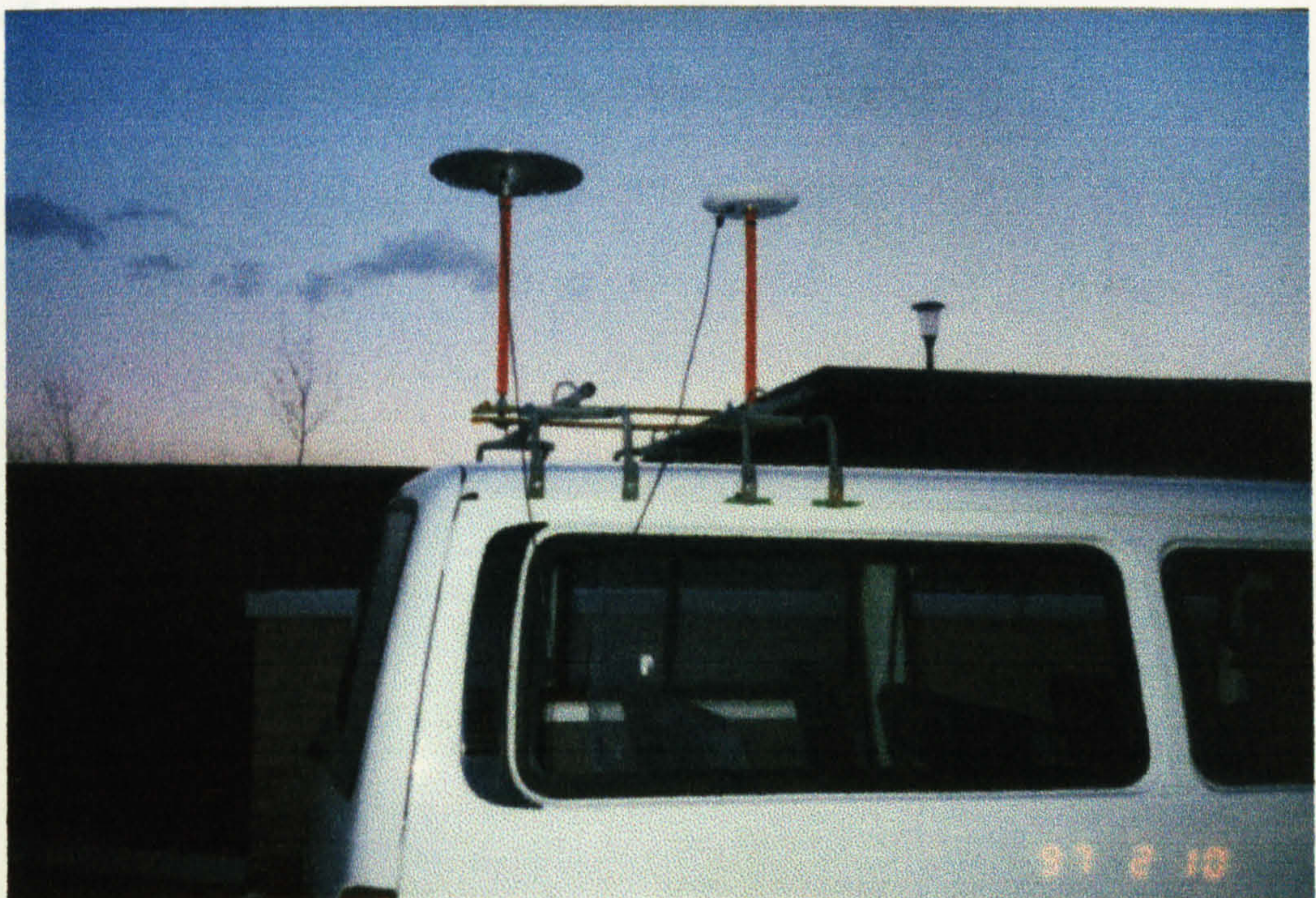
Plate 6.1 Roof Rack, Antenna and Cabling Set-Up
