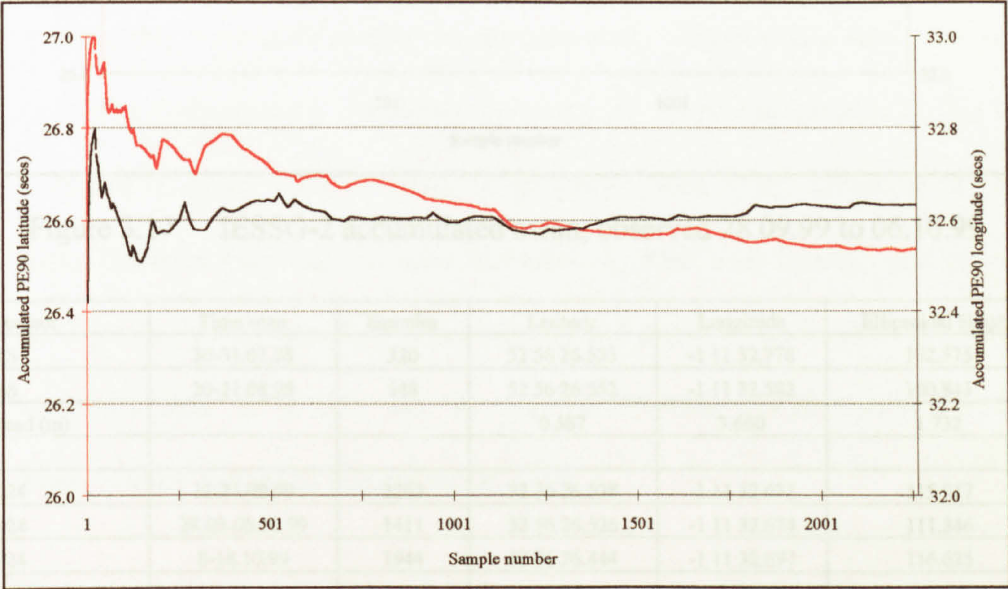
Figure 3.15 IESSG-2 accumulated mean, observed 13.09.99 to 21.09.99
