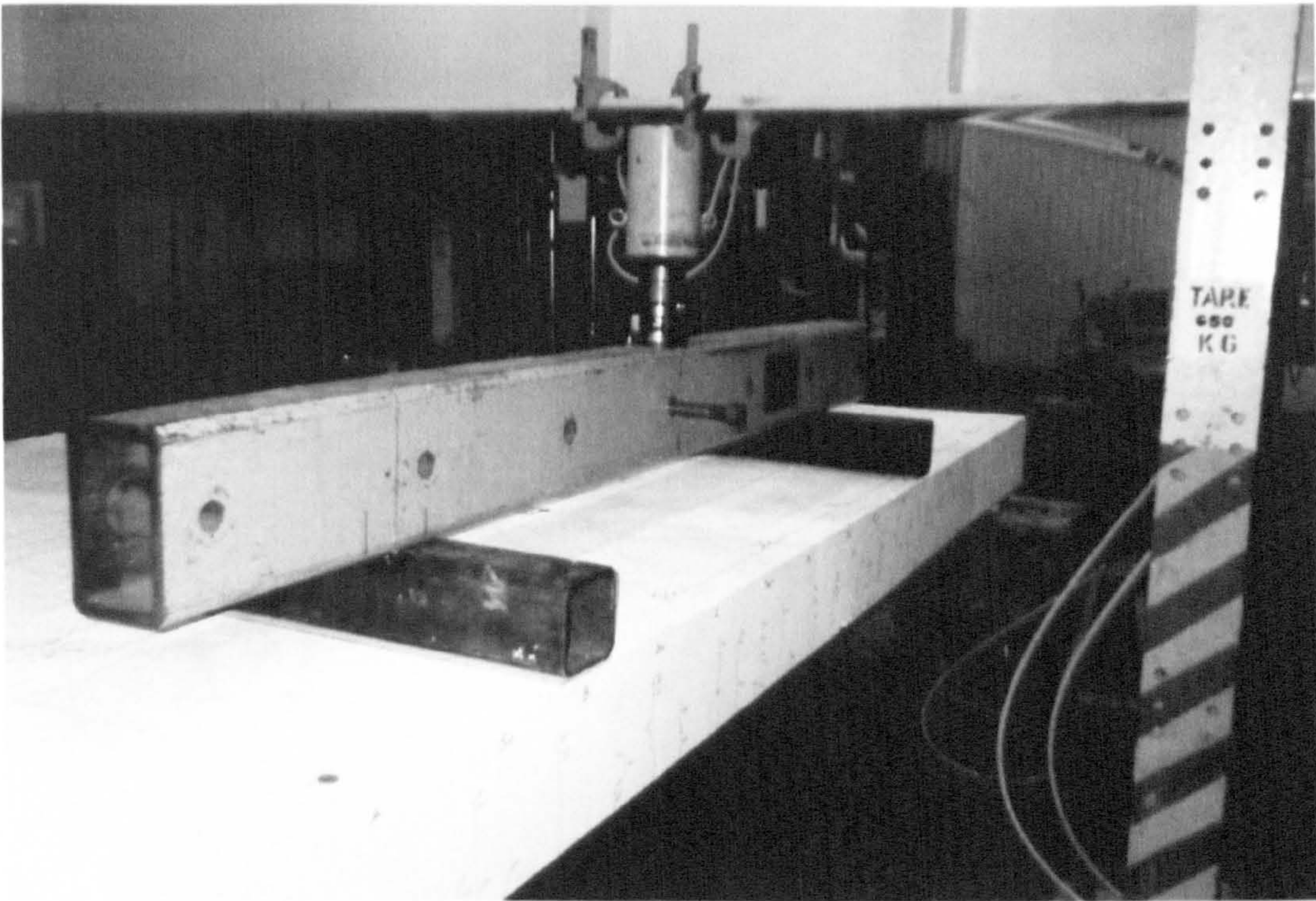
Plate 4-15: Deck 5 loading and cracking
