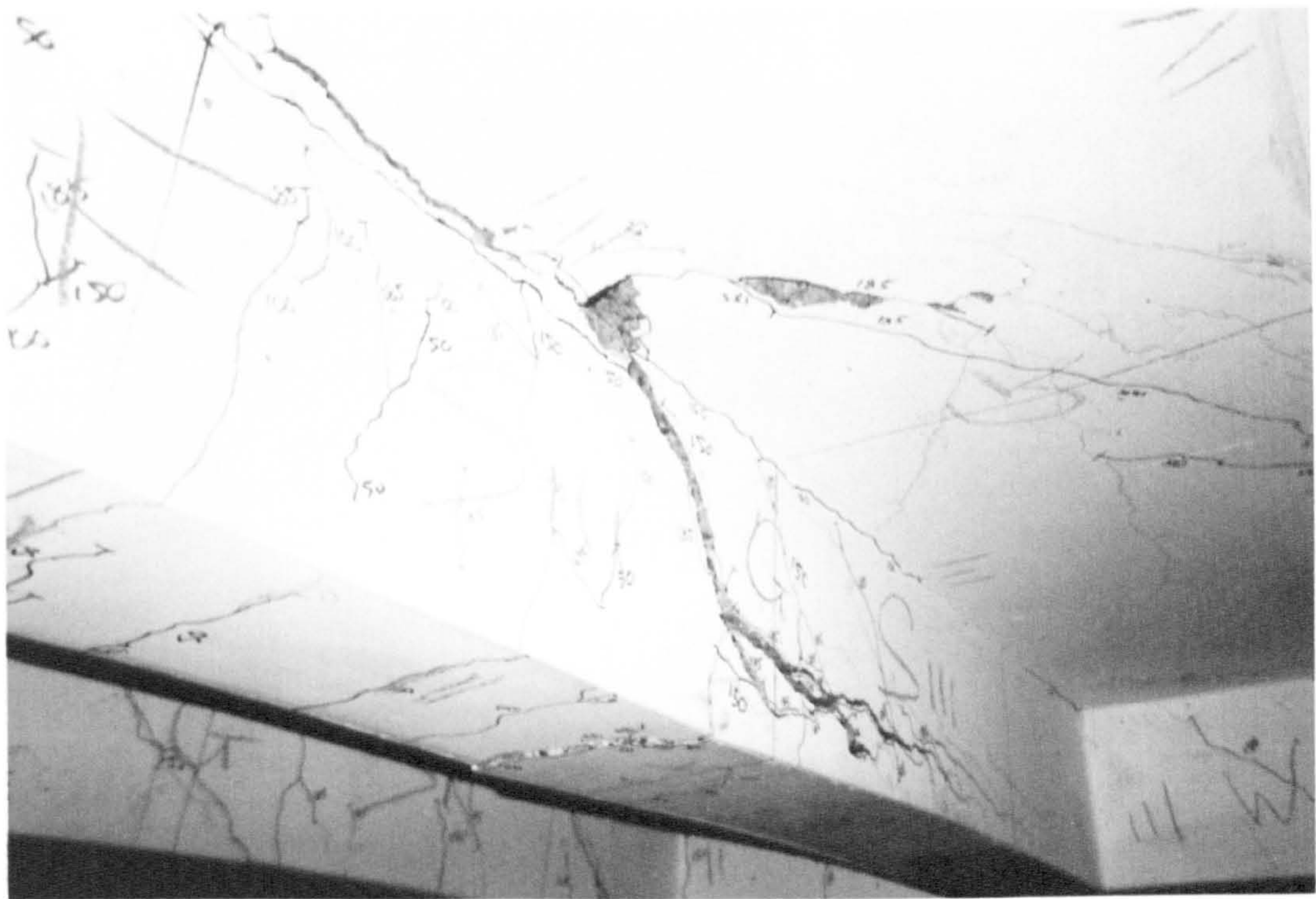
Plate 4-5: Deck 6 combined shear and bending failure in beam iii
