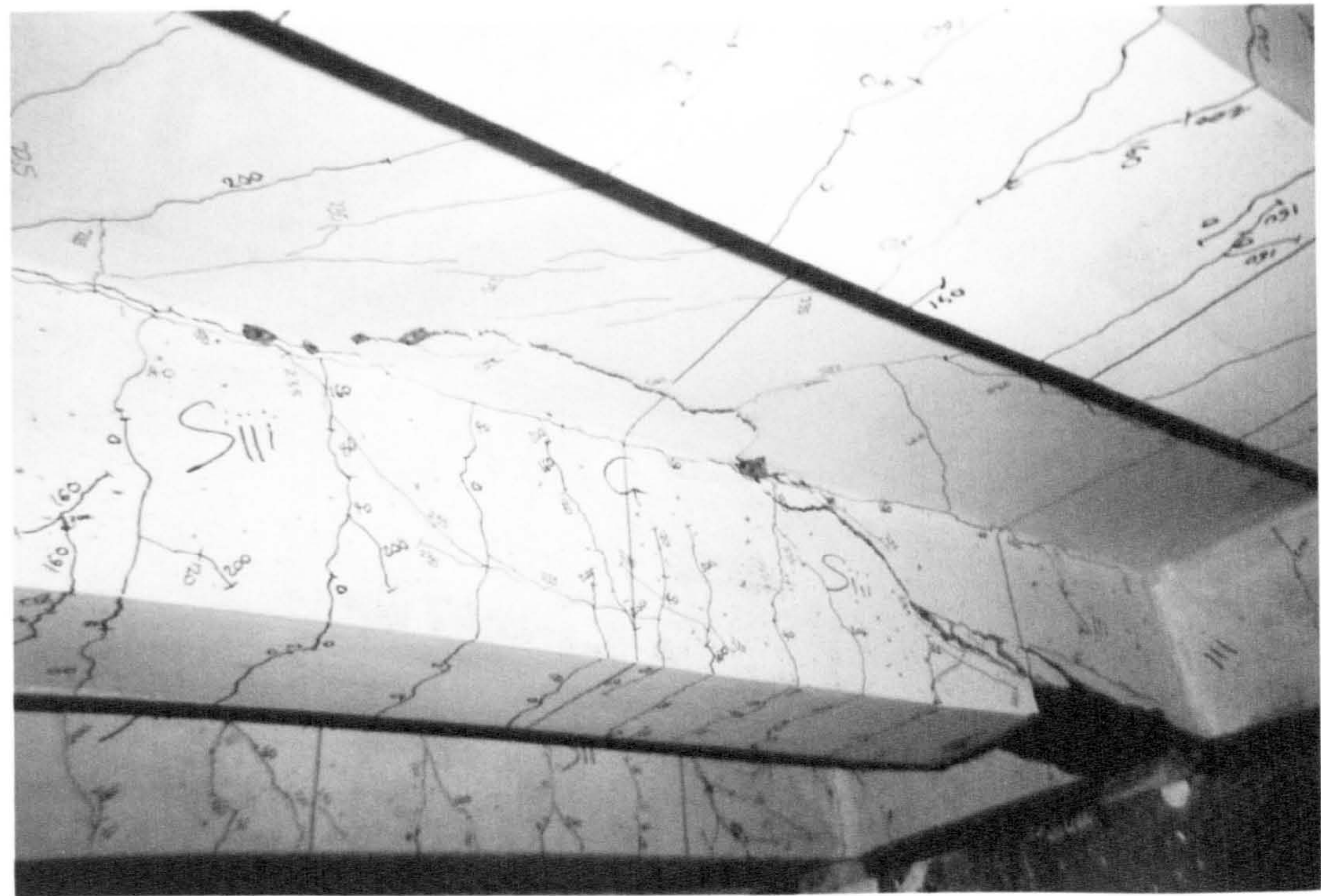
Plate 4-6: Deck 7 combined shear and bending failure in beam iii
