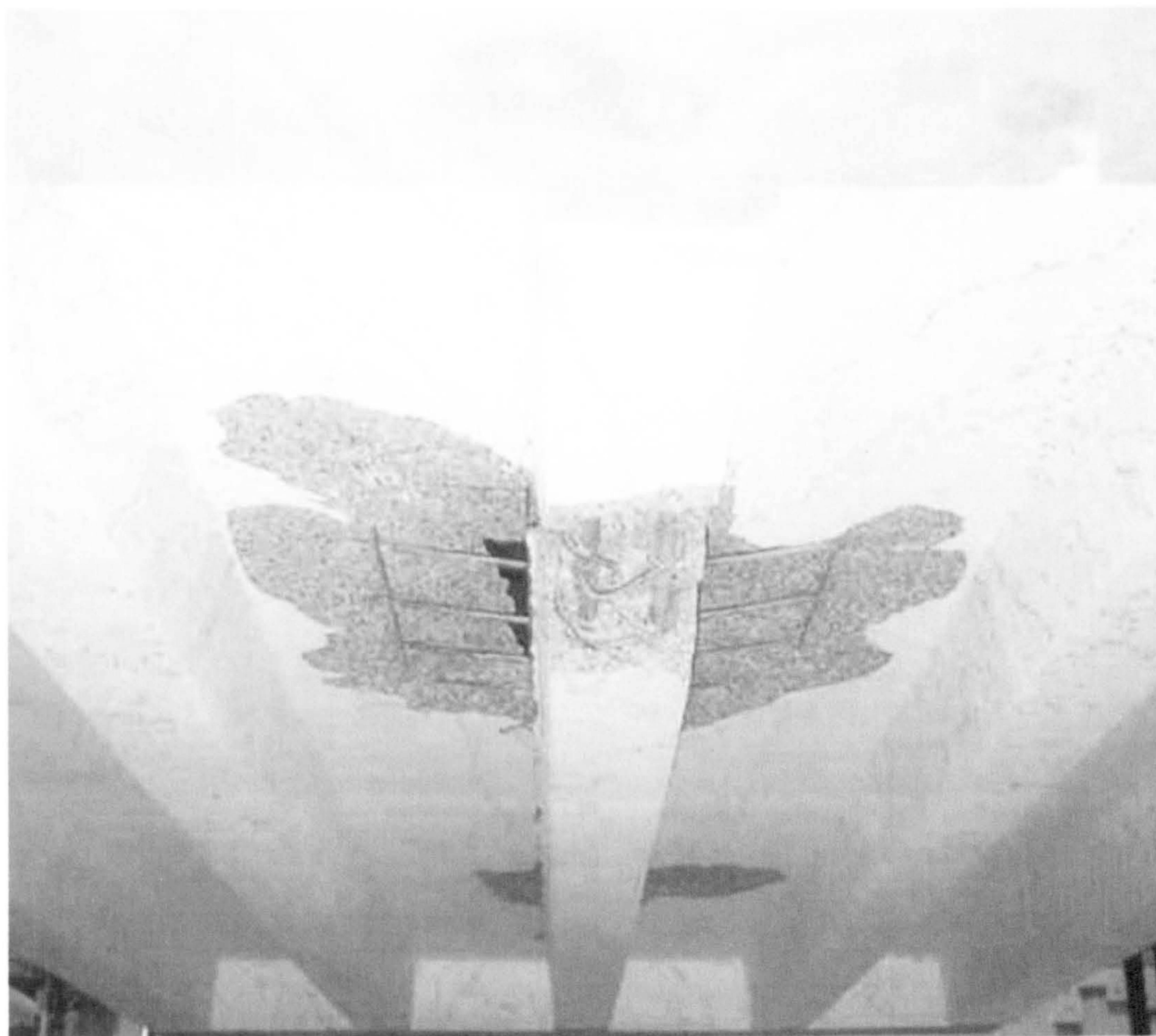
Plate 4-3: Deck 2 showing damage to slab and beam at failure
