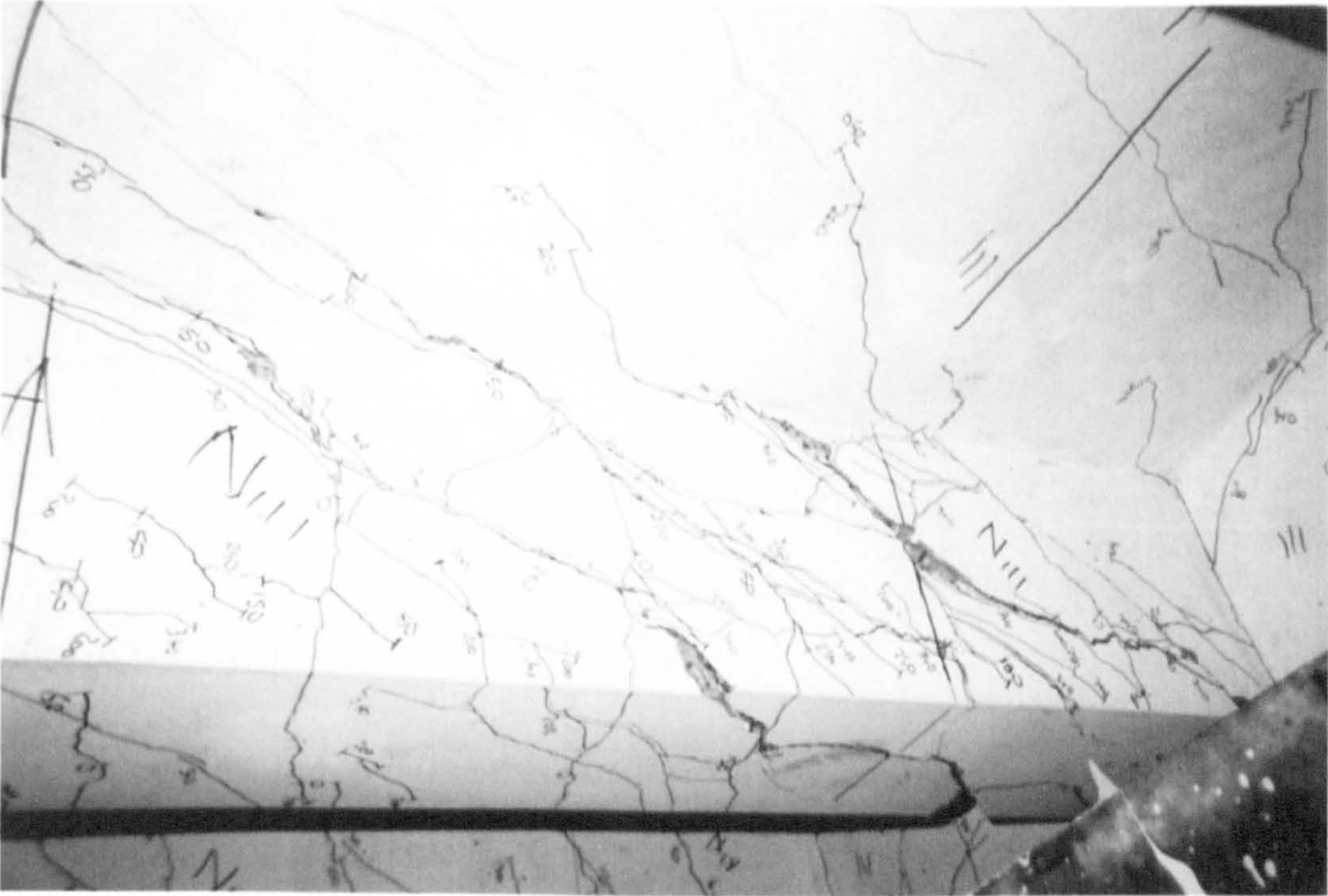
Plate 4-11: Deck 10 torsion cracking in beam iii
