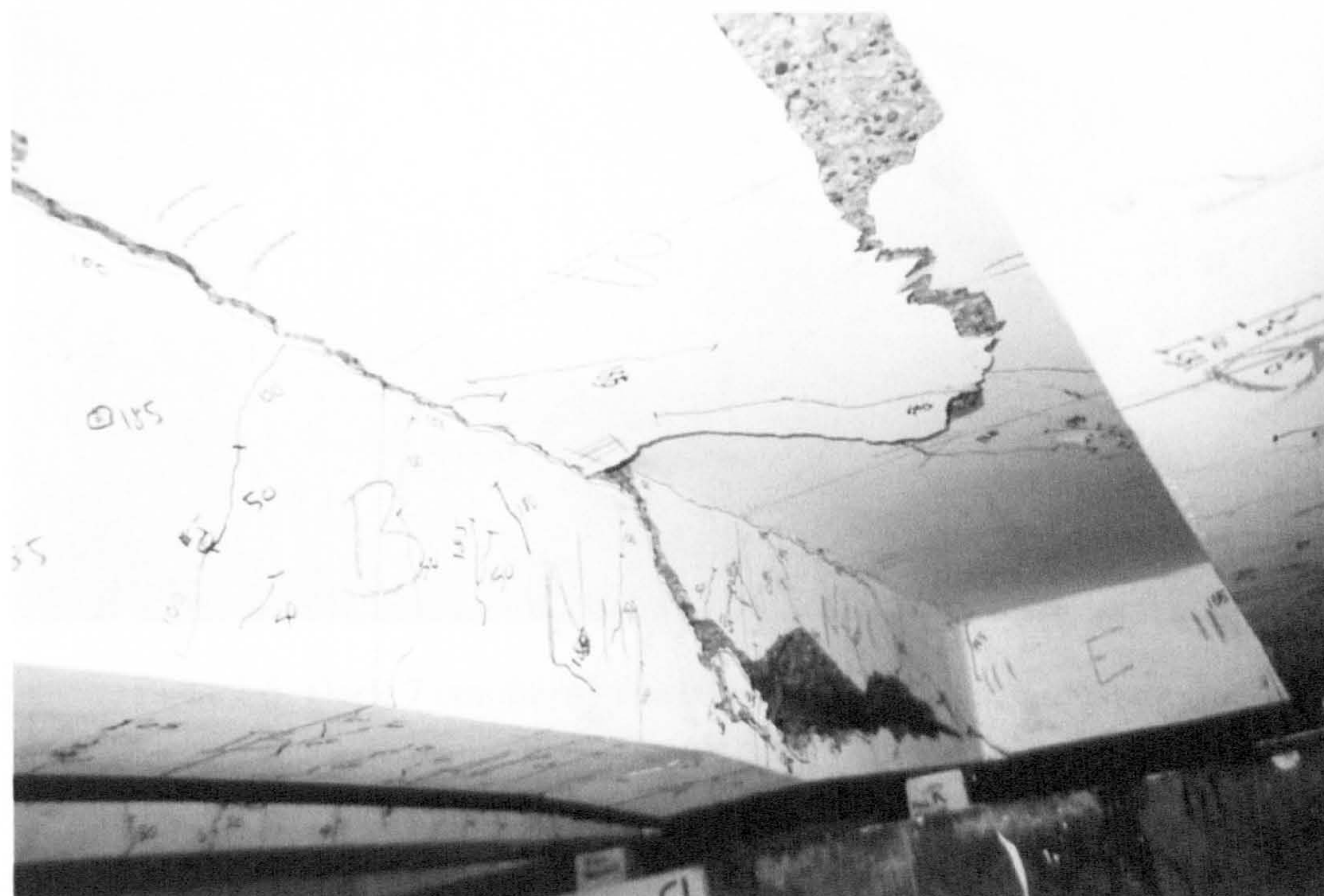
Plate 4-4: Deck 6 combined shear and bending failure in beam iii
