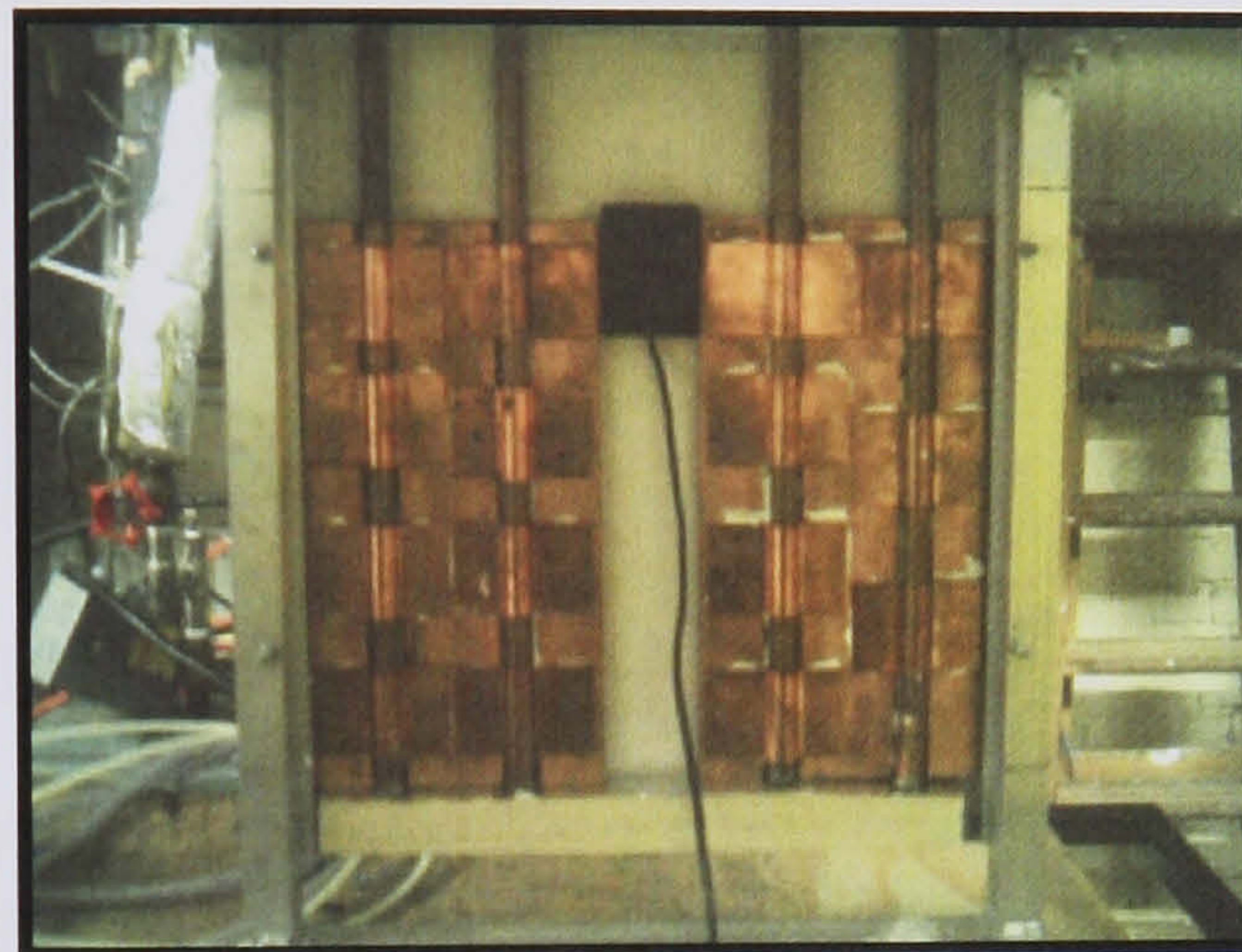
Figure 6.19 Back of PV with two copper plates incorporating four heat pipes
