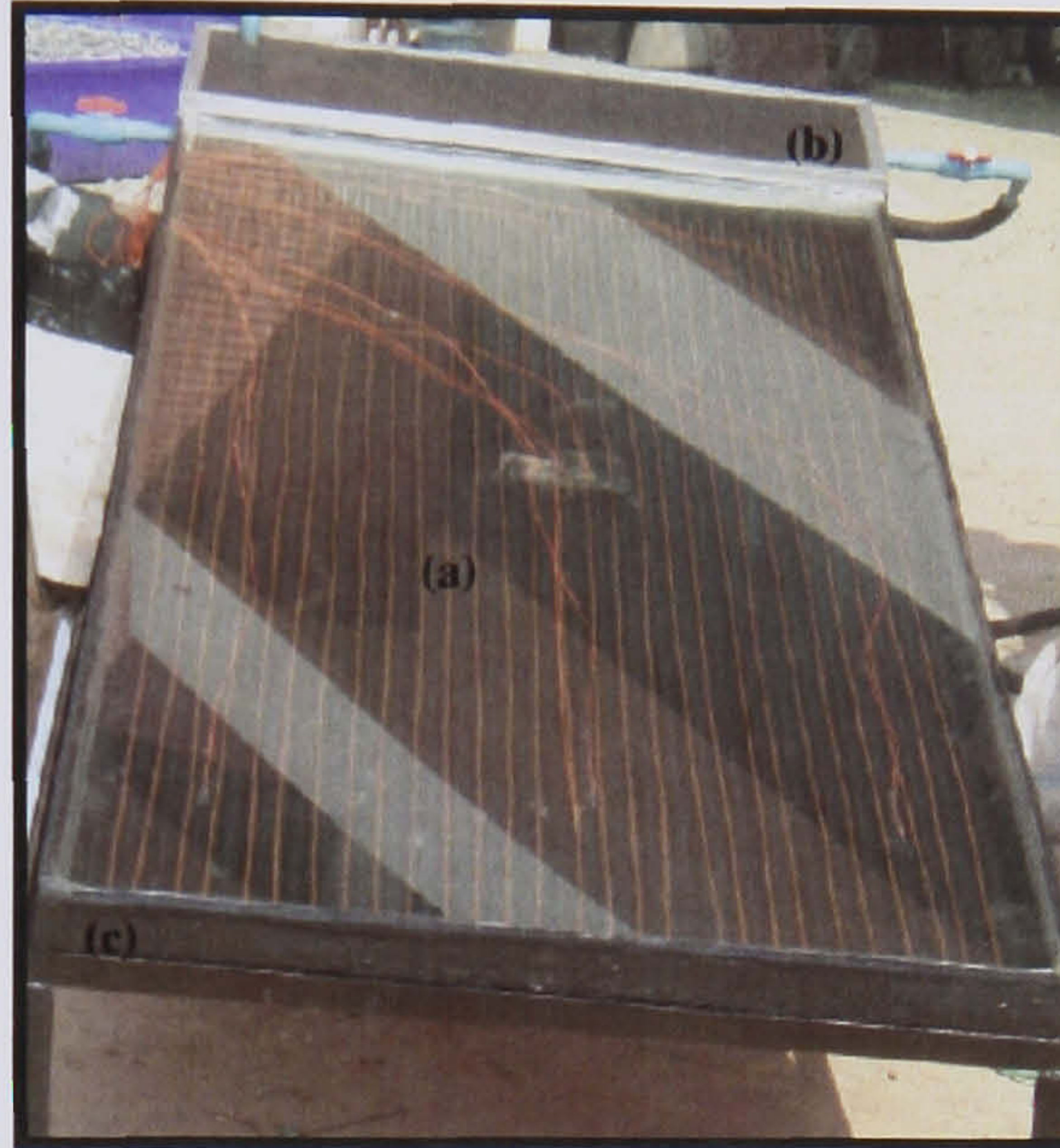
Figure 2.59 The experimental assembly: (a) CEOHP flat plate solar collector; (b) condenser water tank; (c) wooden frame. (Rittidech 2007)
