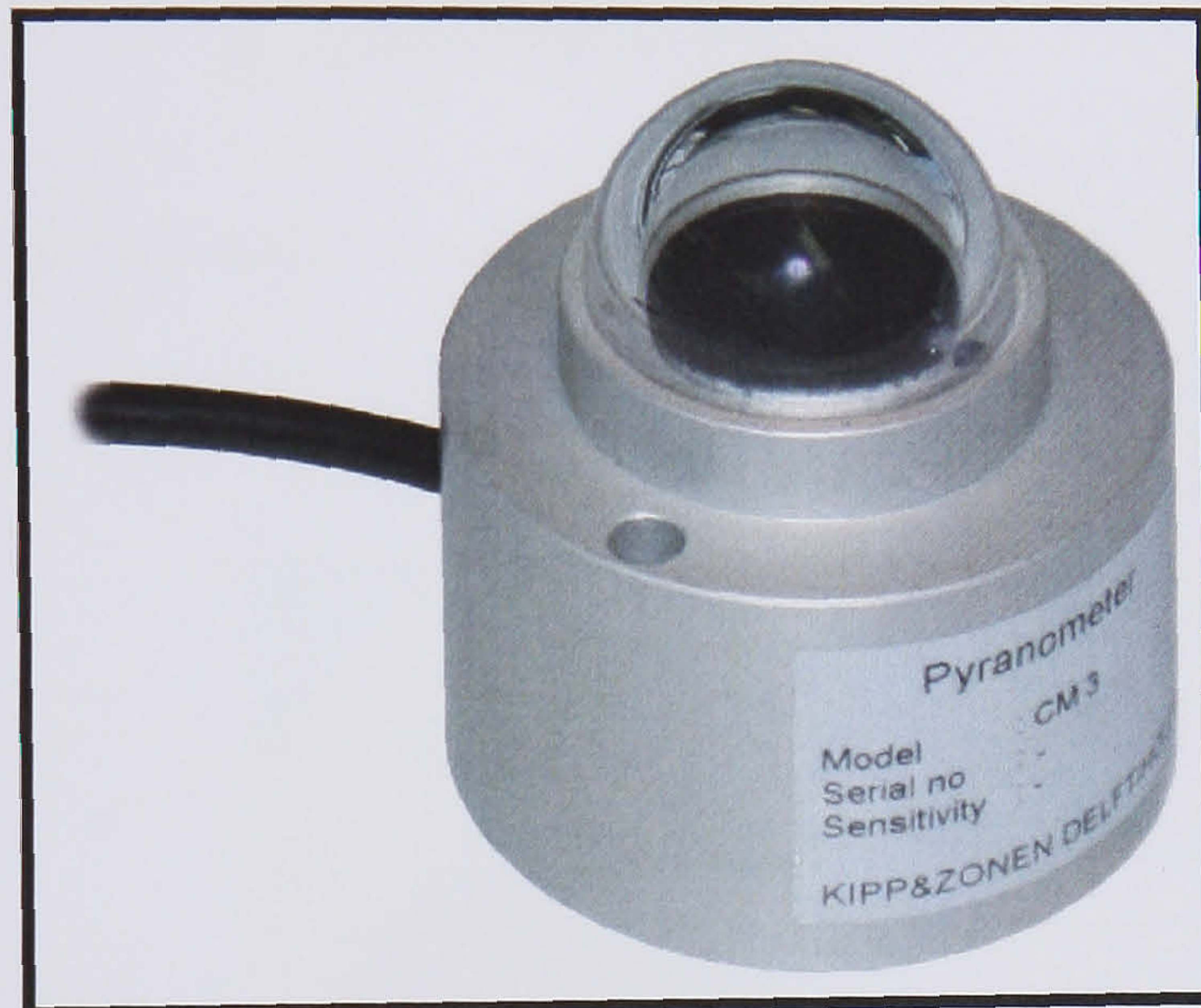
Figure 3.10 CM3 Pyranometer ( www.campbellsci.com )
