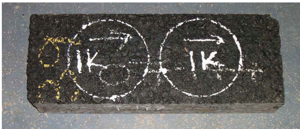
Figure 5.11 – Prismatic specimen used in FWT
