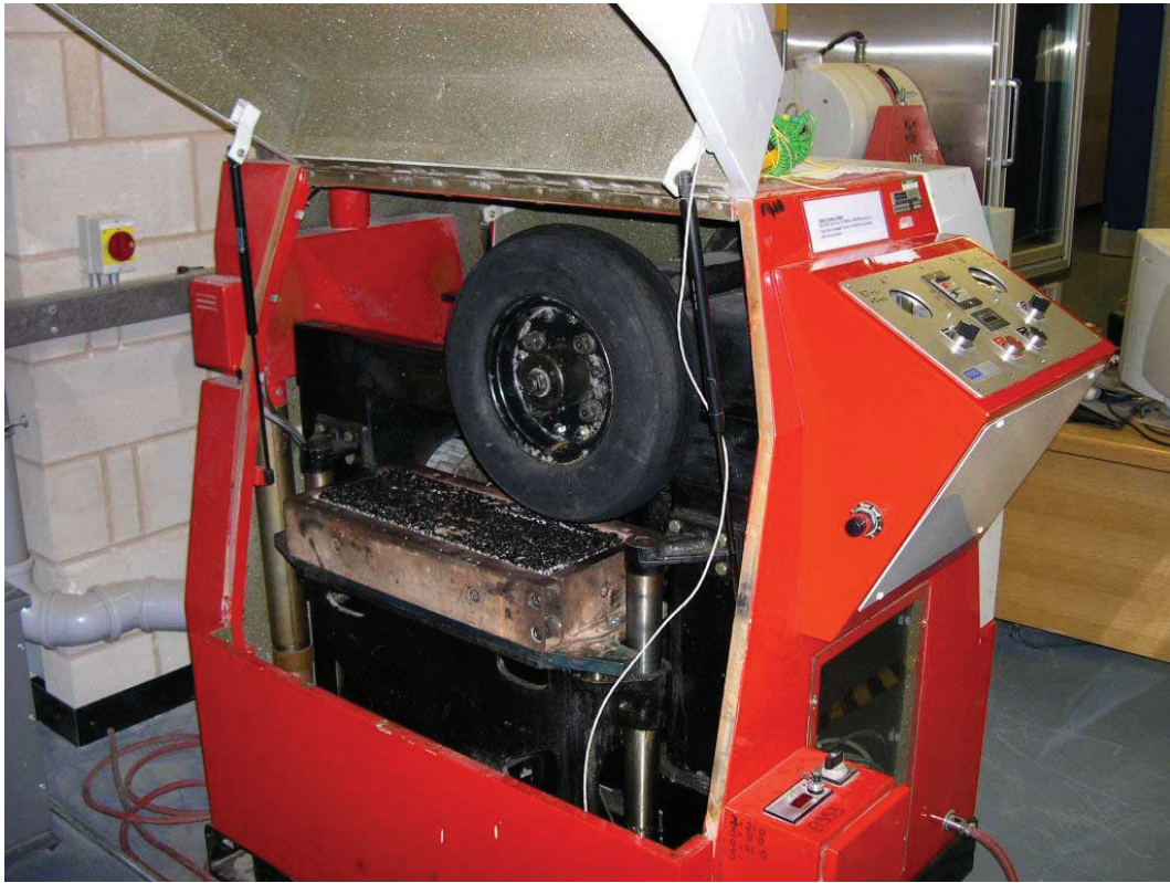
Figure 5.12 – Trafficking setup for FWT
