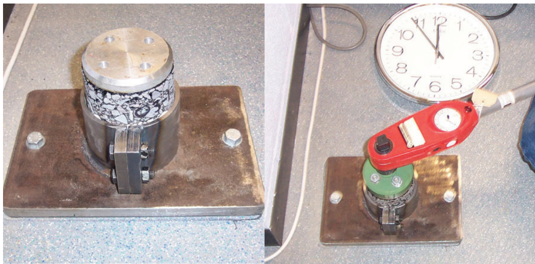
Figure 4.7 – Laboratory manual torque bond test equipment used by Choi et al. [2005]
