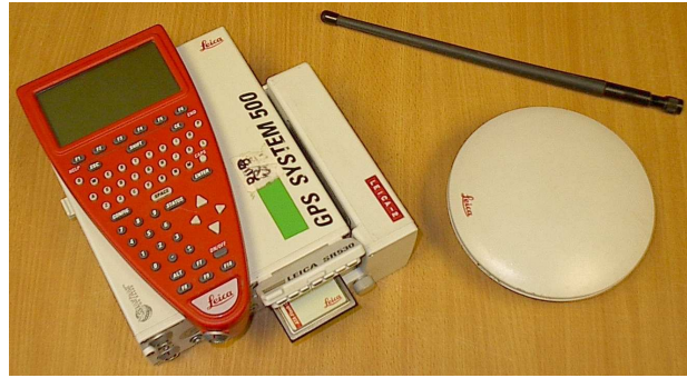
Figure 4.3 GPS Receiver, Antennas, Flash Card, and Radio
