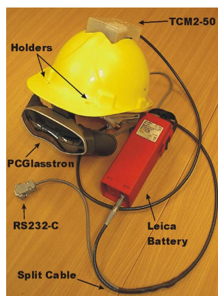
Figure 4.8 Helmet, PCGlasstron, Leica Battery, See-Through HMD and Cable
